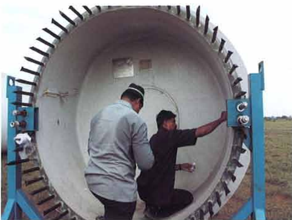
Blade Instrumentation work for Inox 2000 kW Wind Turbine
