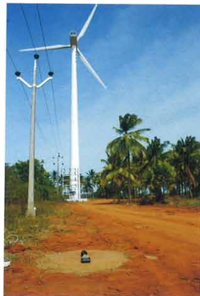
Acoustic Measurements in Progress
