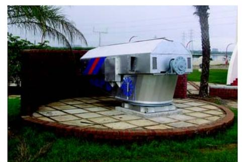
*55 kW Wind turbine nacelle in C-WET*
