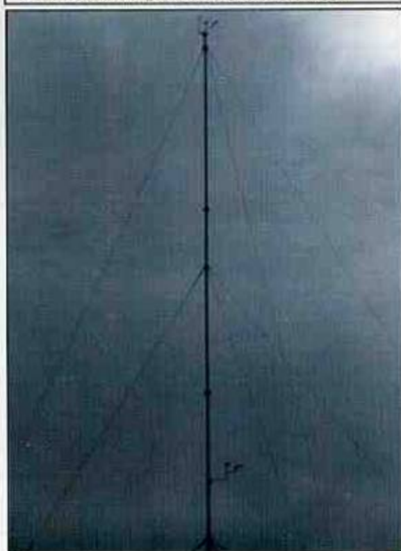
Close-up view of the 10m and 25m level sensors installed at Mylapatti, Tamil Nadu
