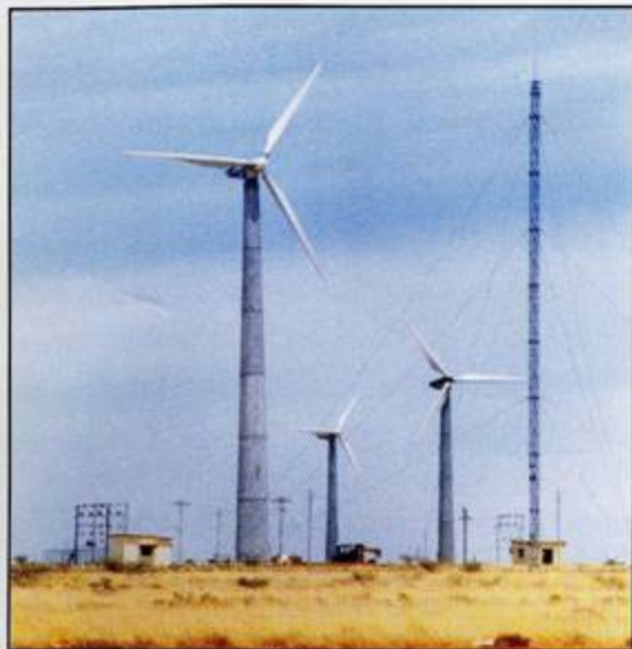
225kW Wind Turbine under Test at Test Bed-B
