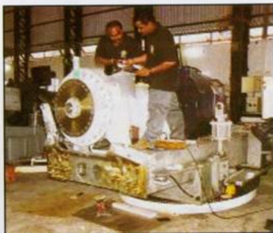
Strain gaging of Vestas Pavan Shakti 600 kW wind turbine at the Vestas RRB factory
