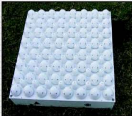
Fig.2: SODAR instrument with 64 transducers
