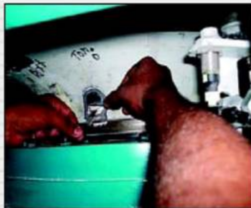
Fig.17: Strain gaging in main shaft of Suzlon 600 kW turbine for its PTT programme
