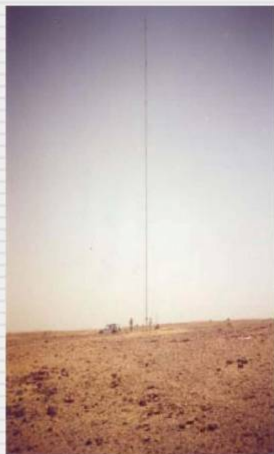
Fig.13: 50m Tall Wind Monitoring Station at Khodal
