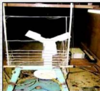
Fig.1: Velocity profile measurements in Wind Tunnel across the wind turbine nacelle at SERC
