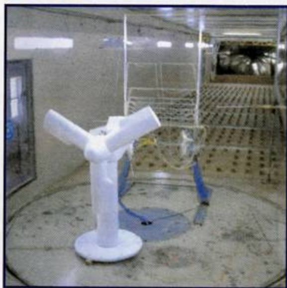
Measurement frame near nacelle
