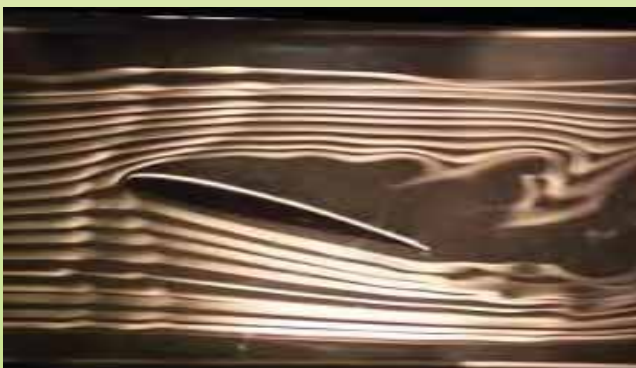
Proposed Aerofoil study in a Wind Tunnel
