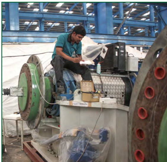
Elecon 600 kW - Shaft strain gage strain measurement
