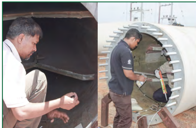
Elecon 600 kW Blade Instrumentation - Strain gage mounting
