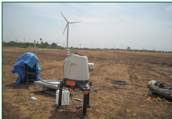
Wake is being measured behind 2 MW wind turbine by using LIDAR
