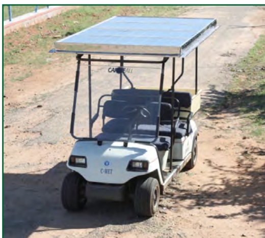
Battery operated vehicle at WTRS designed to operate by Solar PV Panels
