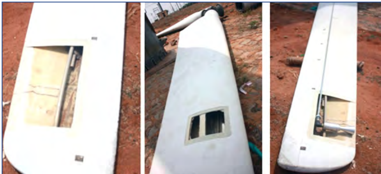
Installation of Micro Thruster at the tip of the blades
