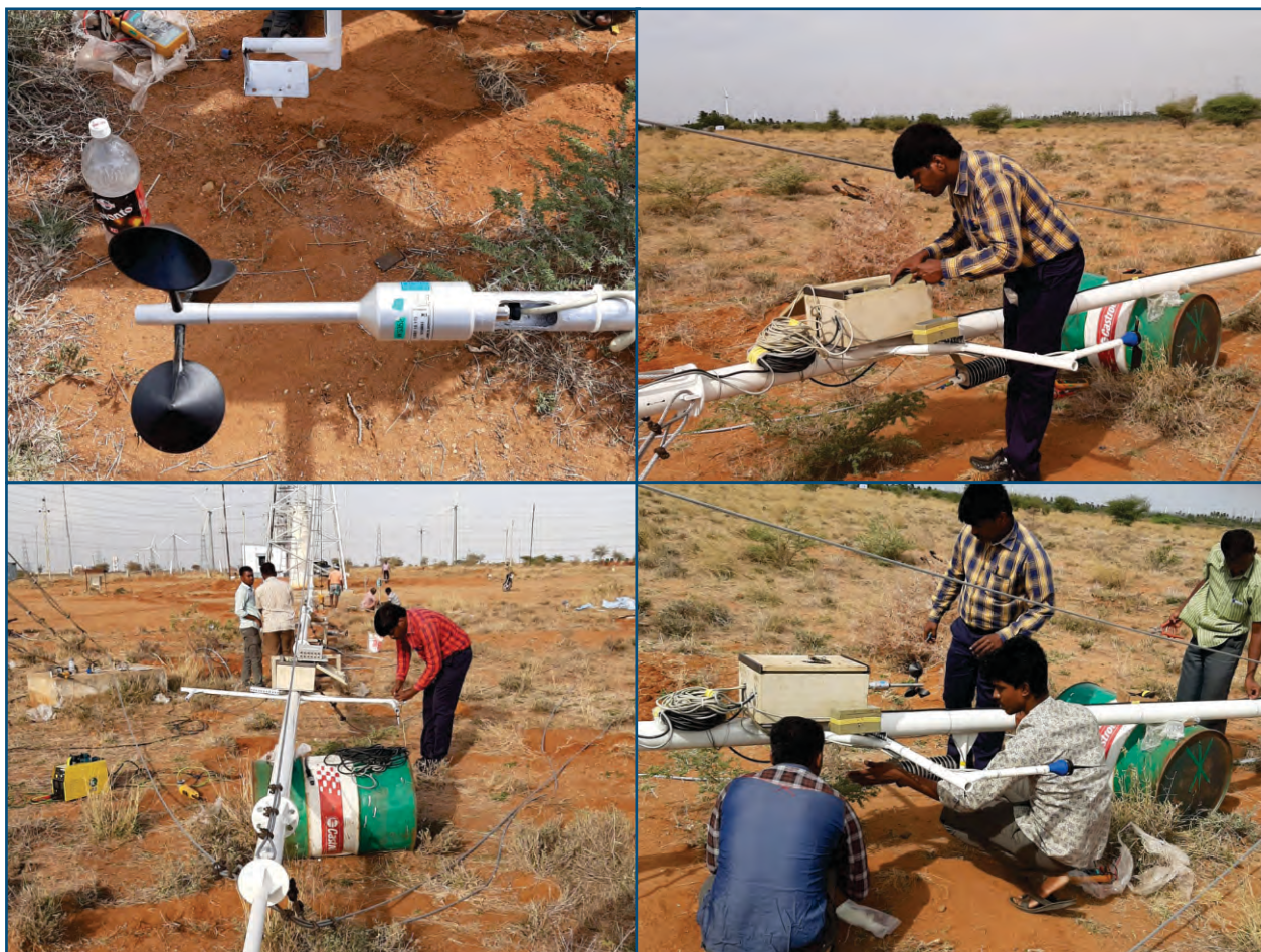
Type Testing of model Vaata Smart, Vertical Axis Wind Turbine in progress at WTRS, Kayathar
