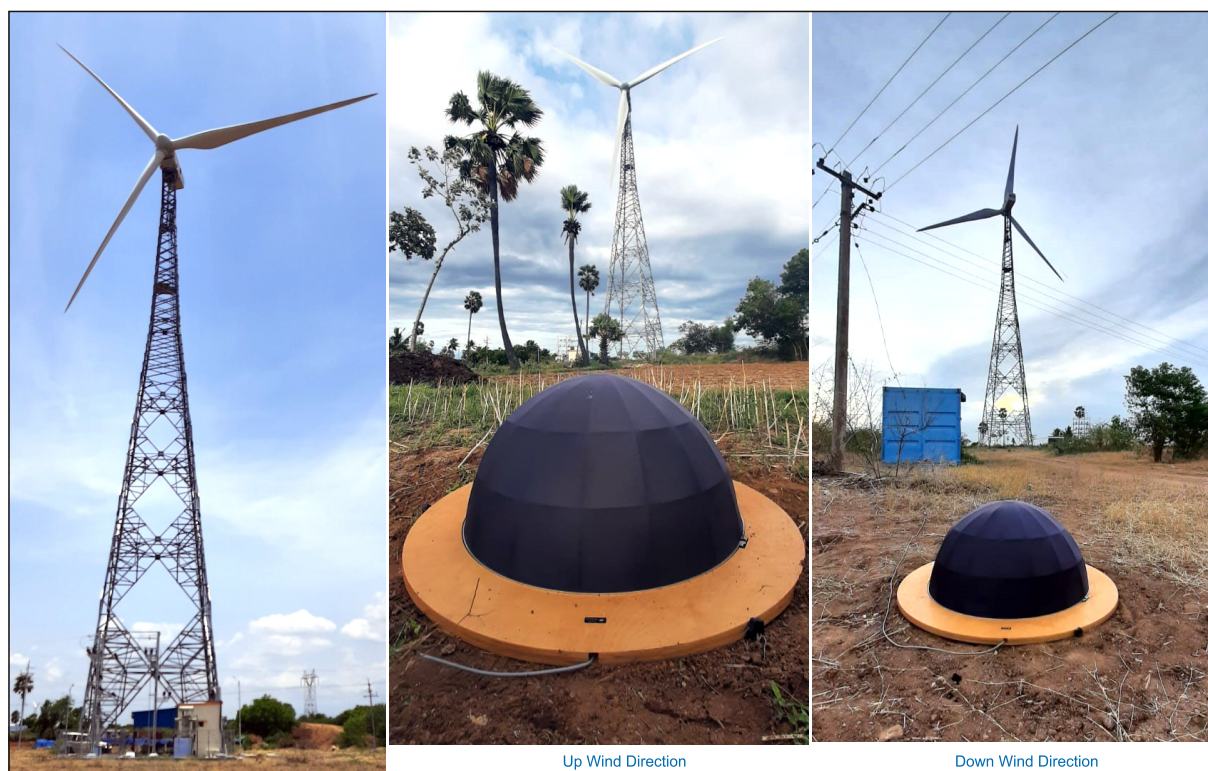
Acoustic Noise Measurement (ANM) for Model –P57,750 kW, a wind turbine from M/s. Para Enterprises Private Limited at Manur Taluk, Tirunelveli District, Tamil Nadu
