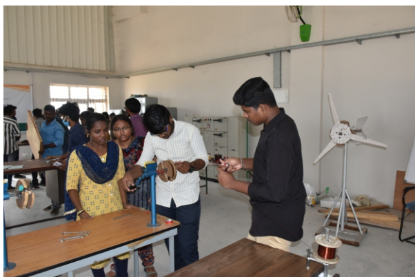
Stator coil winding by the students
