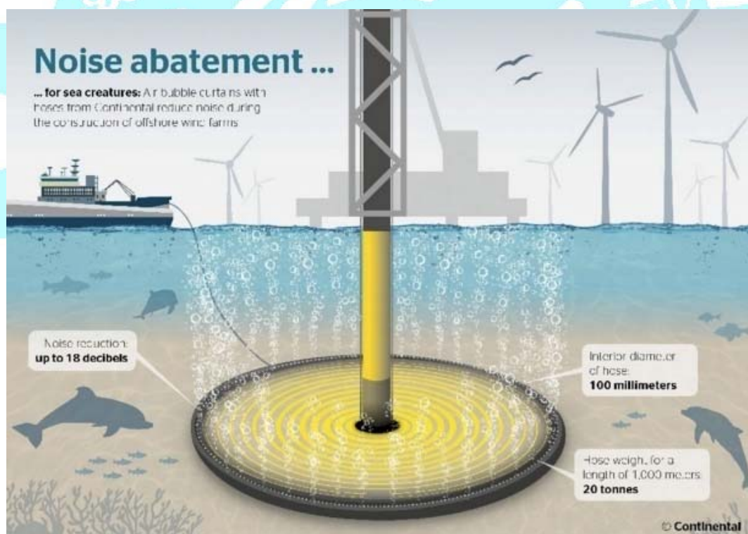
Fig 7.1: Depicting noise abatement via use of bubble curtain.
