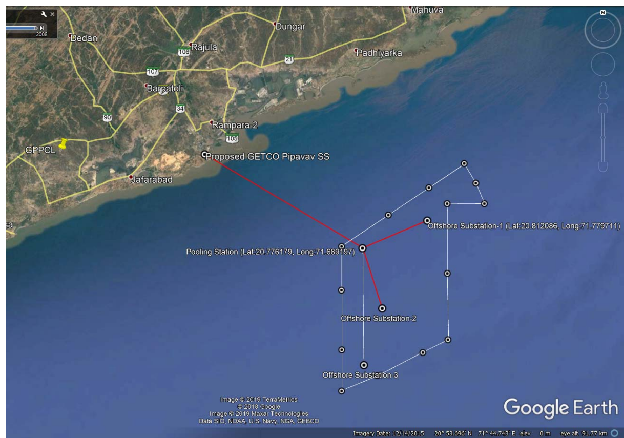
Figure 2.4 HVAC transmissions from the offshore wind farm
