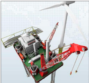
Figure 58 - A small DP2 WTIV Seajack's Kraken
