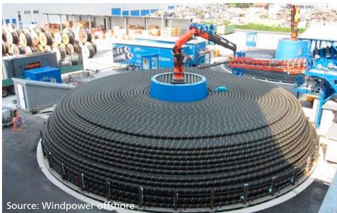
Figure 50 - Offshore wind cables stored onshore
