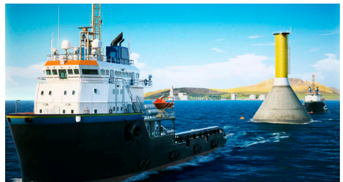
Figure 78 - Towing a floating Gravitass GBS foundation
