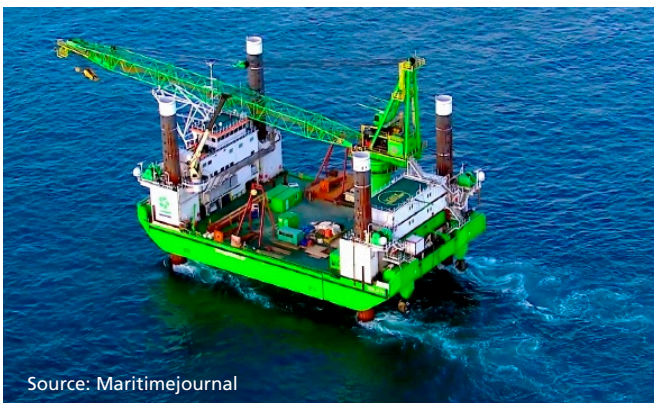
Figure 100 - Jack-up 'Goliath' in strong current in the Raz Blanchard
