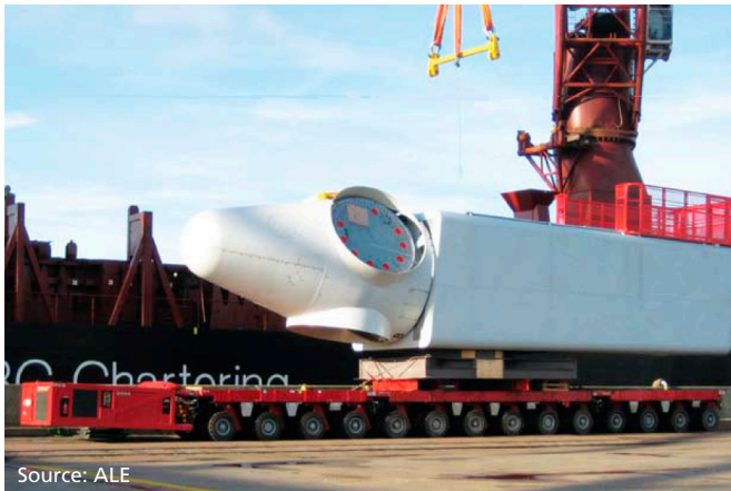
Figure 37 - Siemens SWT 3.6 on SPMT trailer
