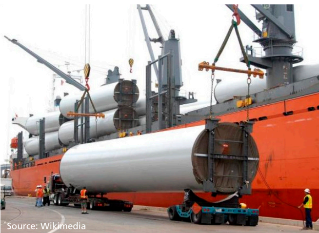
Figure 36 - Tower section vessel cranae load-out
