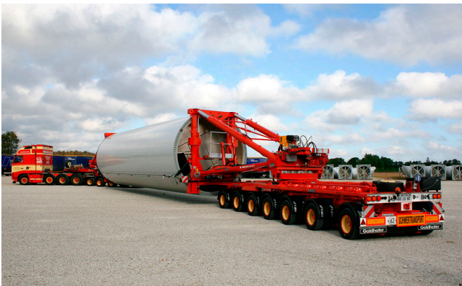
Figure 32 - Goldhofer RA3 tower haulage unit
