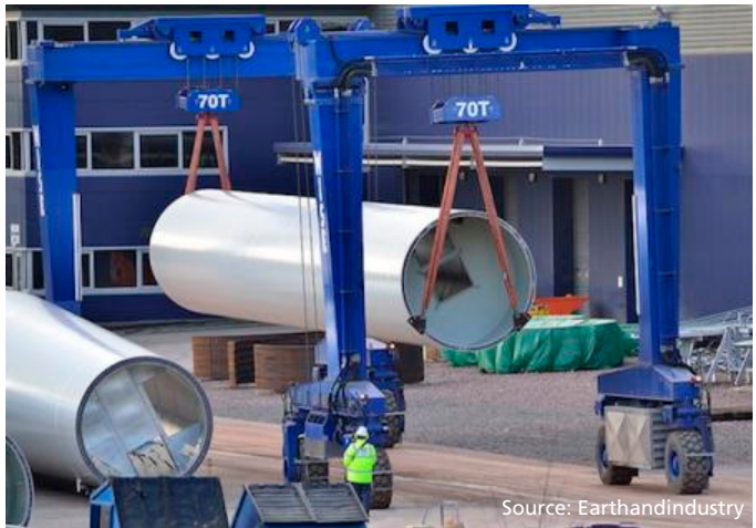
Figure 33 - Tower section transportation
