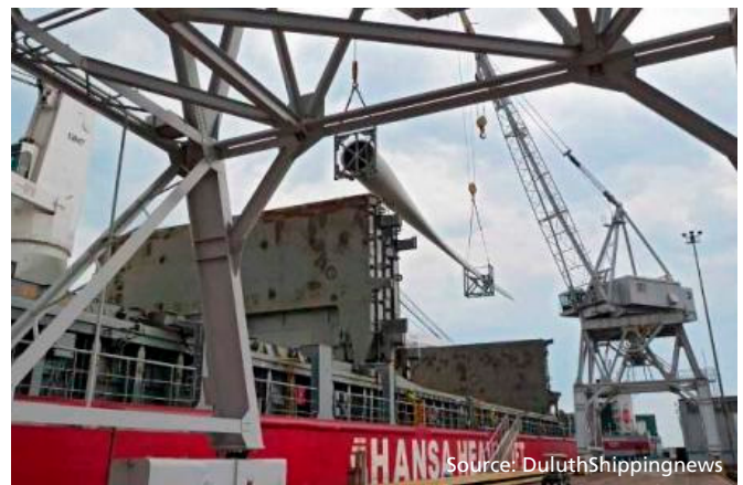
Figure 29 - Port craneage blade load out
