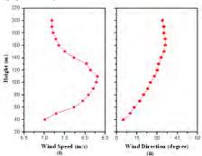
Figure 1. Height profile of (i) Wind speed and (ii) direction measured from SODAR
