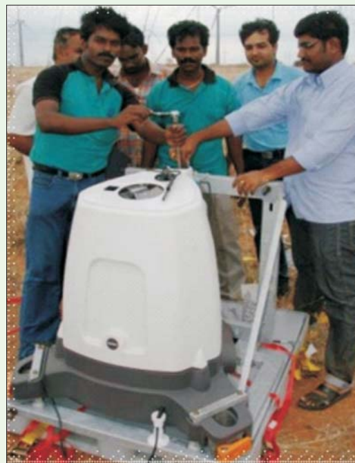
Wind profile measurement by using LIDAR at WTTS/WTRS, Kayathar
