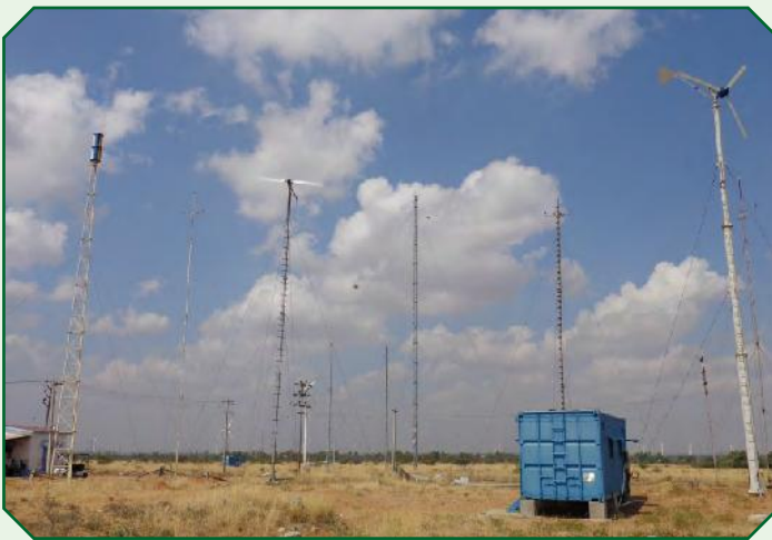
Small Wind Turbine Testing at WTRS
