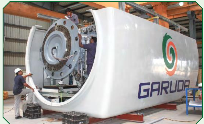
Factory Instrumentation of Garuda 1700.84 kW Wind Trubine
