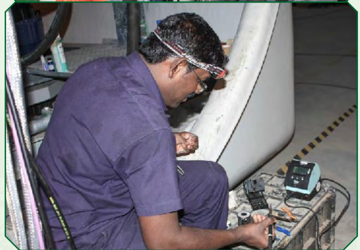
Factory Instrumentation of Garuda - Shaft Strain Gauge
