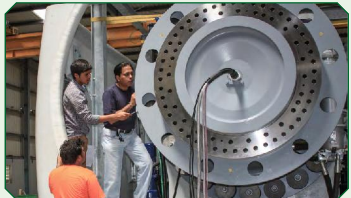
Factory Instrumentation of Garuda 1700.84 kW Wind Trubine
