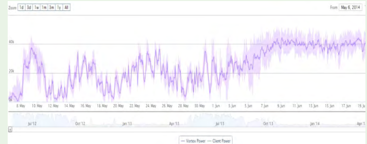
Fig 6. Forecasting results for the 50 MW wind farm
