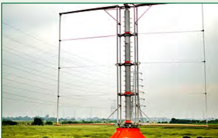
Vertical Axis Small Wind Turbine installed at WTRS for testing
