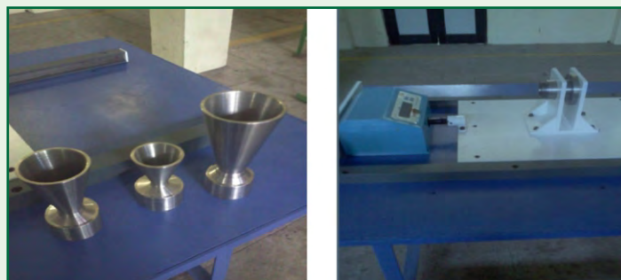
Three different size Thruster fabricated - Thruster test rig setup
