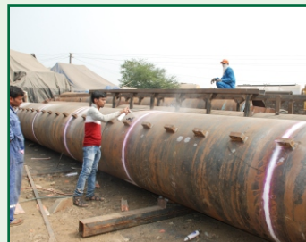
Figure 7 Dye Penetration test
