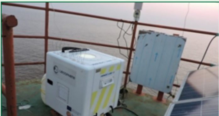
Figure 2 LIDAR at Offshore Platform
