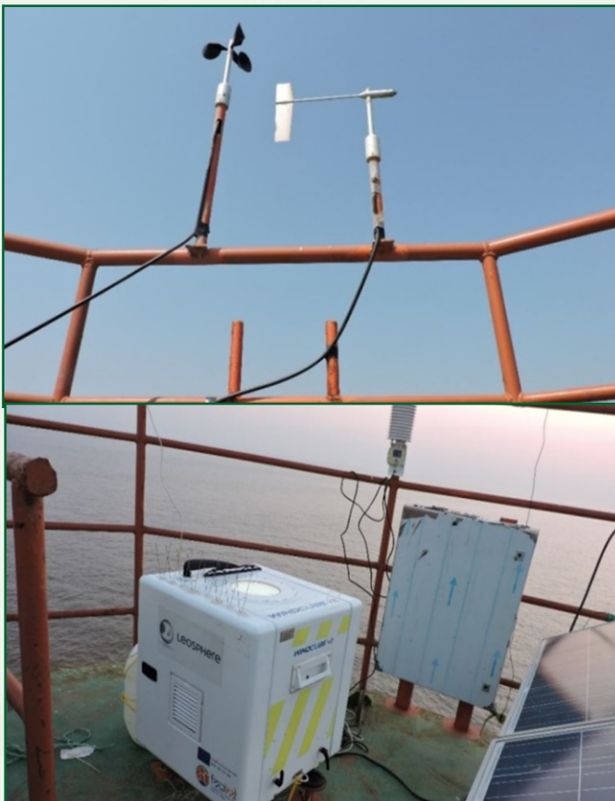
Automated weather station along with Lidar equipment on the platform
