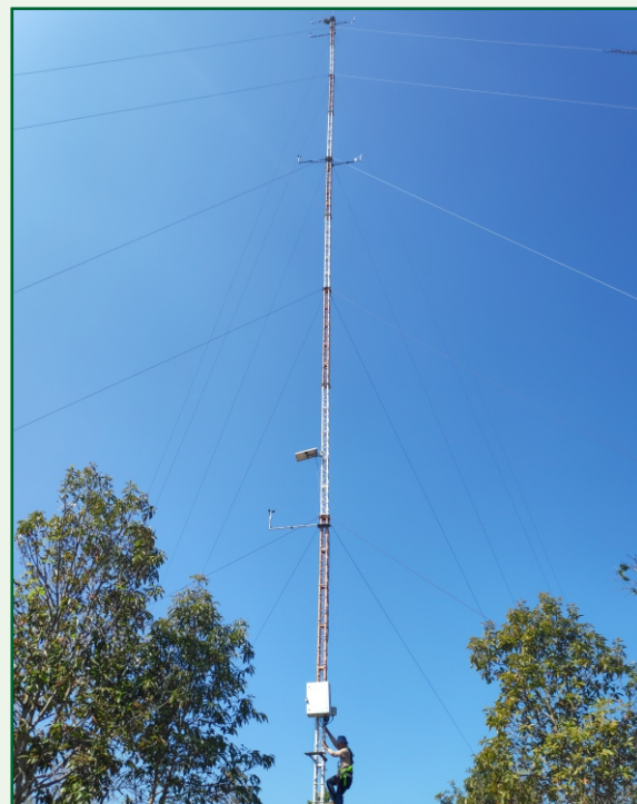
50 m Wind monitoring station installed at Tripura
