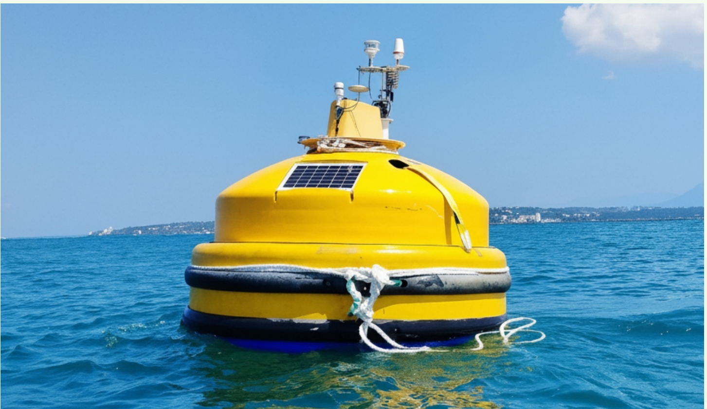
Short term Deployed NIOT Buoy with NIWE LIDAR
