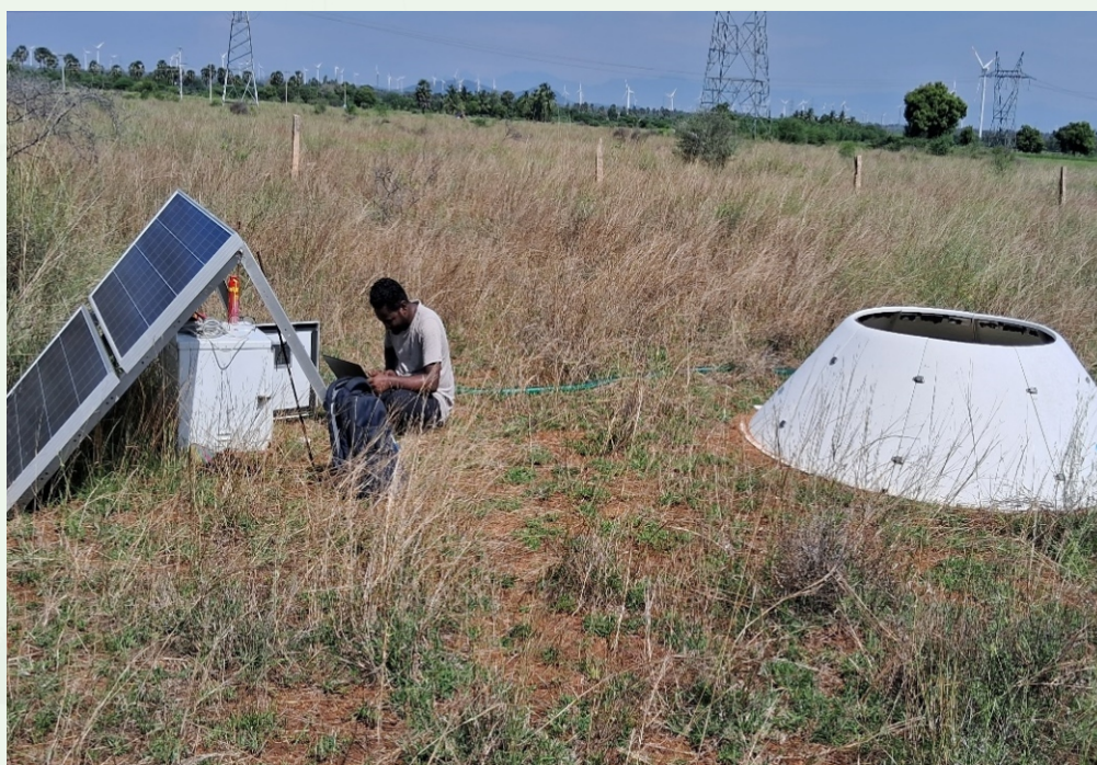
SoDAR Rectification work at Kayathar in progress
