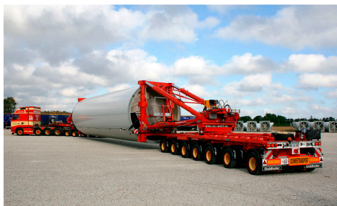
Figure 32 - Goldhofer RA3 tower haulage unit
