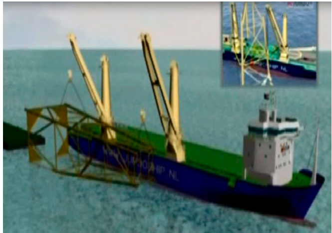
Figure 63 - Heavy lift cargo vessel - jacket installation
