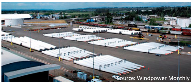
Figure 27 - Wind turbine blade storage (single frame)
