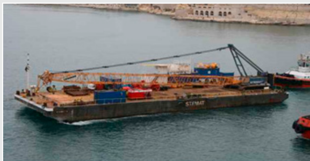
Towed 'dumb' barge with crane
