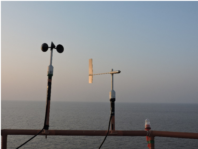
Weather Station at LiDAR Platform (at 20m amsl)
