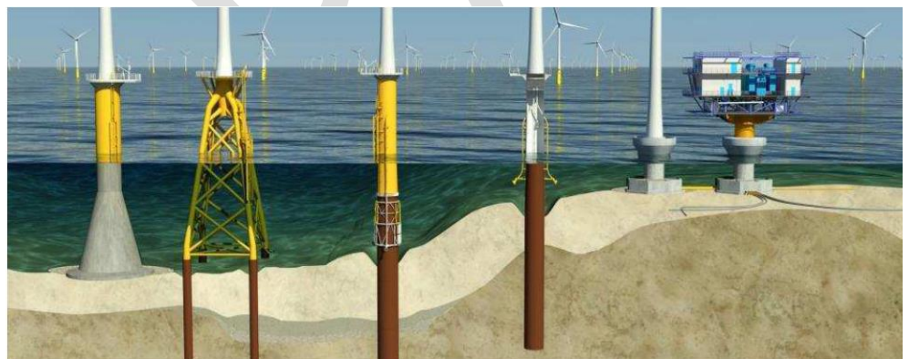
Figure 4-1 Illustration of OWF foundations designed by COWI. From left: Thornton Bank concrete gravity based, Wikingjer jacket (preliminary stage), two times London Array monopile, Nysted WTG and Rødsand 2 offshore substation concrete gravity based
