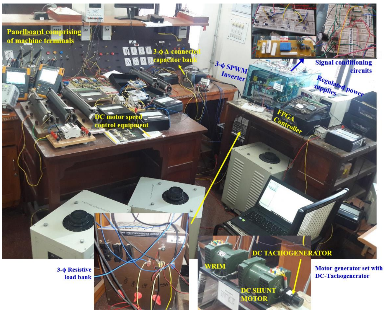
(h) Electrical connections along with the measuring equipments
