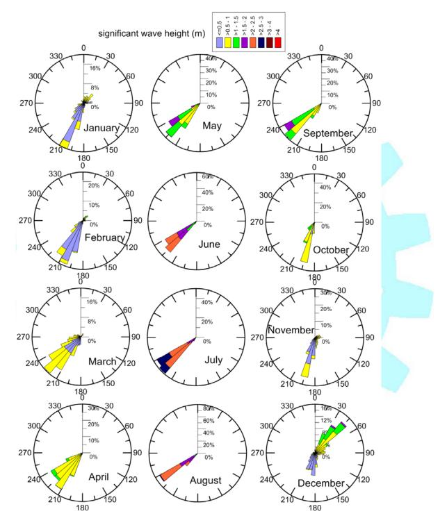
Figure 3.5.1.Wave rose diagram near the study area based on wave hindcast data for the year 2018
