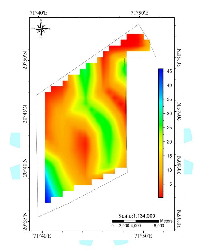
Figure 3.3.4 Distribution of clay content in the surface sediment
