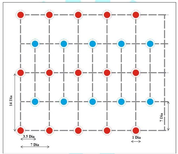
Figure 3.9.12: Staggered grid 7 x 14 diameter spacing
