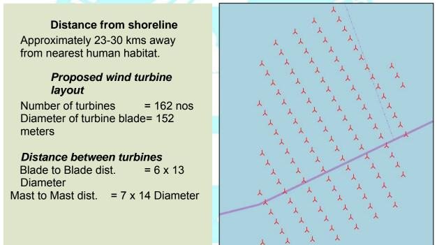
Figure 3.9.4: Proposed Wind Turbine Layout (Option – 2)
