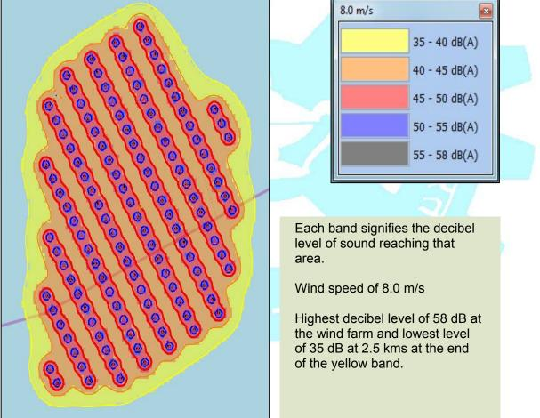
Figure 3.8.11: Simulation results for Option 2 at wind speed 8m/s
