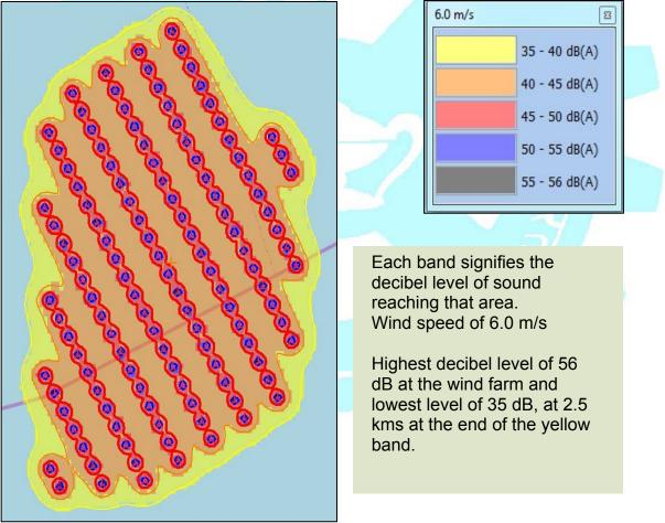
Figure 3.8.10: Simulation results for Option 2 at wind speed 6m/s
