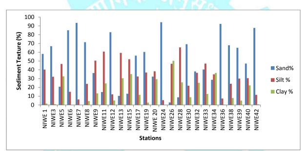
Figure 3.10.6: Spatial variations of sediment texture in the top layer of coastal sediment at the sampling stations in the survey area off Pipavav
