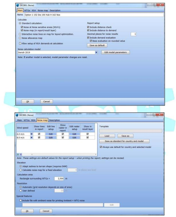
**Simulation Inputs for Option 2 (162 turbines)** Low-frequency noise analysis using the DECIBEL feature in WindPRO 3.3. Input parameters for simulation in WindPRO 3.3 are shown below.
