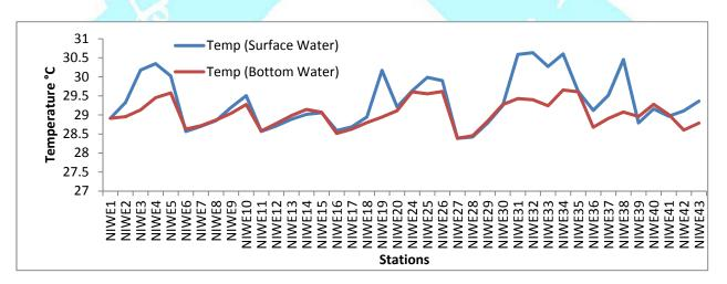
Figure 3.10.1: Spatial variations of temperature in surface and near-bottom waters at the sampling stations off Pipavav.
