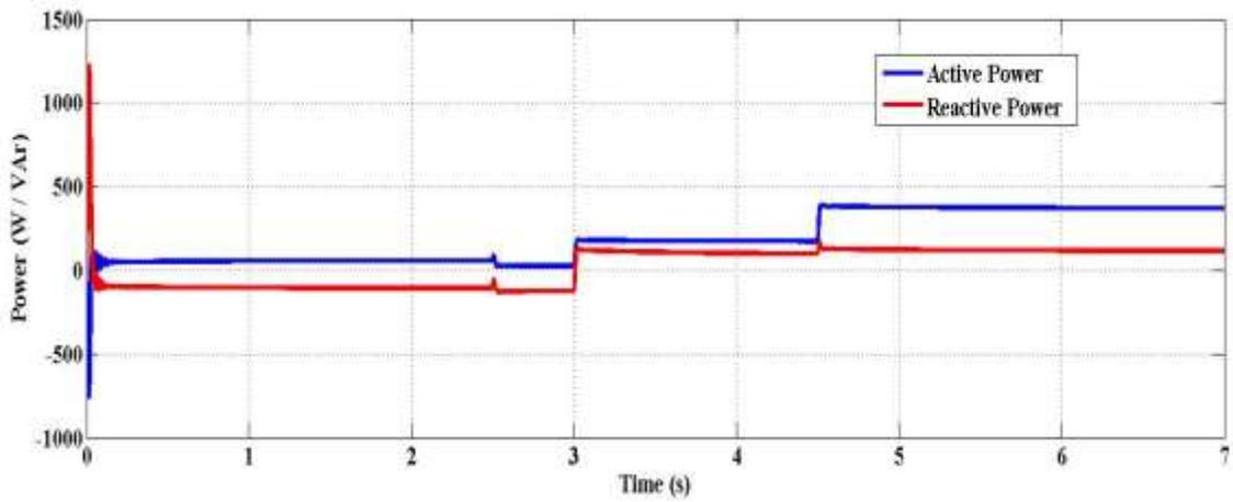
Figure 4.12 Real and reactive powers of the rotor versus time
