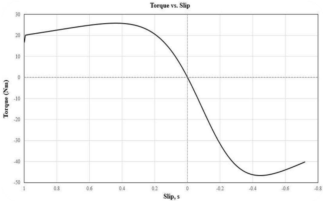
Figure 10.2(b) Torque-slip characteristics of the induction generator used
