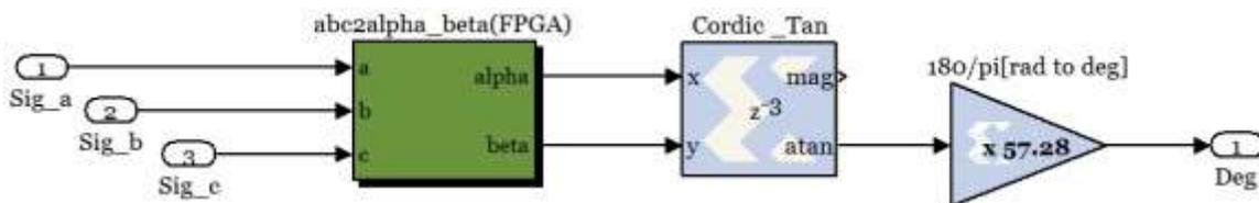
Figure 5.16 Computation of angle of space vectors
