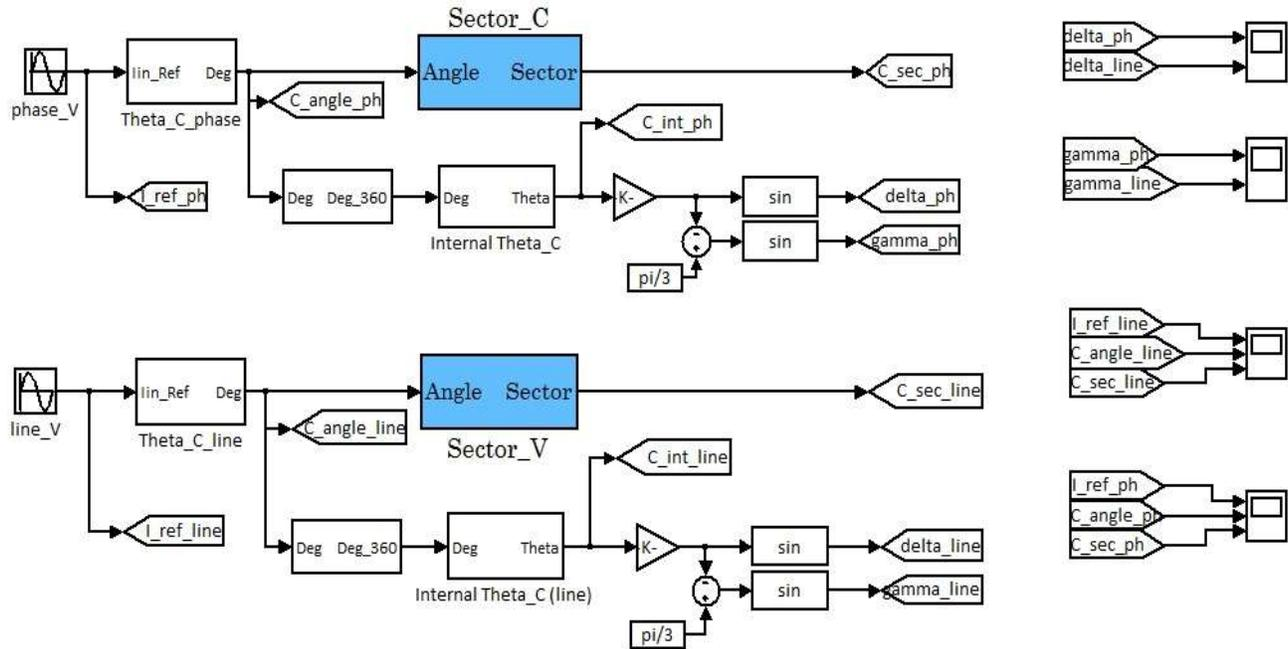
Figure 5.10 Sector computation of the CSV using the VSV
