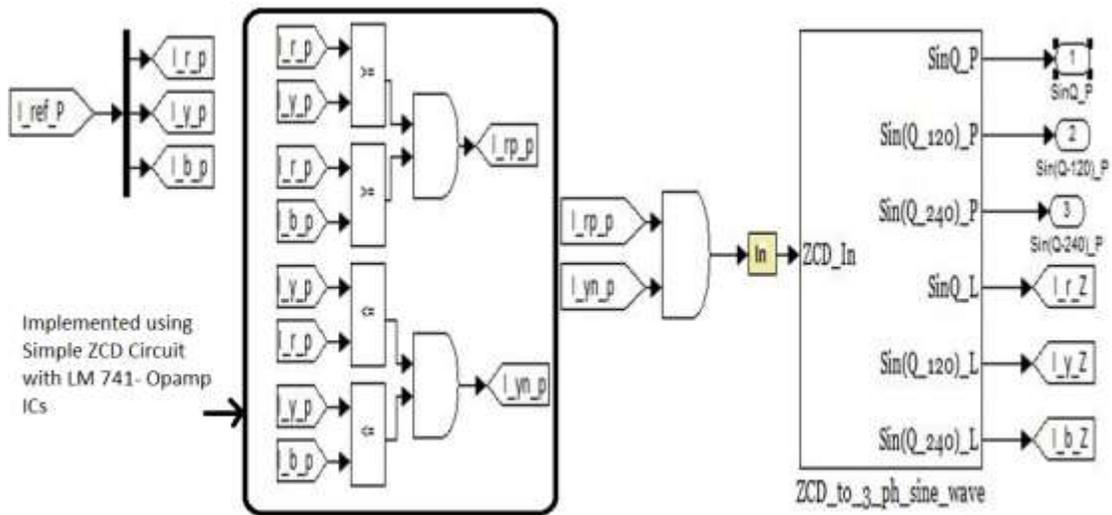
Figure 8.1 Matlab/Xilinx model to reconstruct the reference signals for the currents.t
