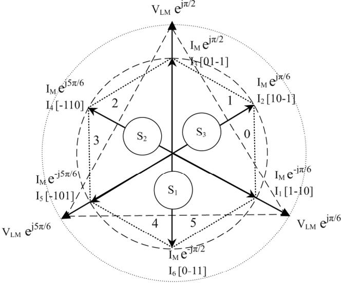
Figure 4. FDCV space vector with rectifier current space vector.
