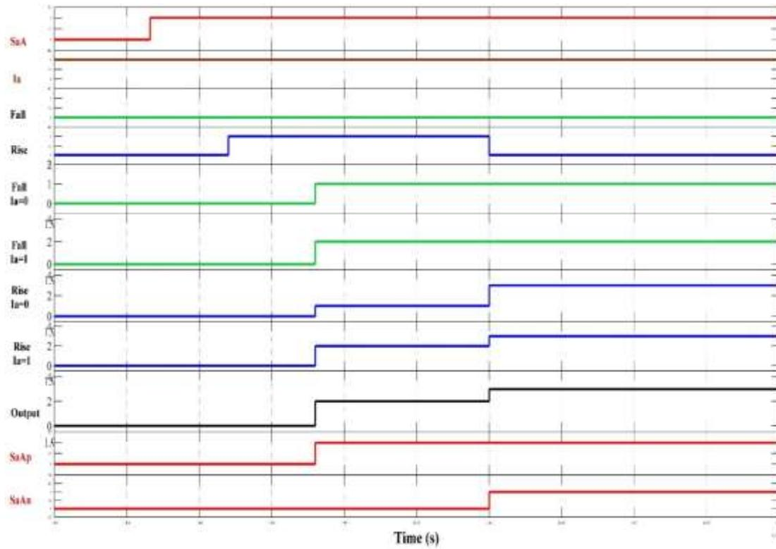
Figure 5.49 Pulses of switch SaA when a falling edge occurs with positive current
