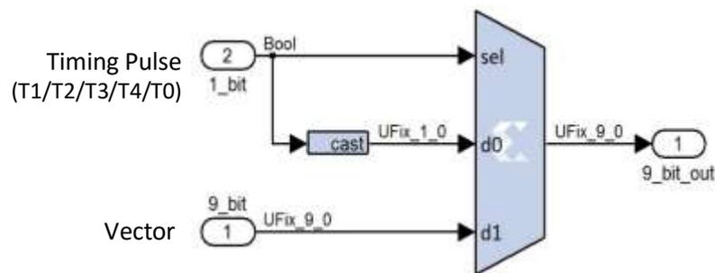
Figure 5.6 Replacing multipliers with multiplexers
