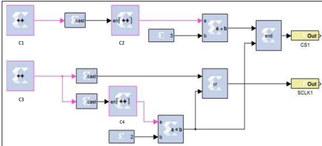
Figure 7.5 Xilinx model to generate Chip Select & SCLK
