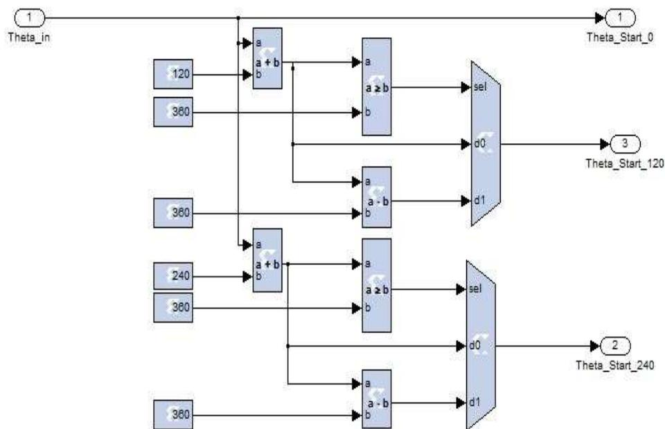
Figure 8.22 Matlab/Xilinx model for generating theta for the three-phase system
