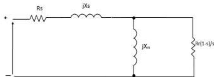
Figure 3.4 (c) Equivalent circuit after combining  $R_c$  and  $R_r/s$
