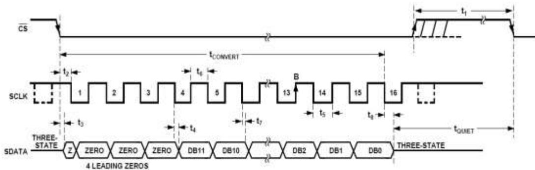
Figure 7.3 AD7476 serial interface timing diagram
