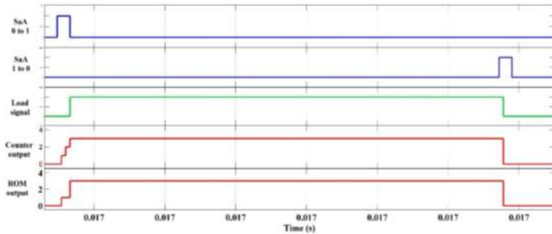
Figure 5.46 Counter and ROM output for the negative current when rising edge is detected
