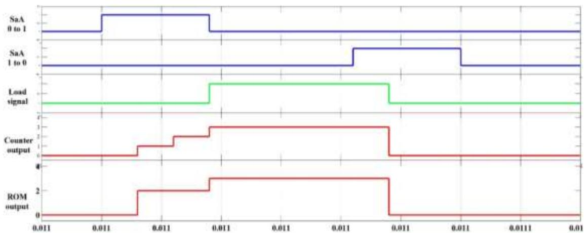
Figure 5.47 Counter and ROM output for positive current when rising edge is detected
