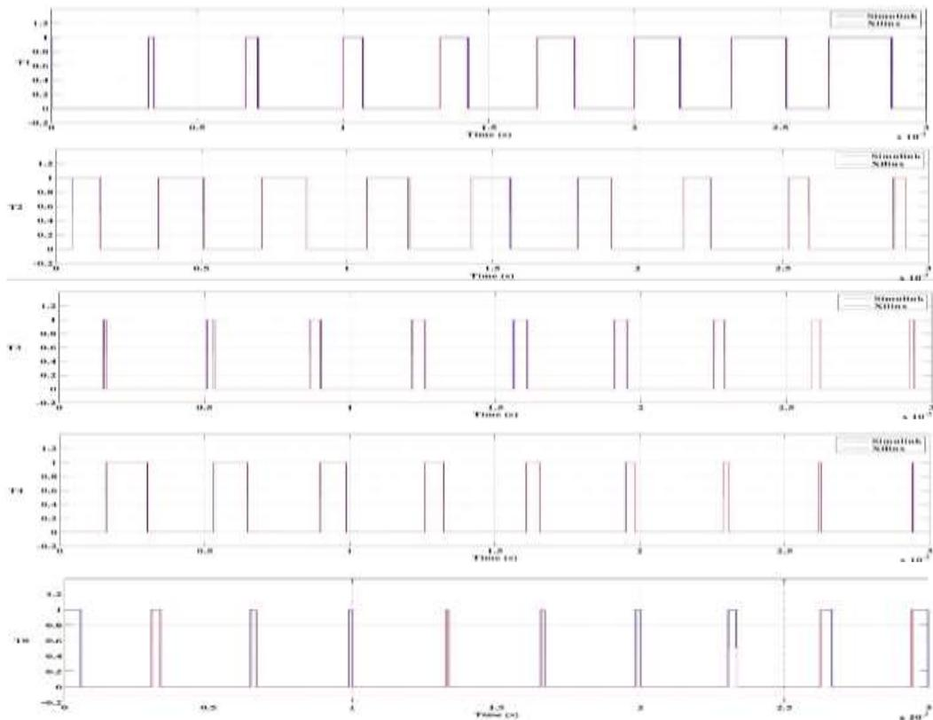
Figure 5.29 Timing pulses obtained from Xilinx and Simulink
