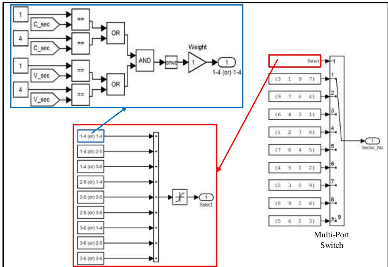
Figure 2.26 Vectors Identification (Implementation of Table 2.3)
