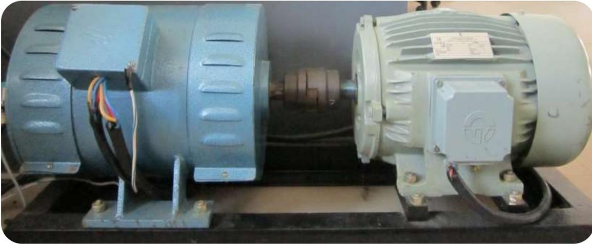
Figure 10.1 Induction motor - induction generator setup
