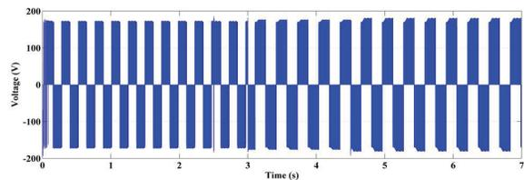
Fig. 8. Line-to-line voltage injected by the converter into the rotor of DFIG
