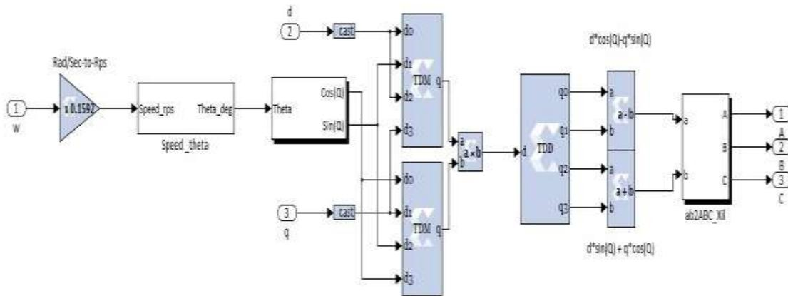
Figure 6.16 Matlab/Xilinx model to generate the reference voltages for the rotor side converter
