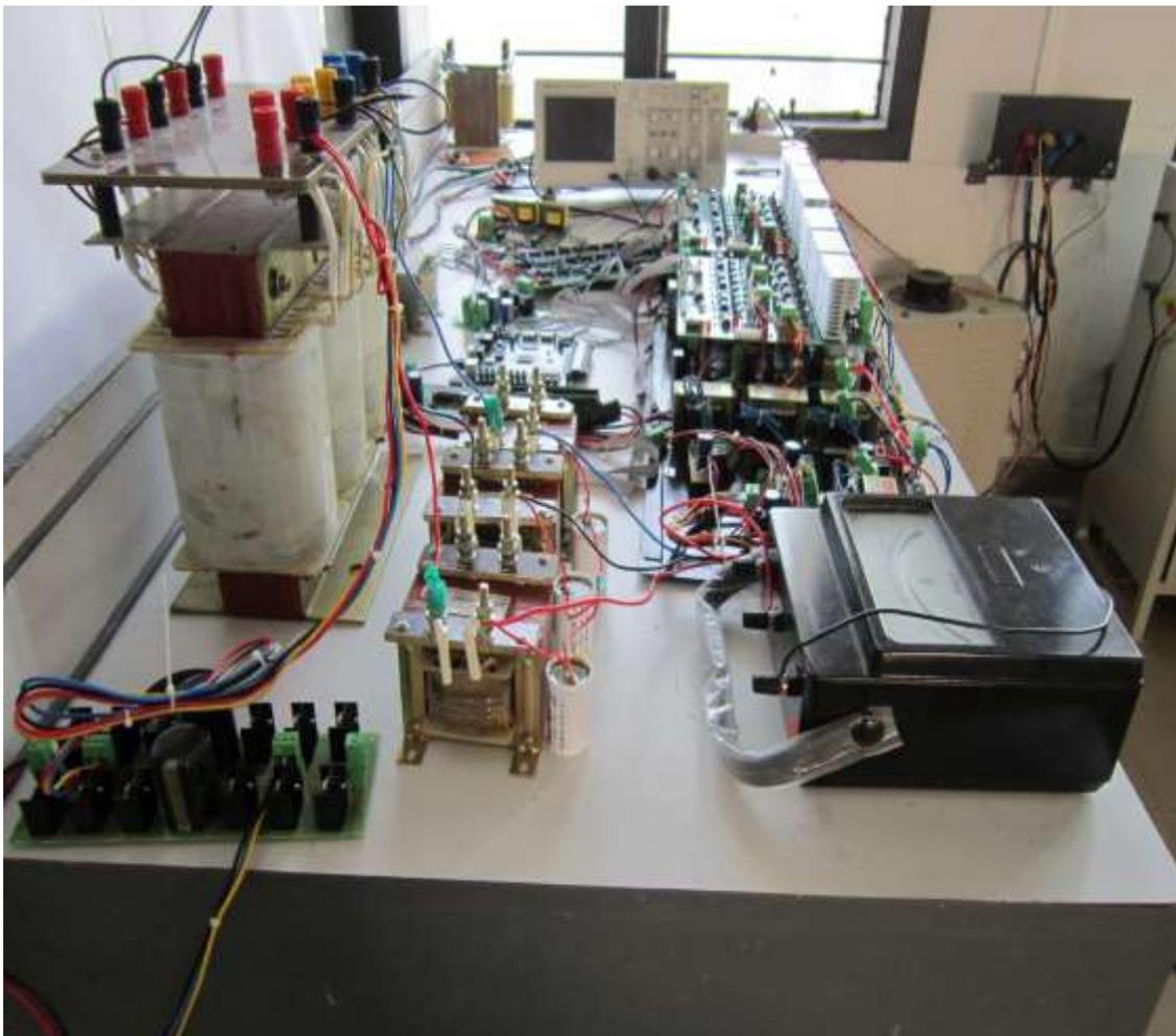
Figure 10.28 Matrix converter prototype setup
