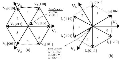
Figs. 2. (a) Inverter Voltage Hexagon, and (b) Rectifier Current Hexagon
