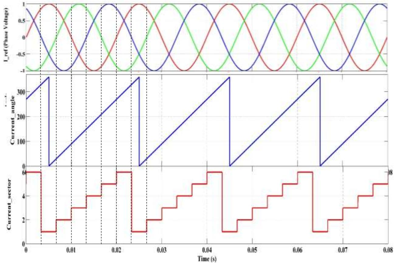
Figure 2.19 Current sector obtained from  $\beta_i$
