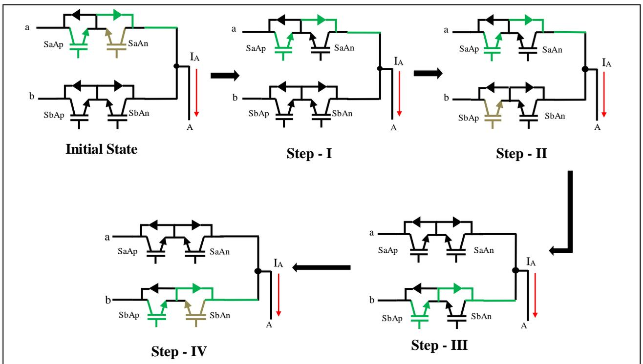
Figure 2.33 Sequence of commutation of devices when  $I_A$  is positive
