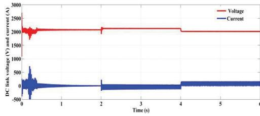
Fig. 10 DC link voltage and current
