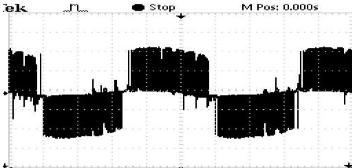
Figure 10.33 (a) Output Line Voltage of matrix converter applied to the rotor of the DFIG
