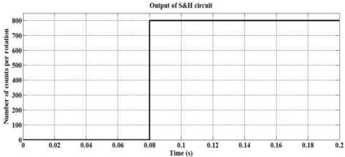
Figure 9.9 No. of counts obtained from the S&H circuit
