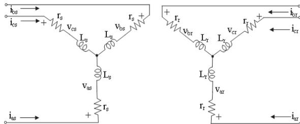
Fig. 2 Stator and rotor circuits of the induction machine
