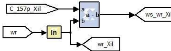
Figure 6.11 Calculation of the slip speed in Matlab/Xilinx using the stator and rotor speeds
