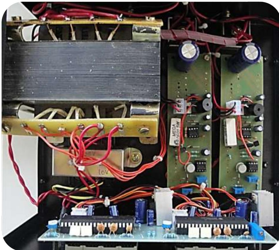
Figure 10.20 Regulated power supply unit
