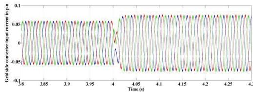
Fig. 12 Input current of Grid side converter
