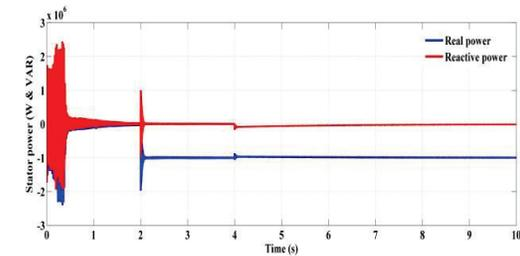
Fig. 9 Stator real and reactive power delivered to the grid
