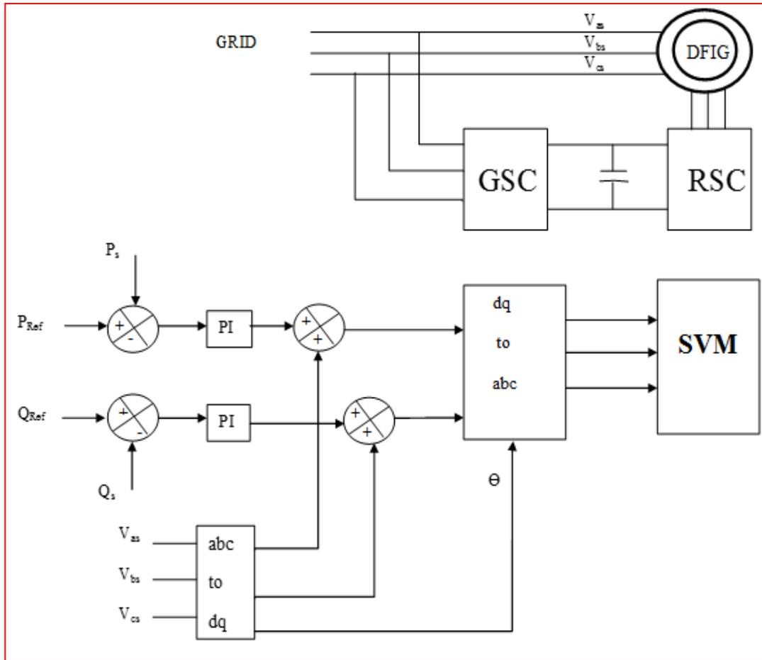
Figure 1.4 Rotor side control scheme for the conventional back-to-back converter
