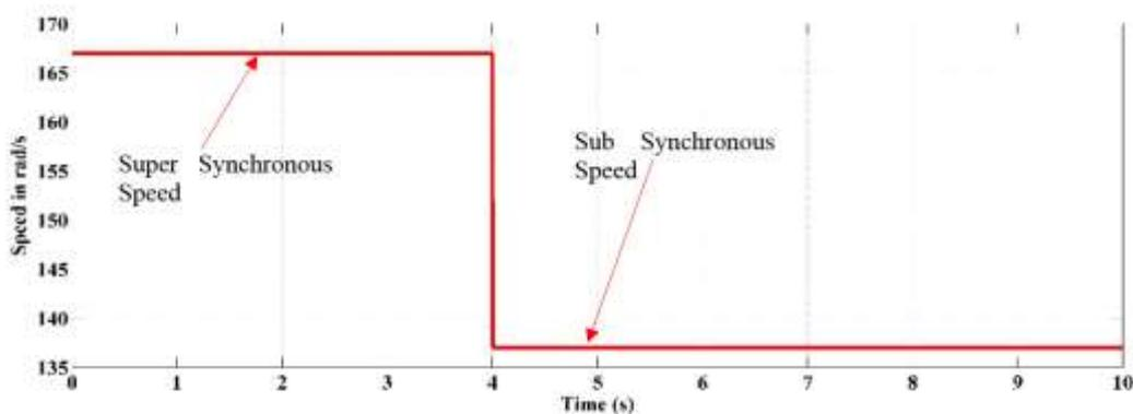
Figure 3.24 Input speed of the DFIM machine
