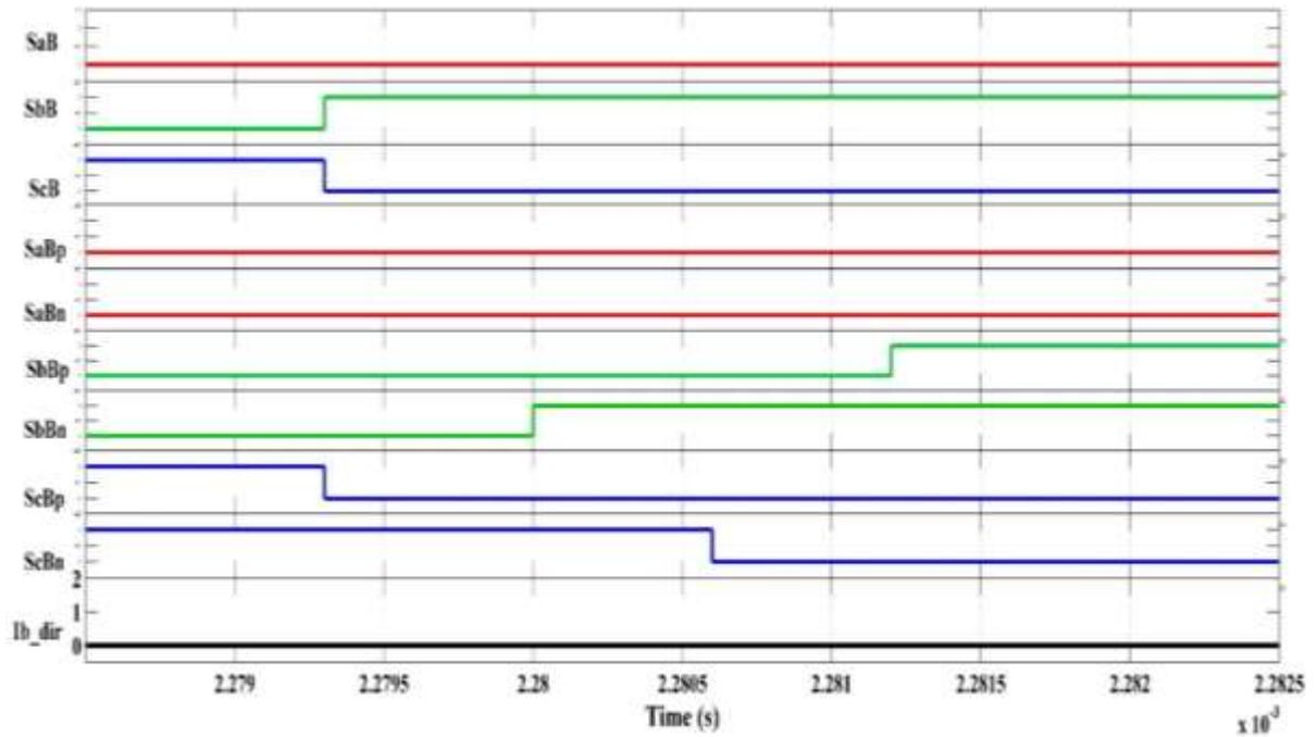
Figure 5.52 Pulses to switches connected to load phase 'A' when current is negative
