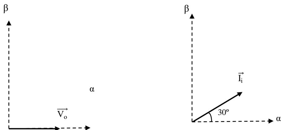
Figure 2.3 Voltage and current Space Vectors for the switch state [acc]
