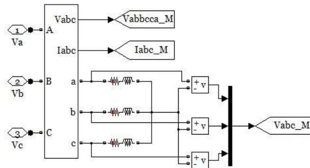
Figure 2.11 Three-phase RL load
