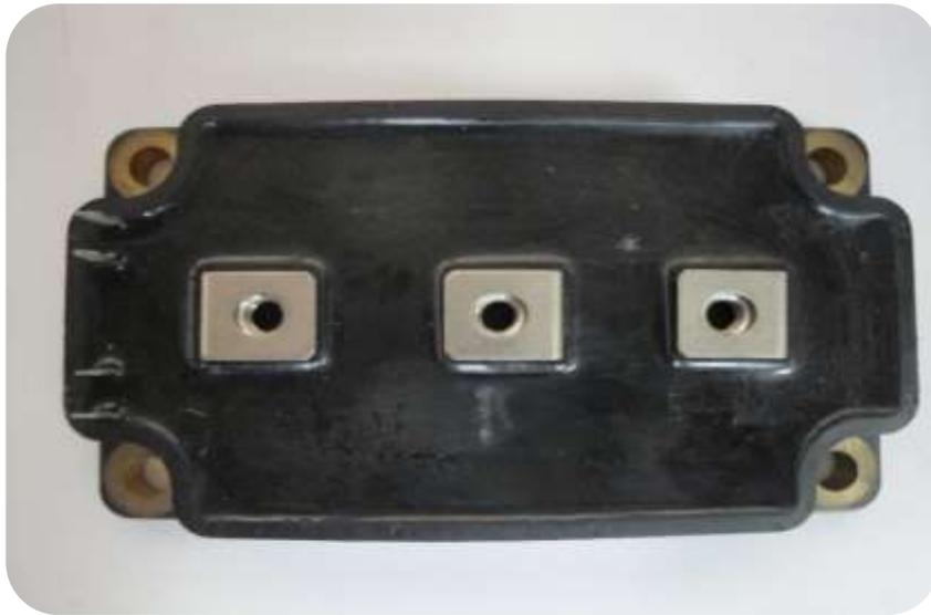
Figure 10.4(a) APTGT150DU120G bidirectional power switch
