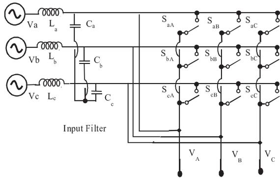
Fig. 3. Conventional matrix converter
