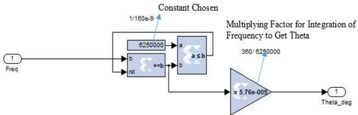
Figure 8.19 Matlab/Xilinx model to obtain theta from the frequency
