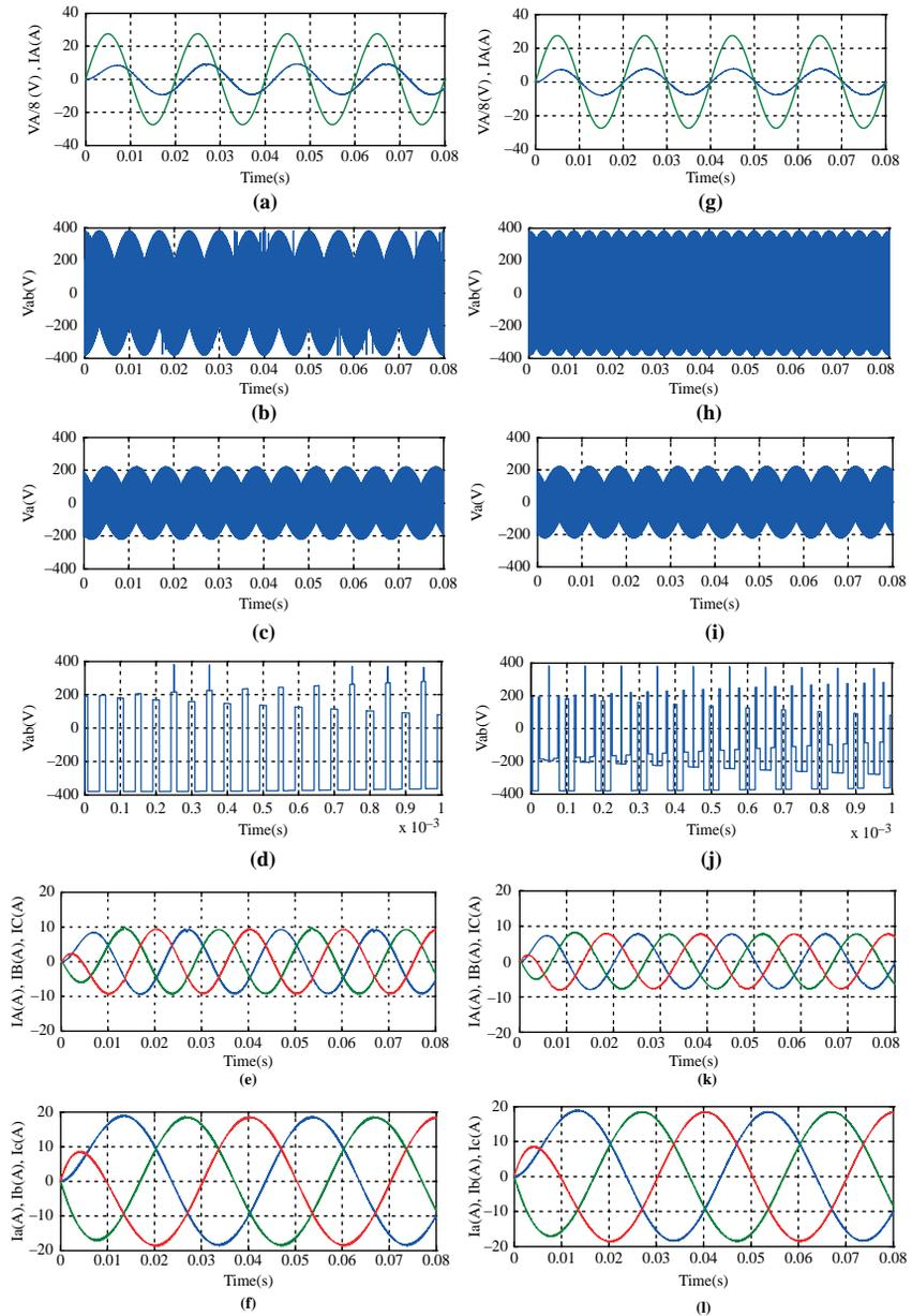
**Notes:** (a)-(f) Without current control and (g)-(l) with current control; (a) and (g) input current and voltage, respectively; (b) and (h) output line voltage; (c) and (i) output phase voltage; (d) and (j) output line voltage magnified; (e) and (k) input currents; (f) and (l) output currents
