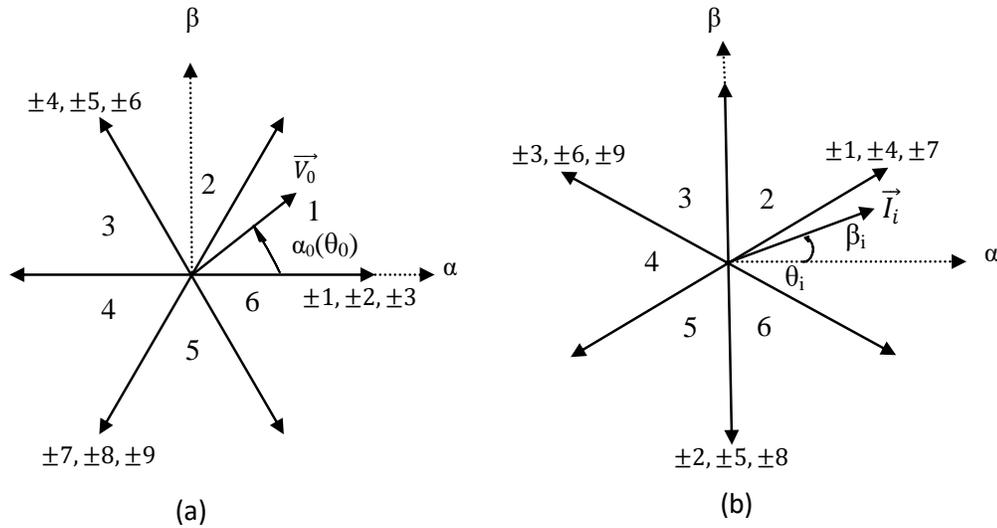
Figure 5.9 (a) Voltage space vector (b) Current space vector
