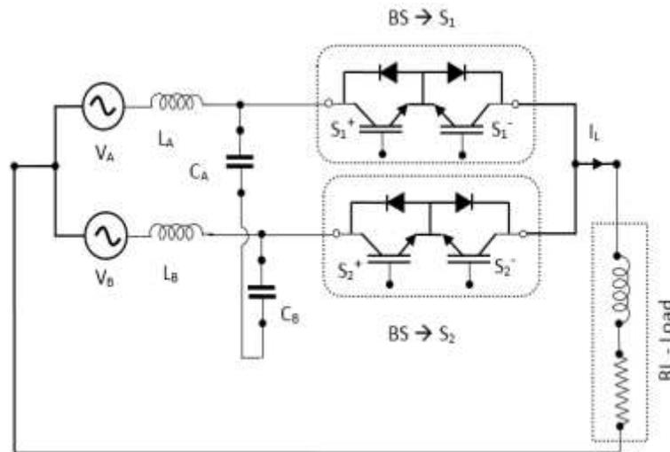
Figure 1.8 Commutation of the bidirectional switches between the two input phases
