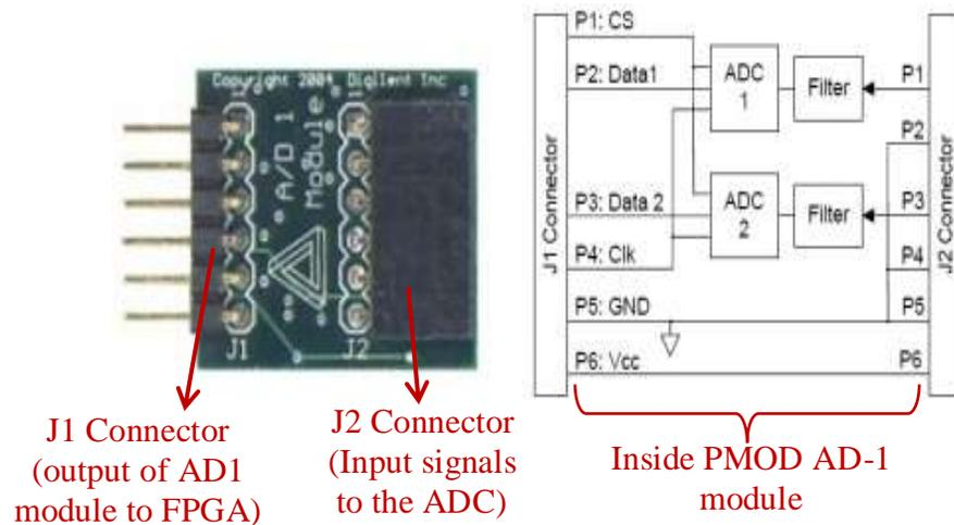
Figure 7.2 Digilent PMOD AD1 board and pin description
