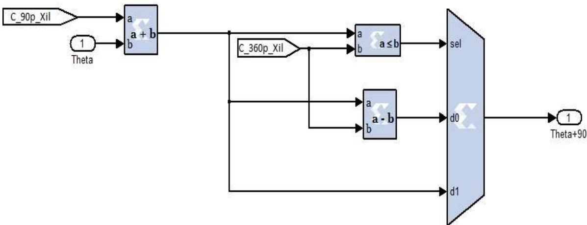
Figure 6.14 Conversion of  $\theta$  to  $\theta+90^\circ$  in order to calculate  $\cos\theta_r$
