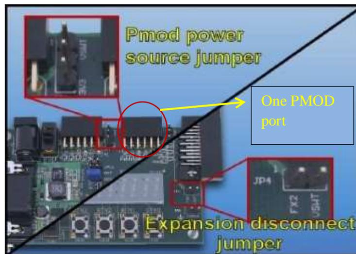
Figure 7.1 PMOD power source jumper
