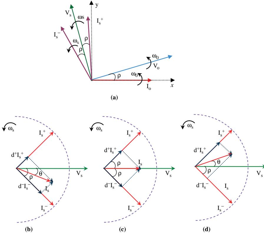
**Notes:** (a) Input current positions; (b) lagging power factor ( $d^+ < d^-$ ); (c) unity power factor ( $d^+ = d^-$ ); (d) leading power factor ( $d^- > d^+$ )
