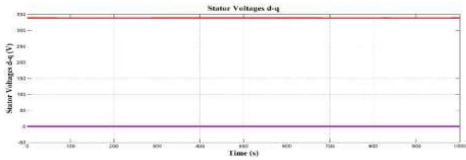
Figure 3.19 Stator voltages in d-q coordinates
