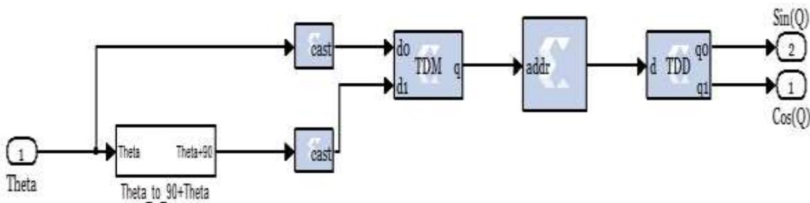
Figure 6.13 Matlab/Xilinx model to calculate  $\sin\theta_r$  and  $\cos\theta_r$  from slip angle  $\theta_r$
