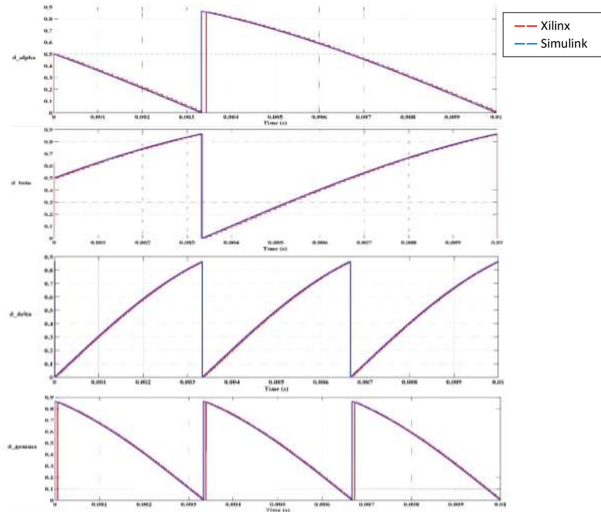
Figure 5.25 Duty cycles of the VSV and CSV from Xilinx and Simulink
