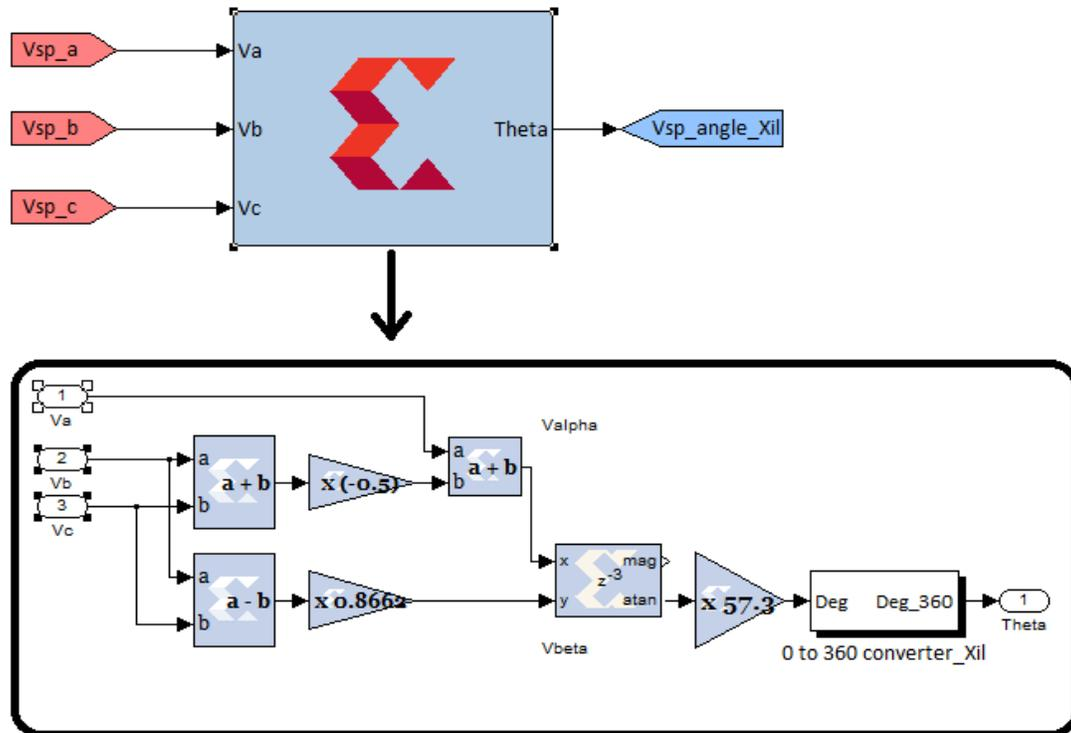
Figure 6.6 Matlab/Xilinx model for calculating theta
