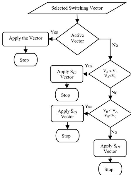
Fig. 6. Algorithm for common mode voltage reduction
