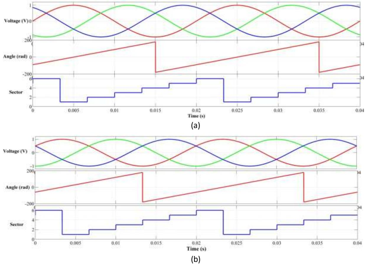
Figure 5.11 CSV sector computation using (a) conventional method (b) proposed method
