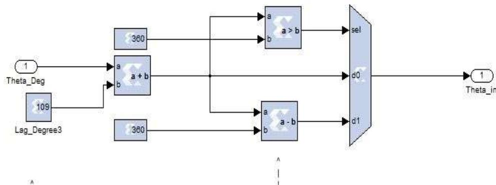
Figure 8.20 Matlab/Xilinx model for generating theta with the lag correction within the limit of  $360^\circ$
