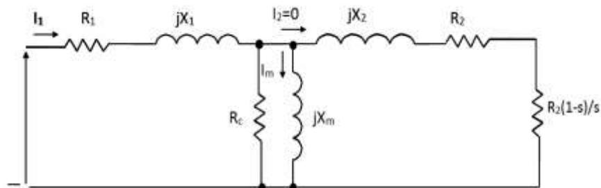
Figure 3.4 (a) Initial equivalent circuit
