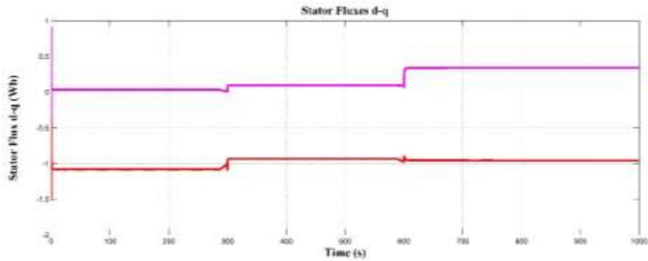
Figure 3.12 Stator flux in d-q coordinates
