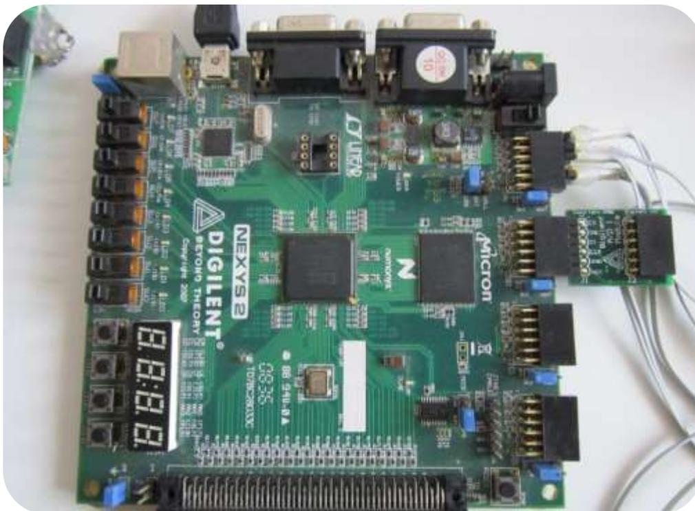
Figure 10.22 FPGA controller unit - Sparten 3E
