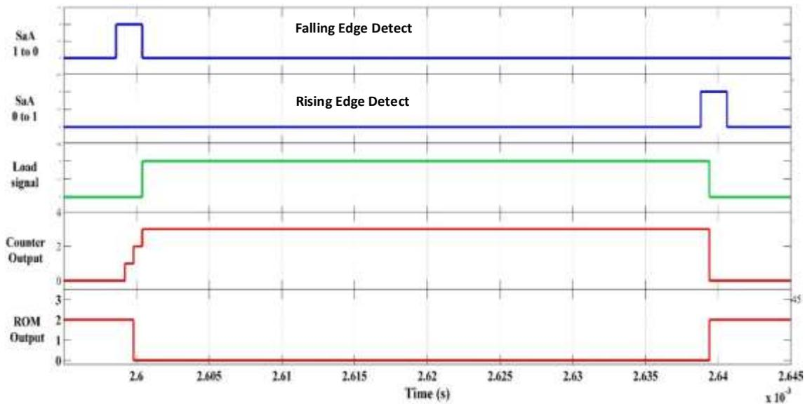
Figure 5.44 Counter output for positive current when a Falling Edge is detected
