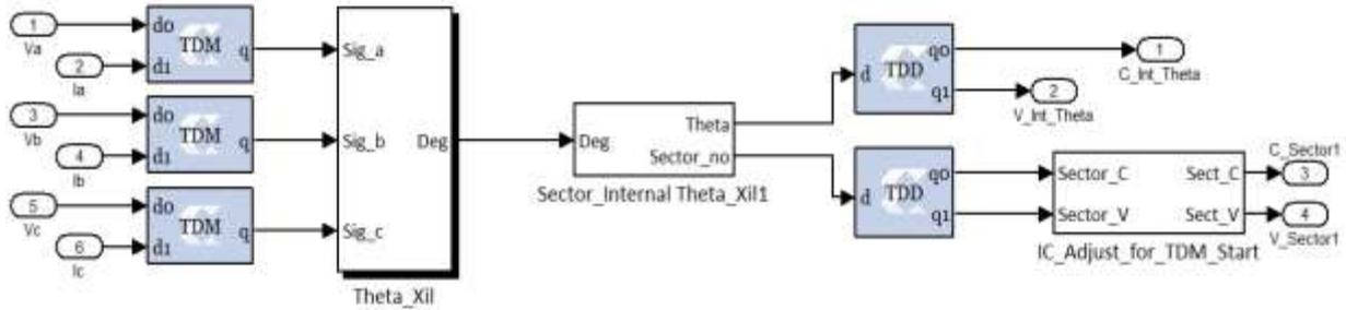
Figure 5.15 Time-multiplexing of voltage and current reference vectors for computation of sectors
