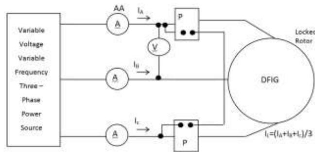
Figure 3.5 Circuit diagram for the blocked rotor test
