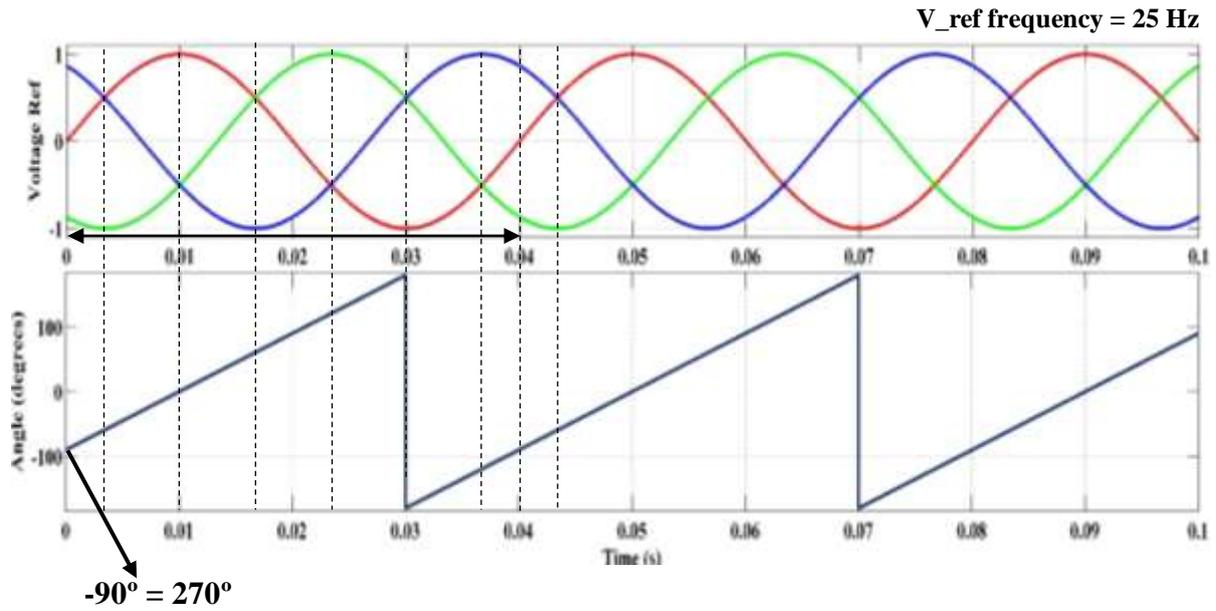
Figure 2.14 Angle of Voltage Reference with respect to “ $\alpha$ ” axis,  $\alpha_0$
