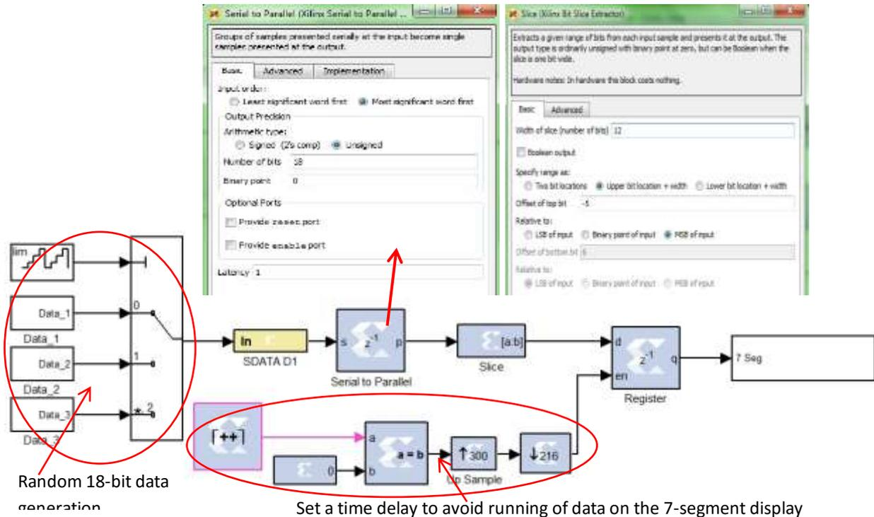
Figure 7.8 Serial to parallel block in Xilinx
