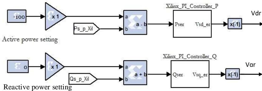
Figure 6.10 PI controller to control the stator active power and reactive power
