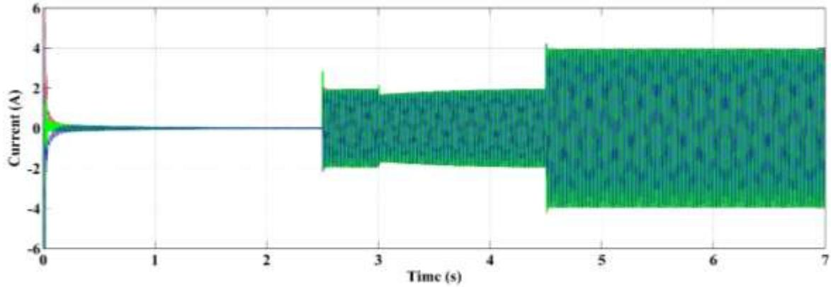
Figure 4.10 Stator currents  $I_{sabc}$  versus time
