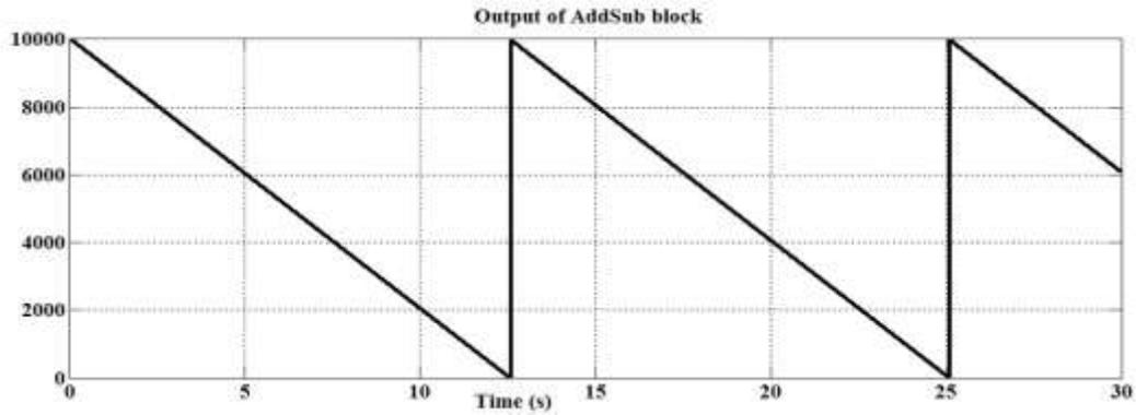
Figure 9.14 Output of the Add-Sub Block
