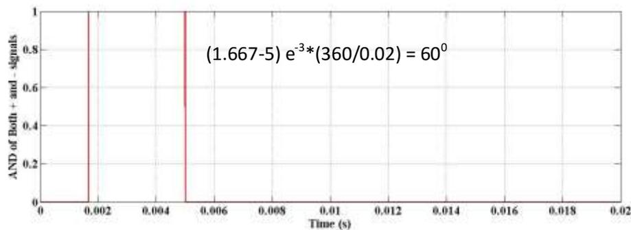
Figure 8.5 'AND' of the most positive and negative instant
