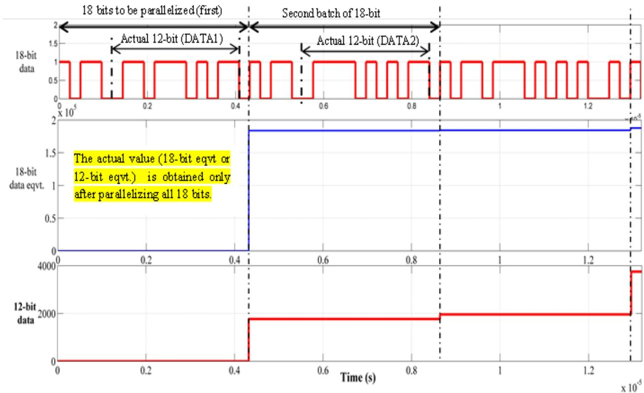
Figure 7.9 Working of serial-parallel block
