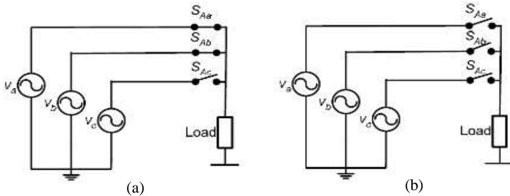
Figure 2.1 Non-Acceptable switch states in MC
