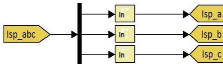
Figure.6.5 Matlab/Xilinx model of the stator currents  $I_{sp\_abc}$
