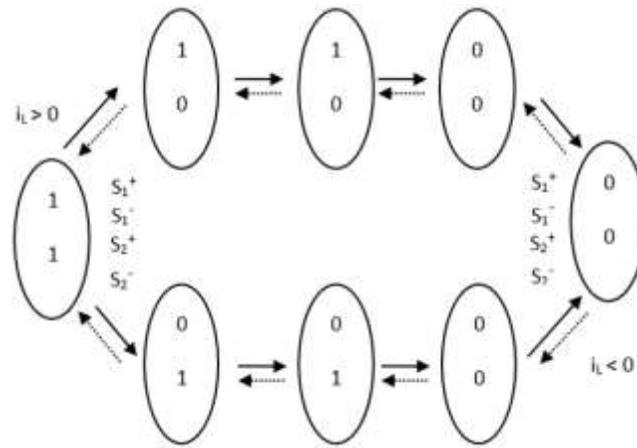
Figure 1.9 State diagram of the four-step current commutation
