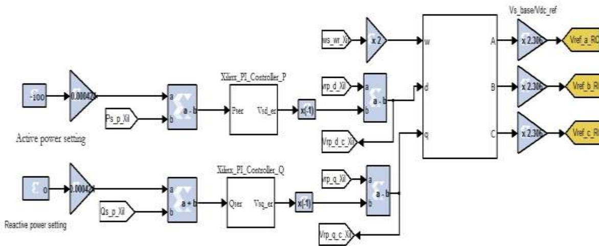
Figure 6.17 Active power and reactive power controllers and generation of the reference signals for the matrix converter fed DFIG based wind energy conversion system
