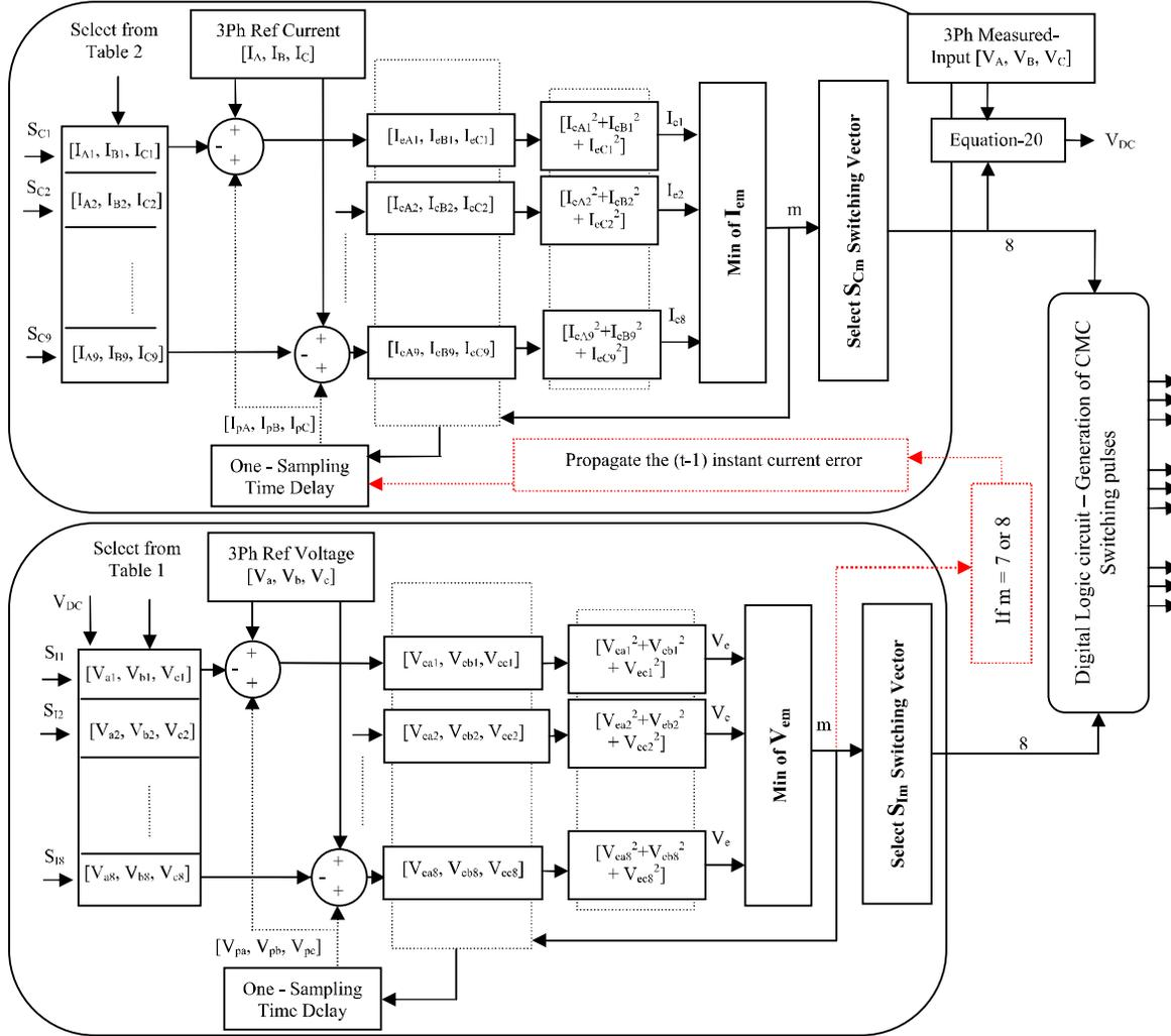
Fig. 5. Parallel Execution Sequence of MESS Algorithm
