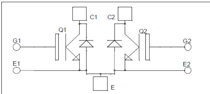
Figure 10.4 (b) Internal connection diagram of APTGT150DU120G
