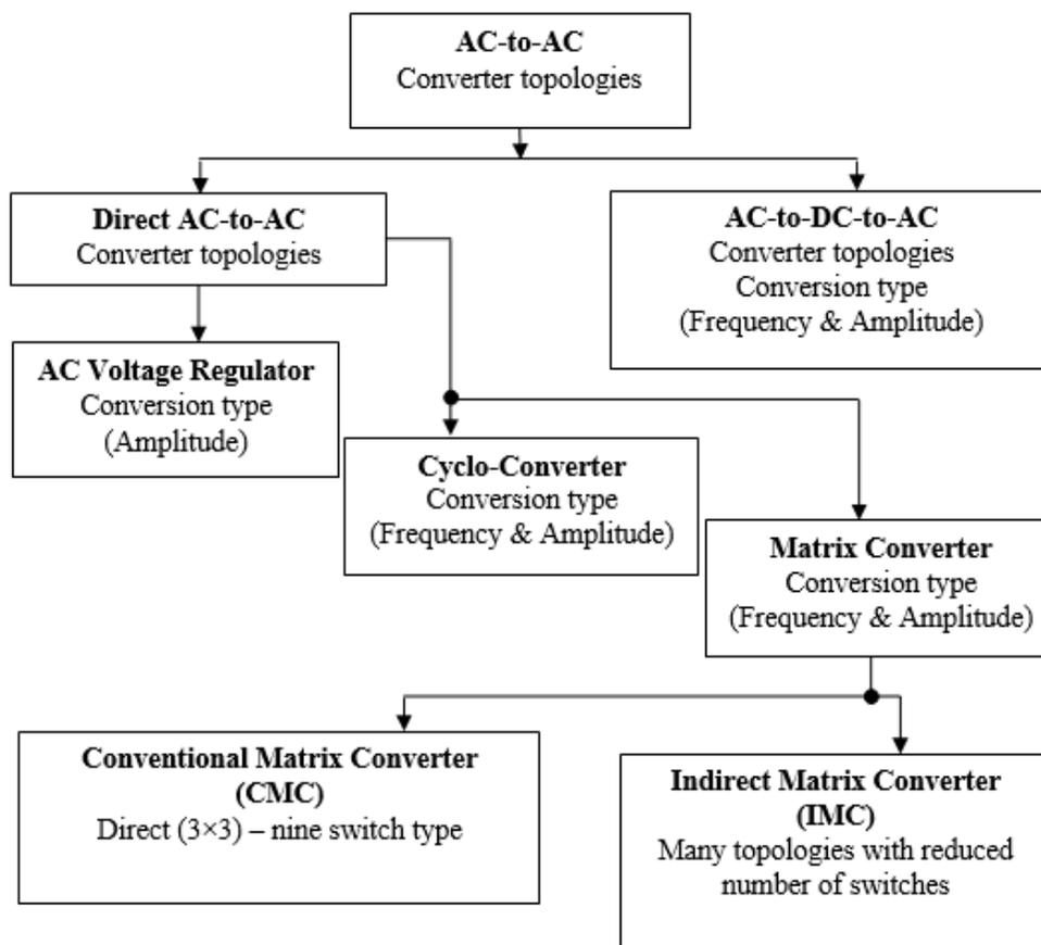
Figure 1.5 AC-to-AC converter topologies
