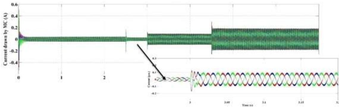
Figure 4.9 (b) Matrix converter input current versus time
