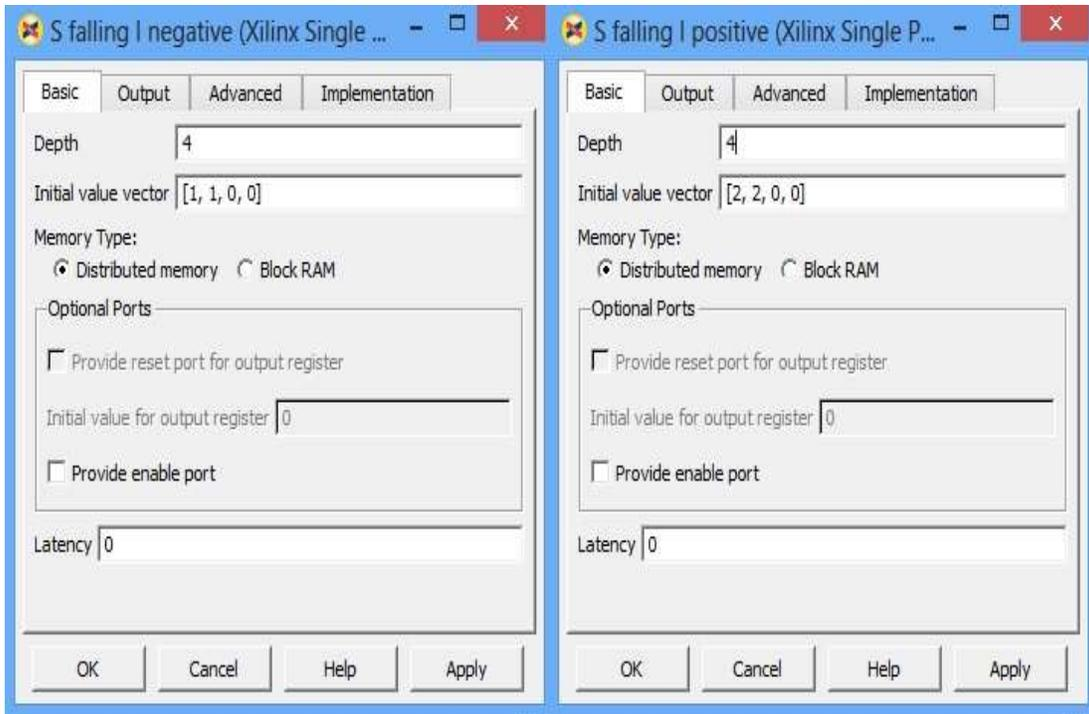
Figure 5.41 Commutation sequence stored in ROM when the switch is to be turned OFF
