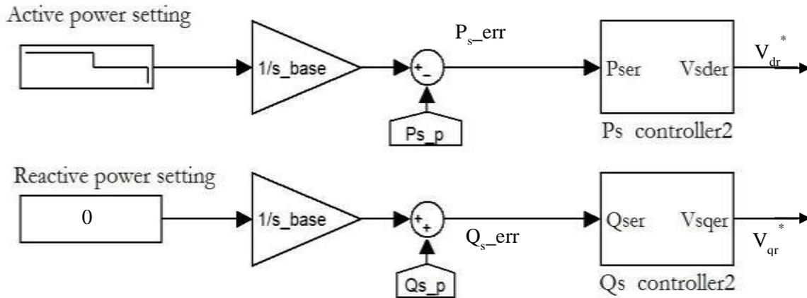
Figure 4.1 Matlab/Simulink Model for the rotor side controller
