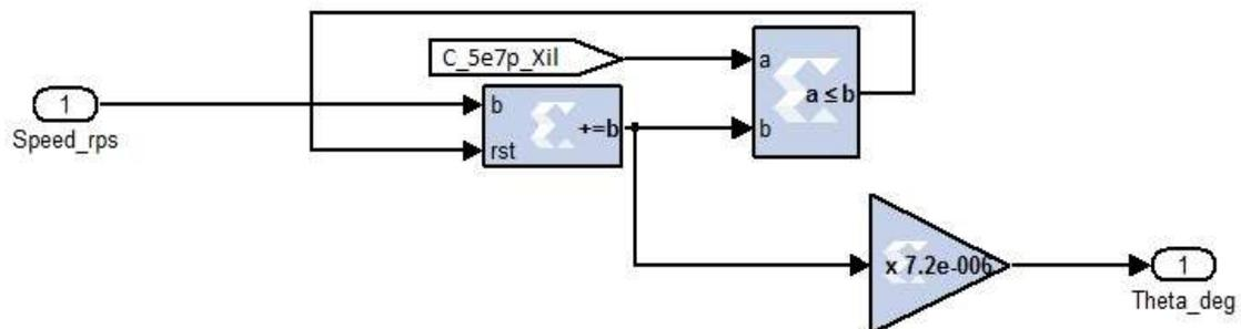
Figure 6.12 Matlab/Xilinx model for converting the slip speed to slip angle  $\theta_r$
