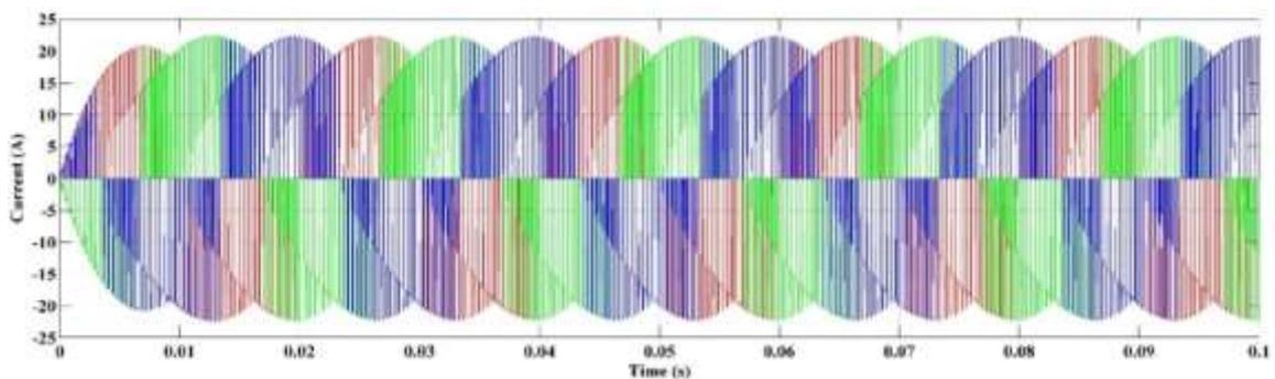
Figure 2.38 3-phase Input current of MC without input filter
