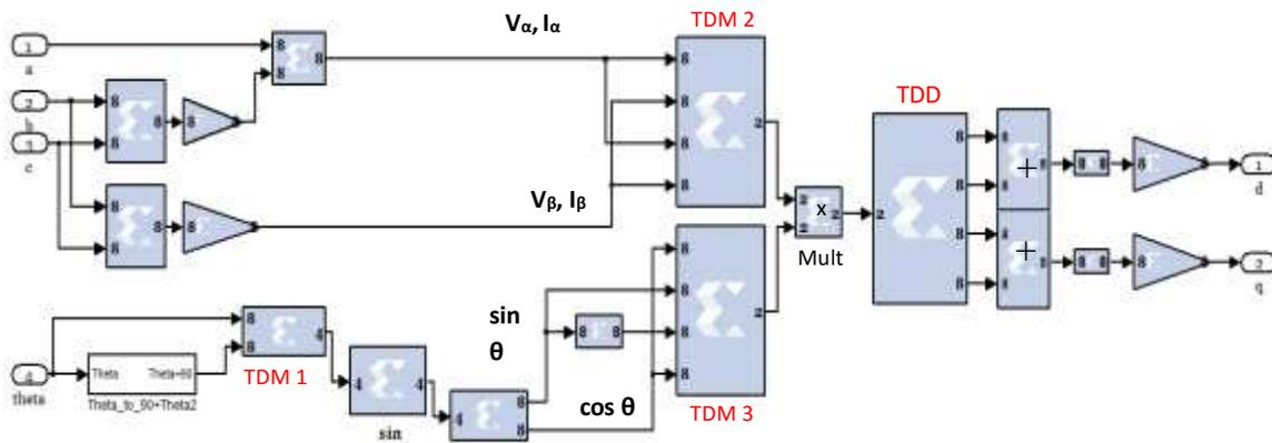
Figure 5.2 abc-dq transformation of the voltage and the current
