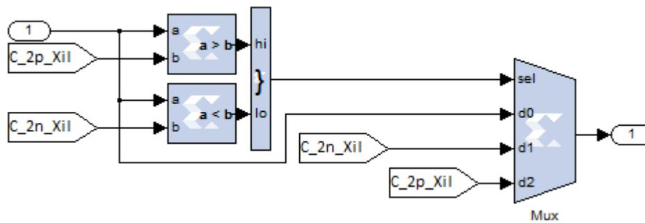
Figure 6.2 Matlab/Xilinx model of the saturation unit
