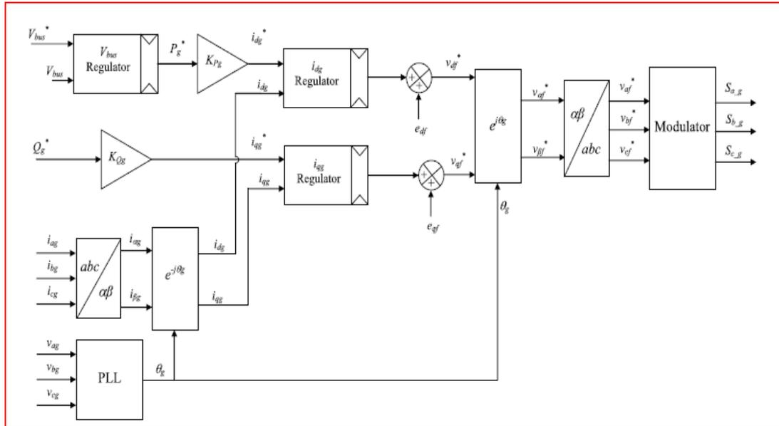
Figure 1.3 Grid voltage oriented vector control scheme for the grid side controller
