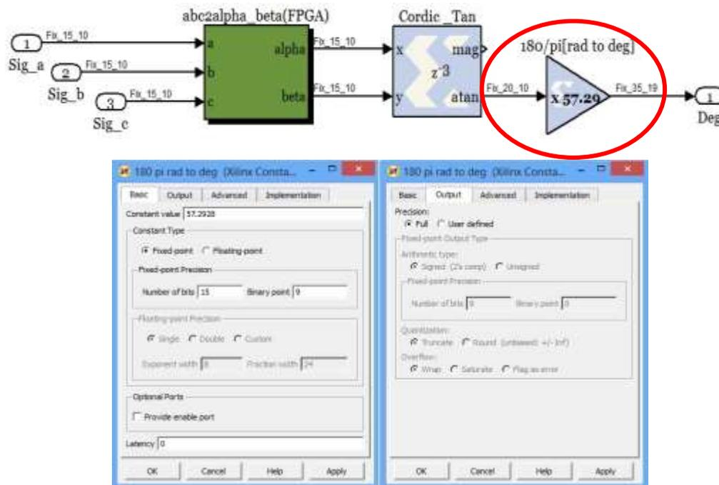
Figure 5.7 Bit requirement when the output of the block is FULL
