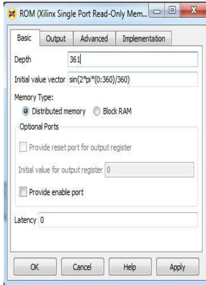
Figure 6.15 Parameters of the ROM Block to calculate  $\sin\theta_r$  and  $\cos\theta_r$
