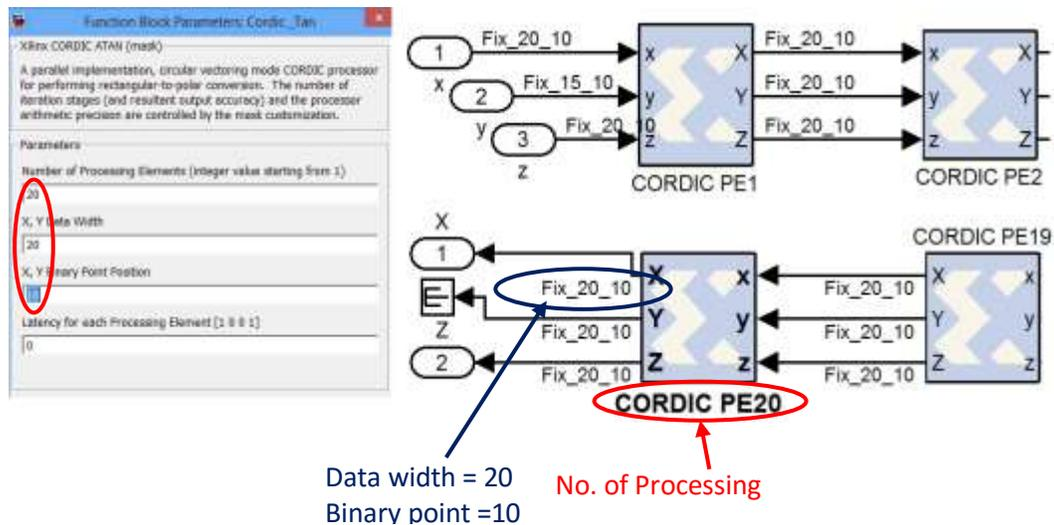
Figure 5.17 Settings of the Cordic aTan block
