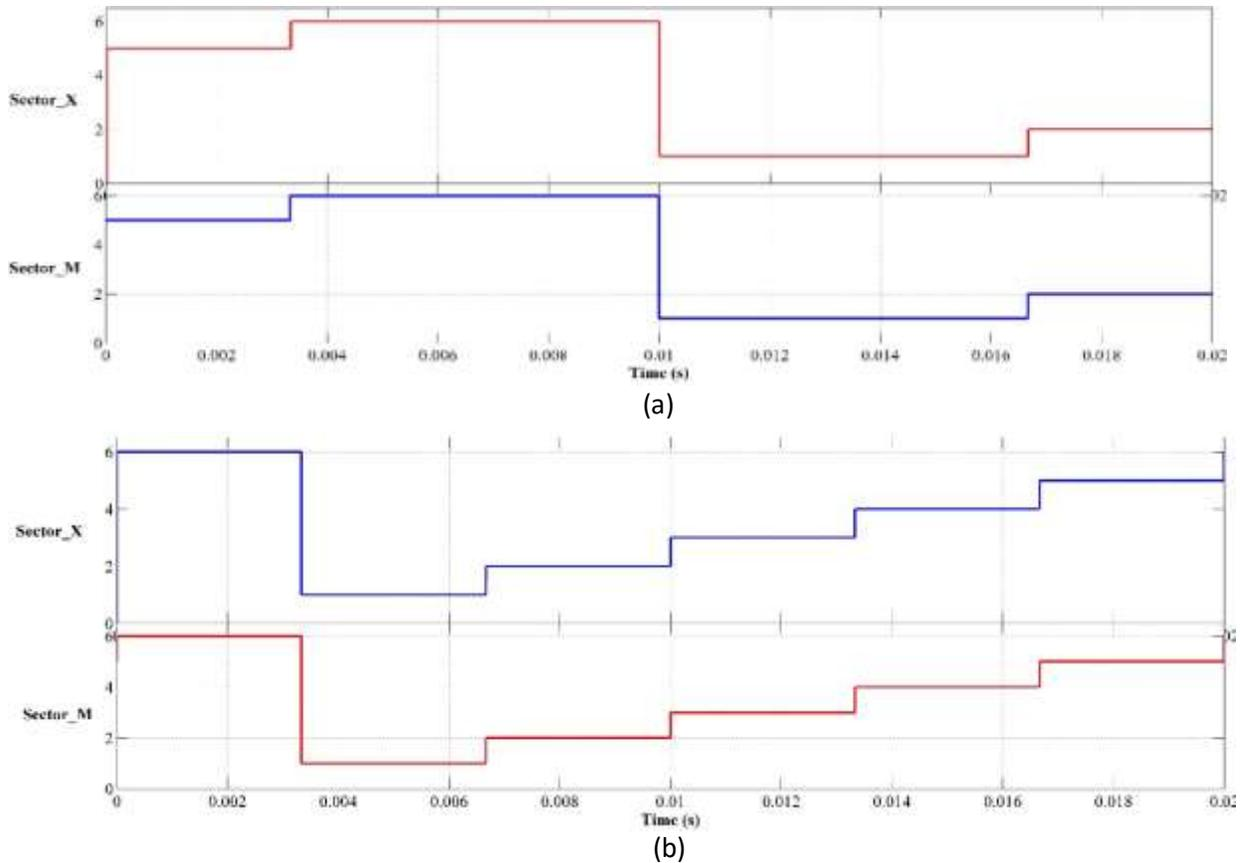
Figure 5.20 Sectors obtained from Xilinx and Simulink (a) VSV Sectors (b) CSV Sectors
