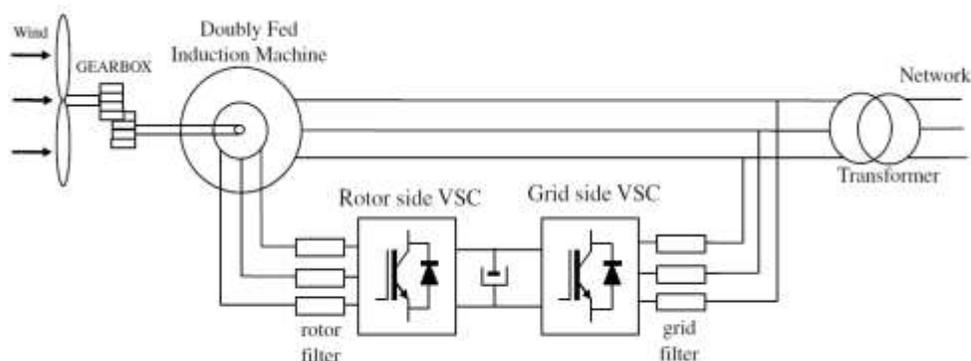
Figure 1.1 Conventional variable speed wind energy conversion system
