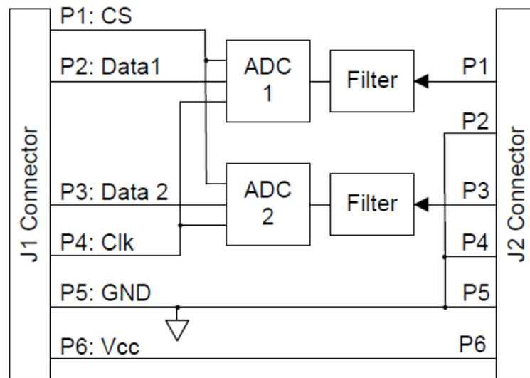
Figure 10.24 PMOD AD1 and the internal block diagram
