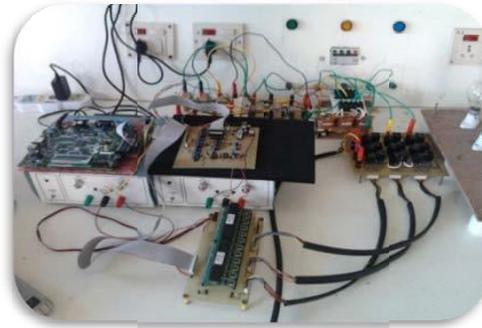
Fig. 11. Matrix Converter Hardware Prototype
