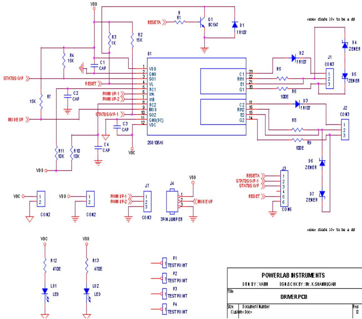
Figure 10.12 Circuit Diagram of the driver module
