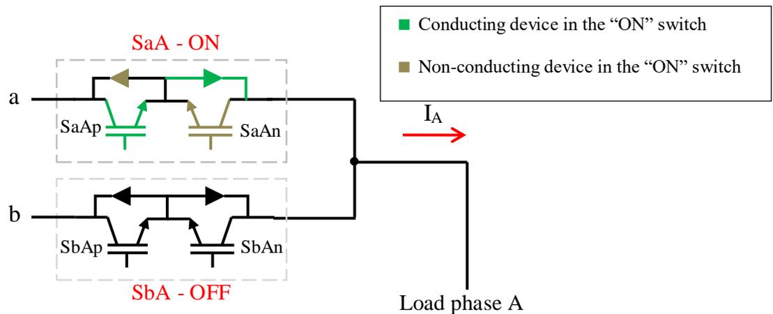
Figure 2.32 Load phase A connected to the input phase ‘a’
