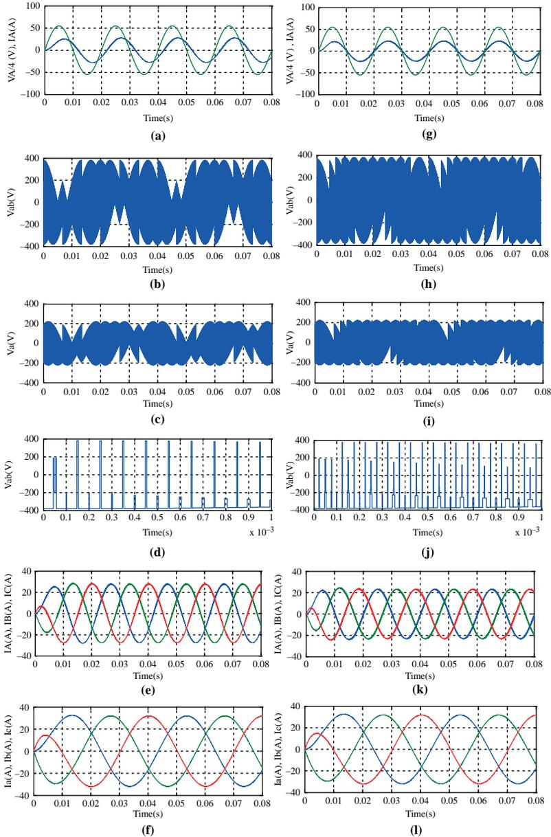
**Notes:** (a)-(f) Without current control and (g)-(l) with current control; (a) and (g) input current and voltage, respectively; (b) and (h) output line voltage; (c) and (i) output phase voltage; (d) and (j) output line voltage magnified; (e) and (k) input currents; (f) and (l) output currents
