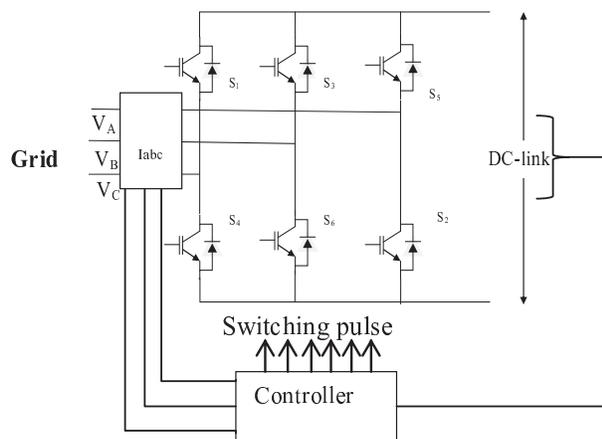
Fig. 3 Grid side converter
