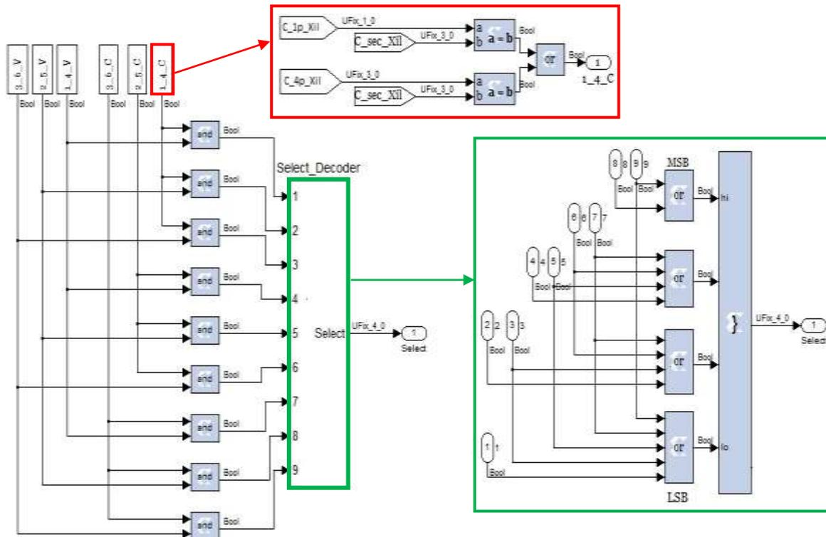
Figure 5.30 Switch state selection
