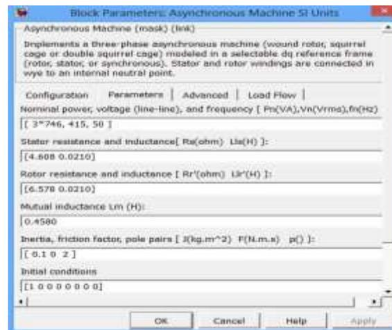
Figure 3.8 Parameters entered in Matlab/Simulink model
