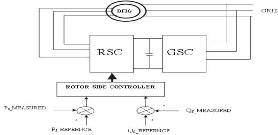
Fig. 5 Block diagram of the RSC
