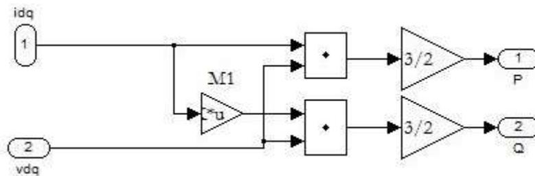
Figure 3.17 Matlab/Simulink Model for calculating the rotor power
