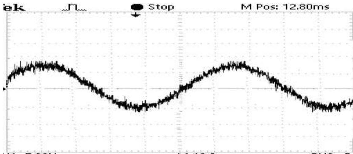
Figure 10.32 Output current of matrix converter with RL Load
