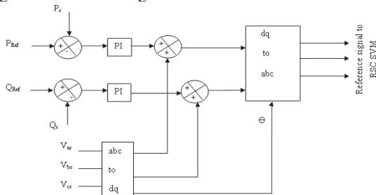
Fig. 6 Rotor side controller
