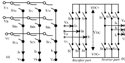
Figs. 1. (a) Conventional Matrix Converter, (b) Back to Back Converter
