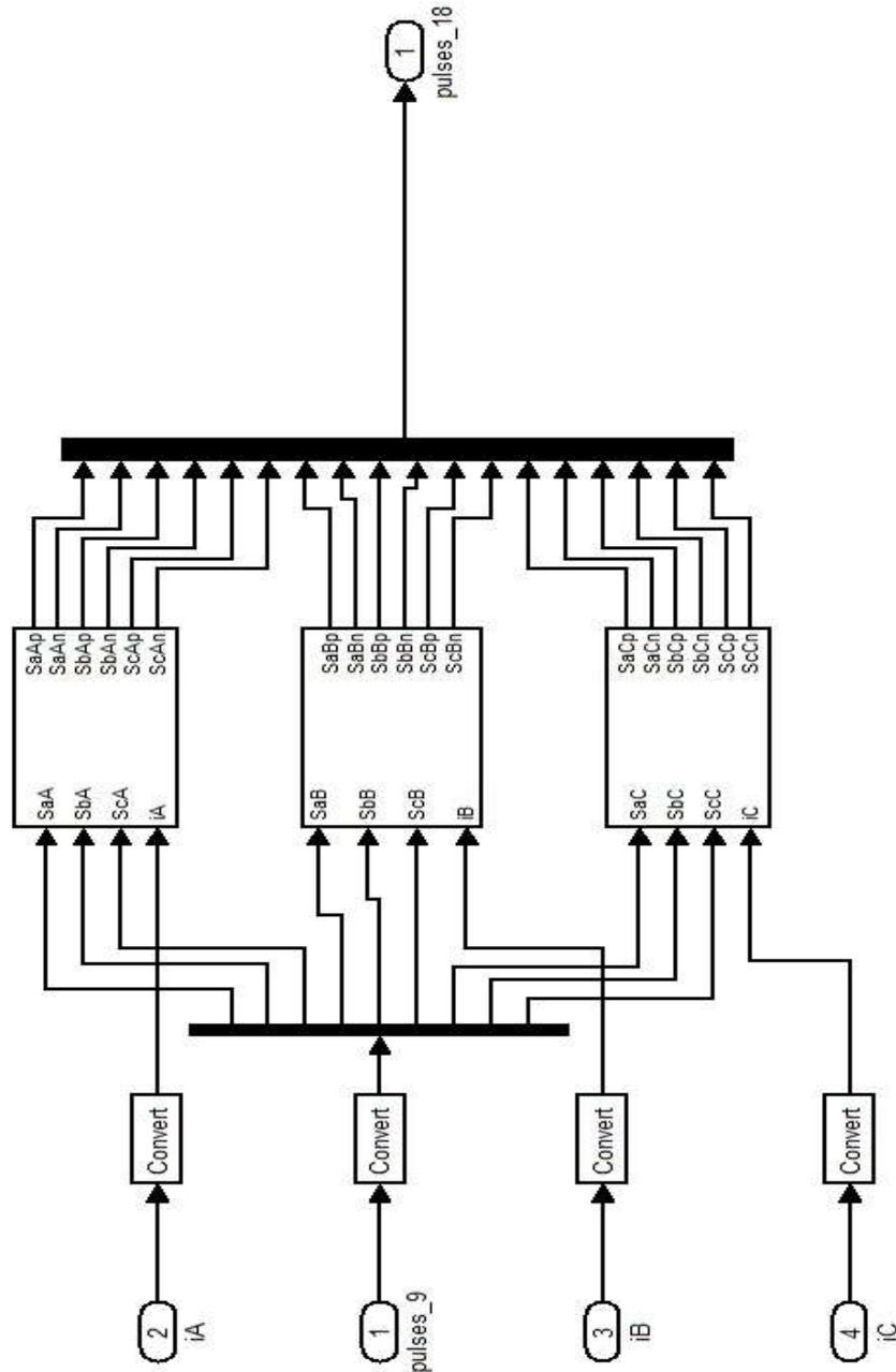
Figure 2.35 Four step sequencer for all load phases.
