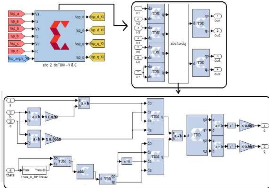
Figure 6.7 Transformation of the three-phase voltages and currents into two-phase synchronously rotating voltages and currents using the TDM
