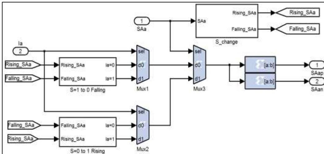
Figure 5.37 Block diagram of commutation sequencer for switch  $S_{aA}$
