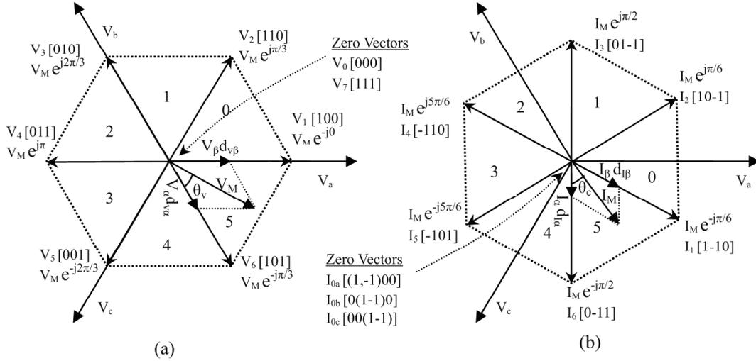
Figure 2. (a) Inverter voltage hexagon and (b) rectifier current hexagon.
