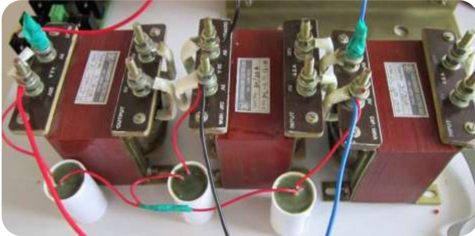
Figure 10.15 Input filter circuit
