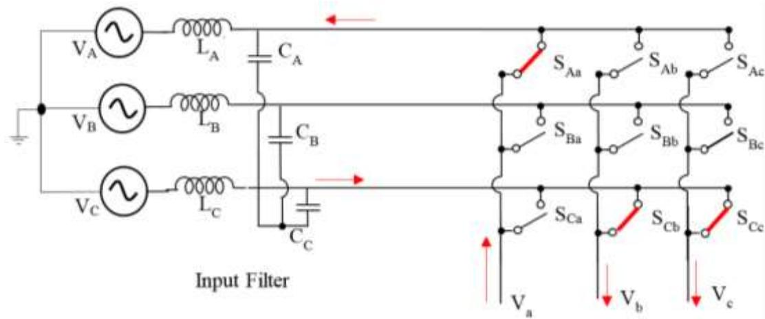
Figure 2.2 Switch state [acc] in the MC
