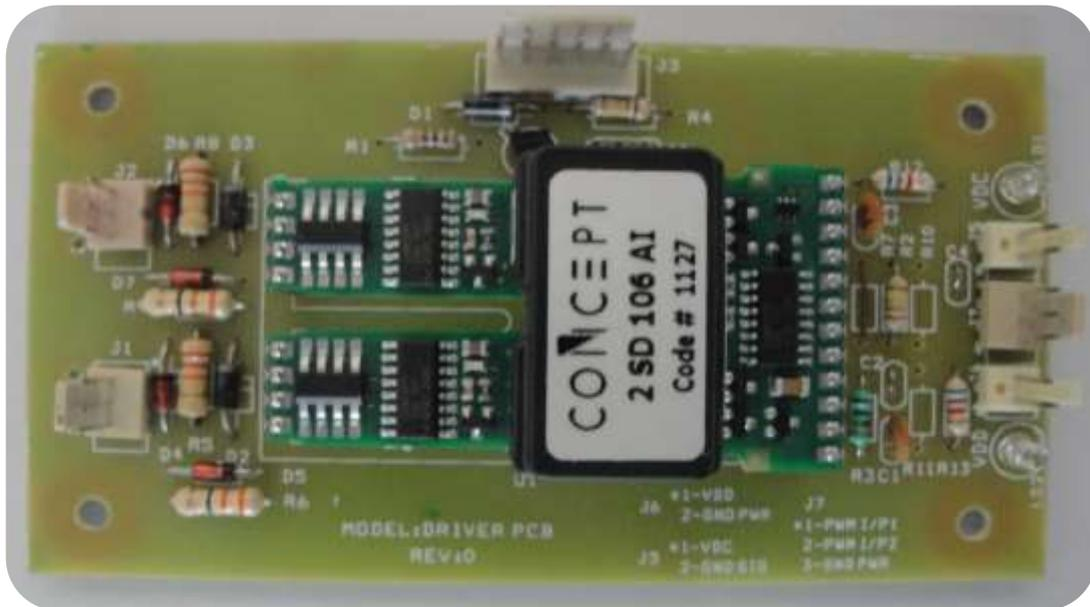
Figure 10.13 Concept Driver Module
