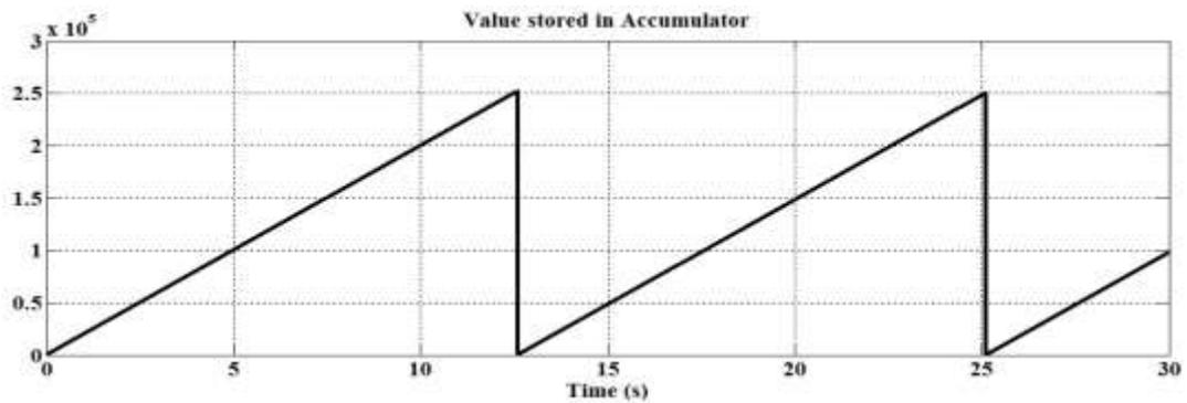
Figure 9.15 Value stored in the accumulator during repeated subtraction
