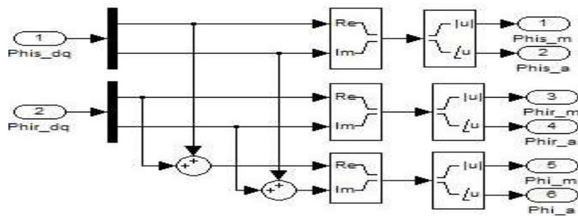
Figure 3.11 Matlab/Simulink model to calculate the magnitude of the flux in the DFIG
