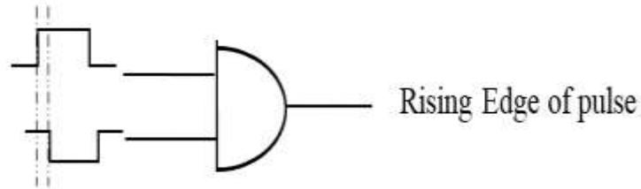
Figure 9.3: AND gate to detect the rising edge of any pulse
