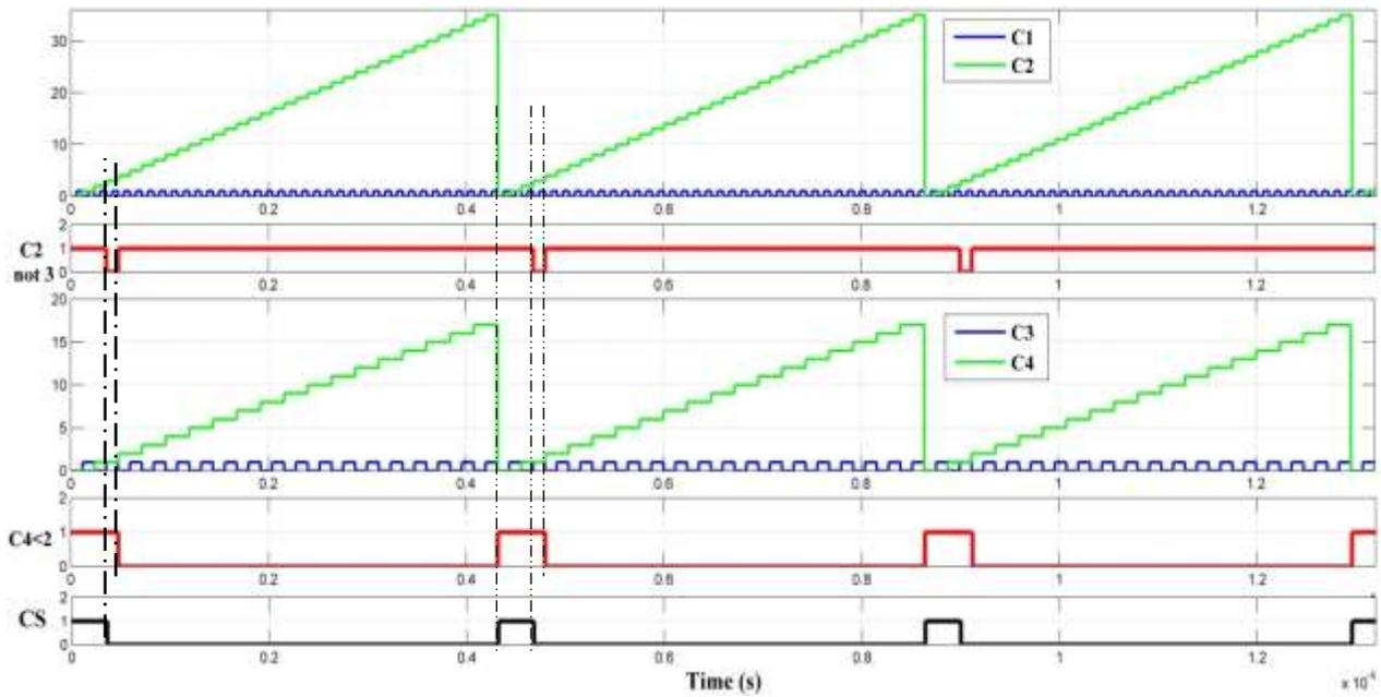
Figure 7.6 Generation of the Chip Select signal
