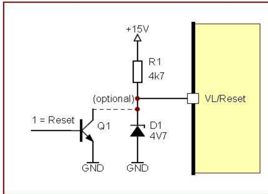
Figure 10.8 Circuit for input VL/reset for 5 V logic
