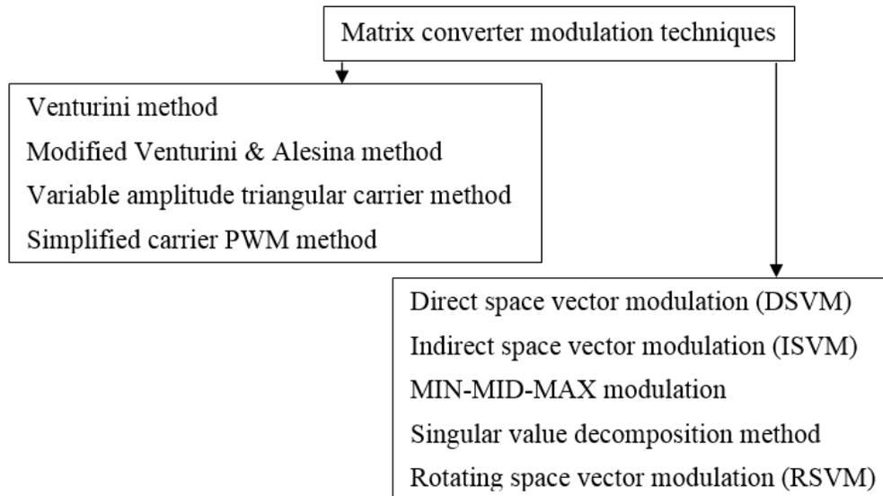
Figure 1.10 Classification of the matrix converter modulation techniques
