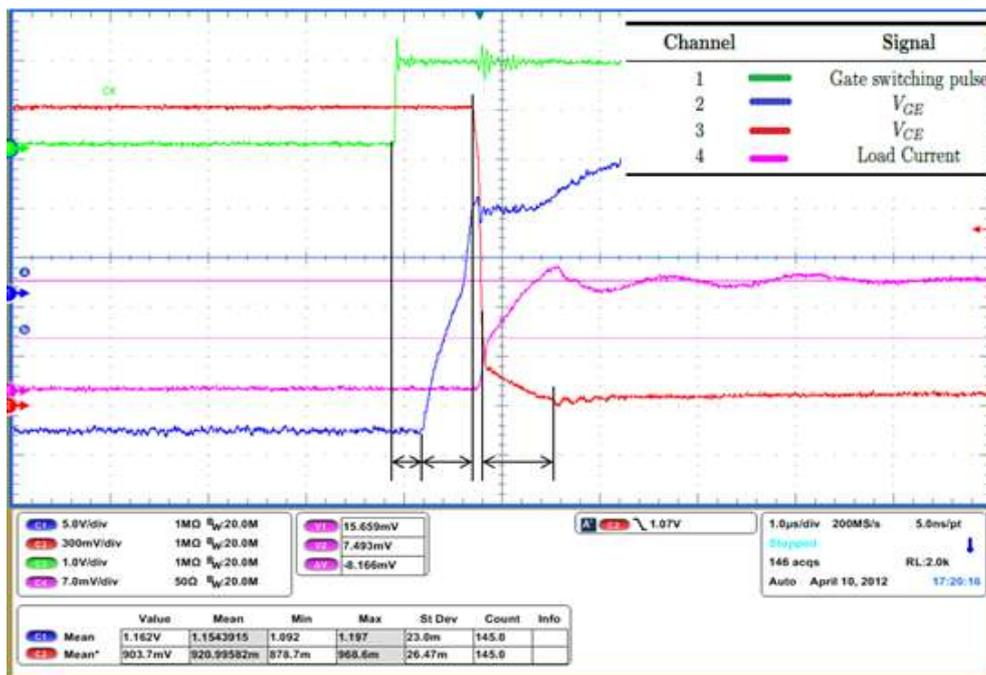
Figure 10.5(a) IGBT Turn-ON characteristics
