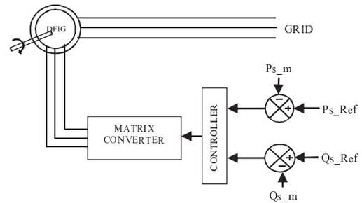
Fig. 4. Block diagram of the DPC for the MC-based DFIG system
