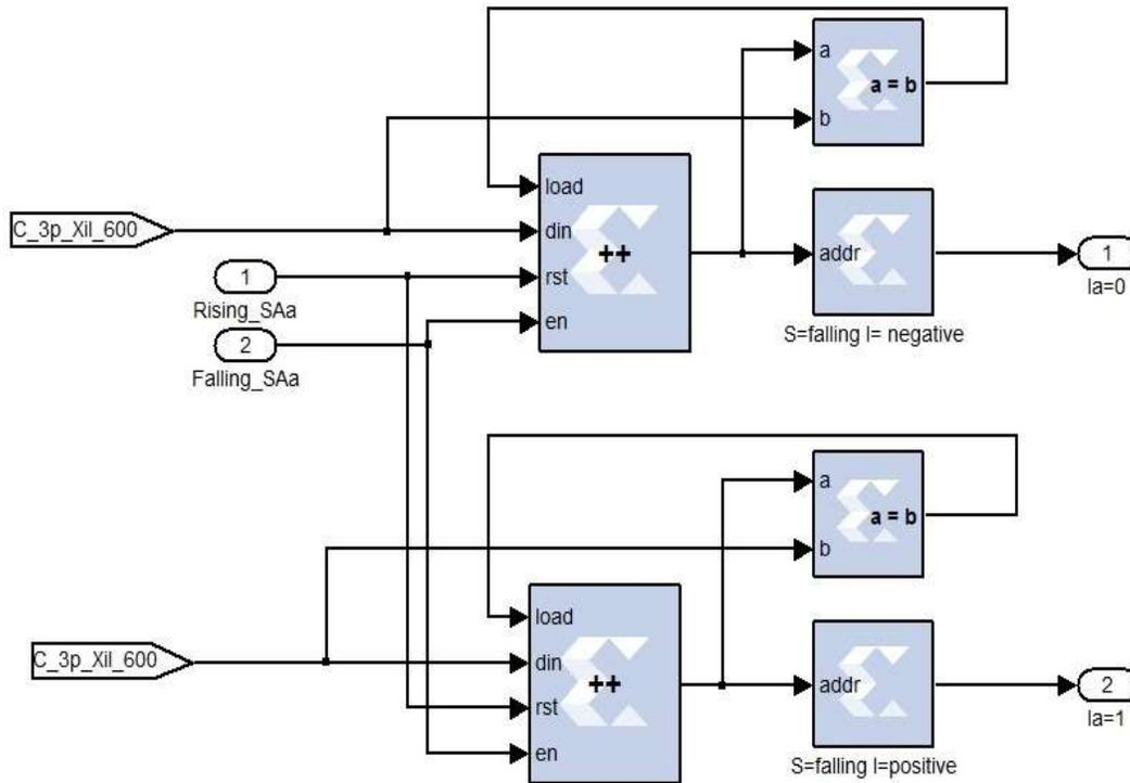
Figure 5.40 Commutation sequence generation when a falling edge is detected
