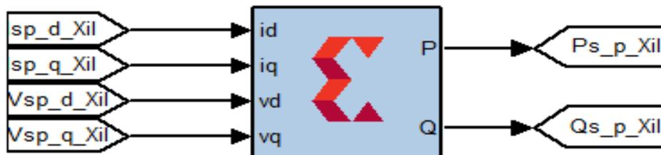
Figure 6.8 Sub-system to calculate the stator active power and reactive power in Matlab/Xilinx
