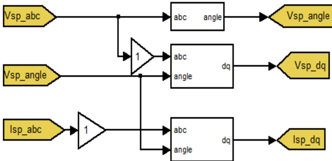
Figure 4.2 Matlab/Simulink model for calculating voltages, currents and voltage angle in the dq rotating frame
