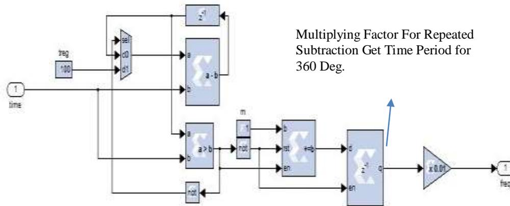
Figure 8.15 Matlab/Xilinx model to calculate the frequency of the signal from the calculated time-period using repeated subtraction
