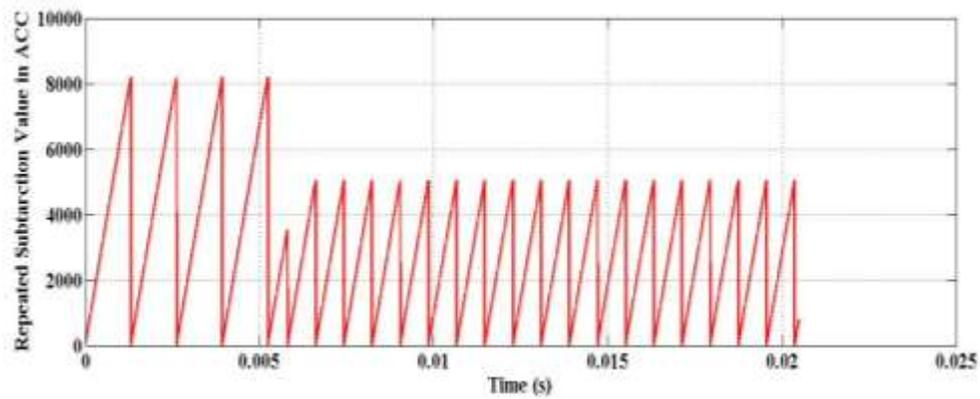
Figure 8.16 Results stored in the accumulator after every repeated subtraction
