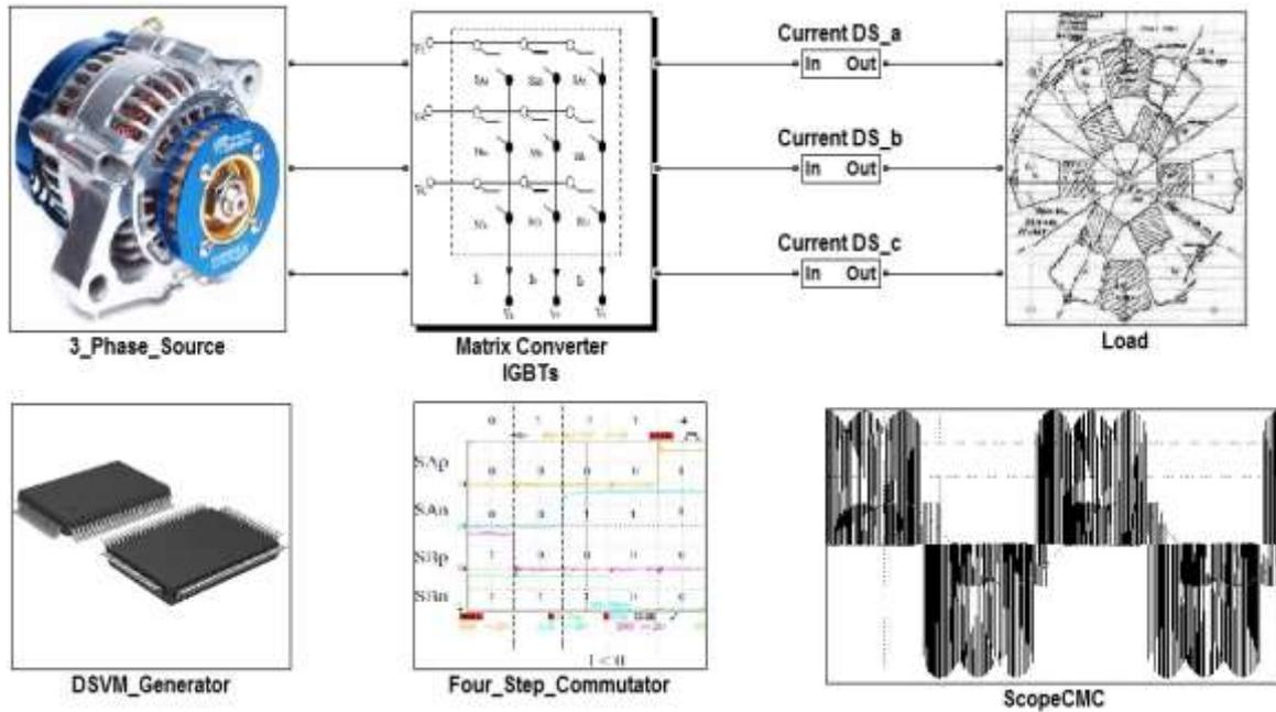
Figure 2.8 Setup of the MC triggered using DSVM
