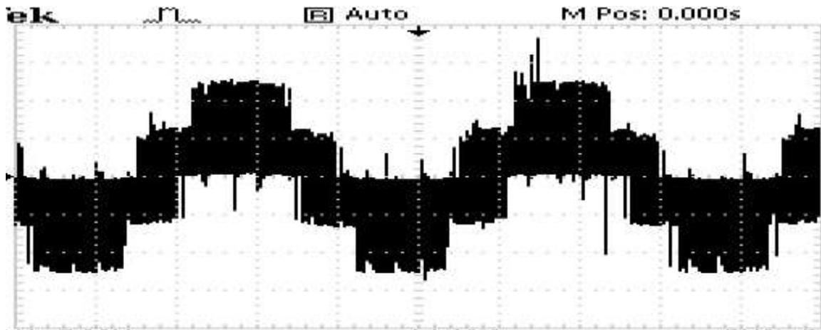
Figure 10.30 (a) Output Phase voltage of matrix converter with RL load
