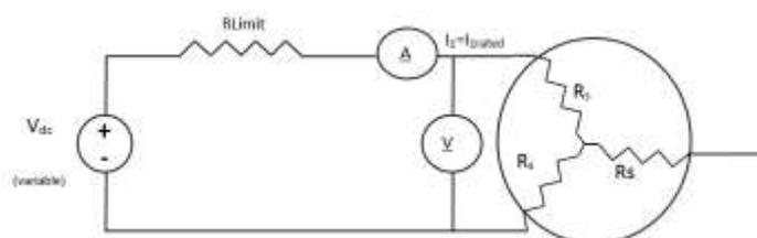
Figure 3.2 Test circuit for the DC resistance test
