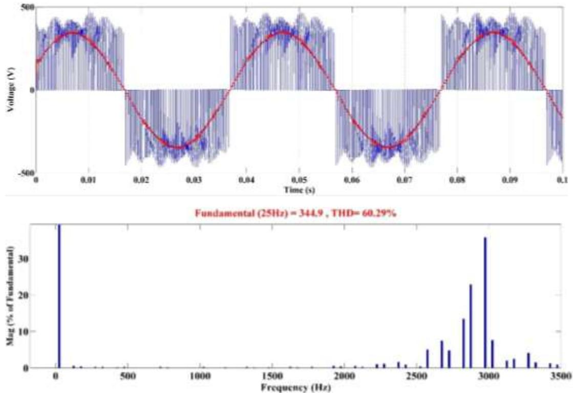
Figure 2.42 Output line-to-line voltage and its harmonic spectrum with input filter
