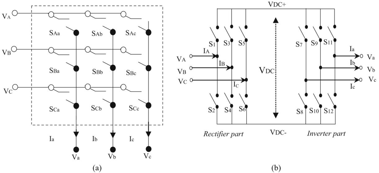
Figure 1. (a) Conventional MC and (b) MC as two stage converter.
