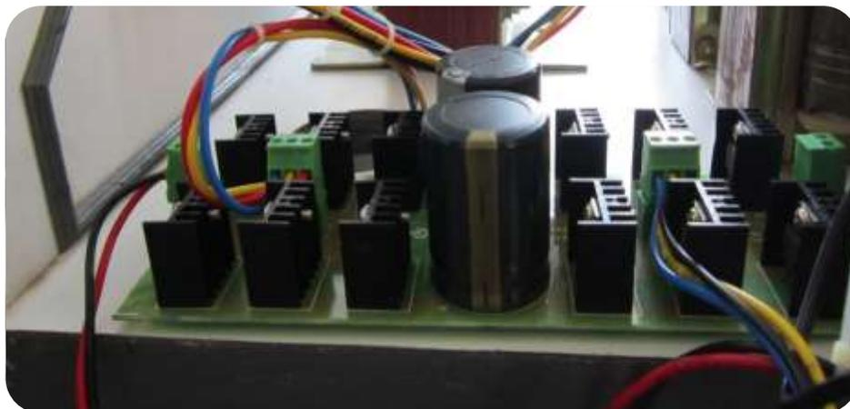
Figure 10.14 Matrix converter clamp circuit
