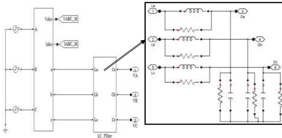
Figure 2.9 Source side of the MC
