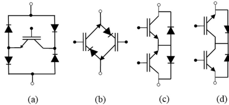
Figure 1.7 Four-quadrant bidirectional switches (a) diode-embedded switch (b) reverse blocking IGBT (c) common emitter IGBT and (d) common collector IGBT
