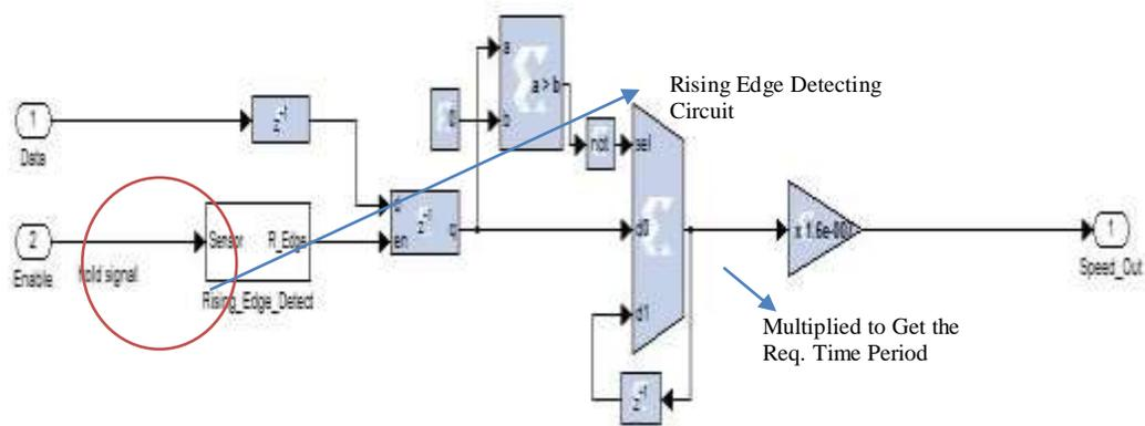
Figure 8.9 Matlab/Xilinx Model to calculate the Time Period of the Captured Signal
