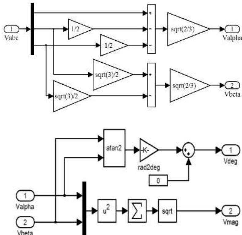
Figure 2.13  $\alpha$ - $\beta$  Transformation of reference voltage and its angle in  $\alpha$ - $\beta$  plane
