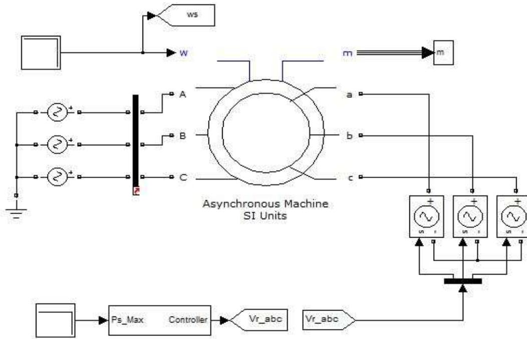
Figure 3.23 Matlab/Simulink model of the DFIM as a generator
