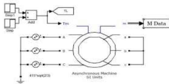
Figure 3.7 Matlab/Simulink model of the DFIG Machine
