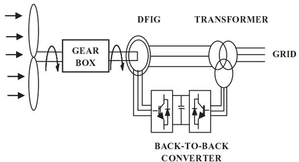
Fig. 1 Block diagram of the back-to-back converter based DFIG
