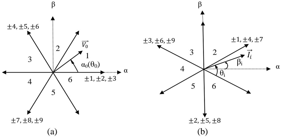
Figure 2.6 (a) Output voltage SSVs (b) Input current SSVs
