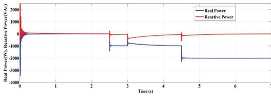
Fig. 6. Stator active and reactive powers
