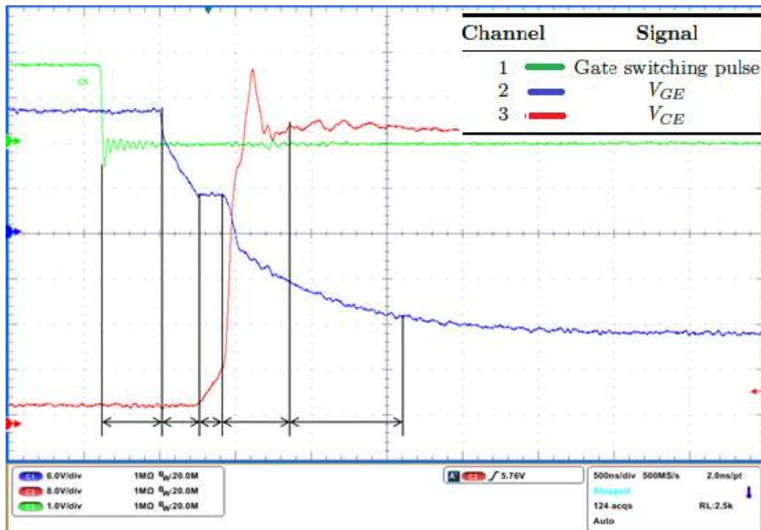
Figure 10.5(b) IGBT turn-OFF characteristics
