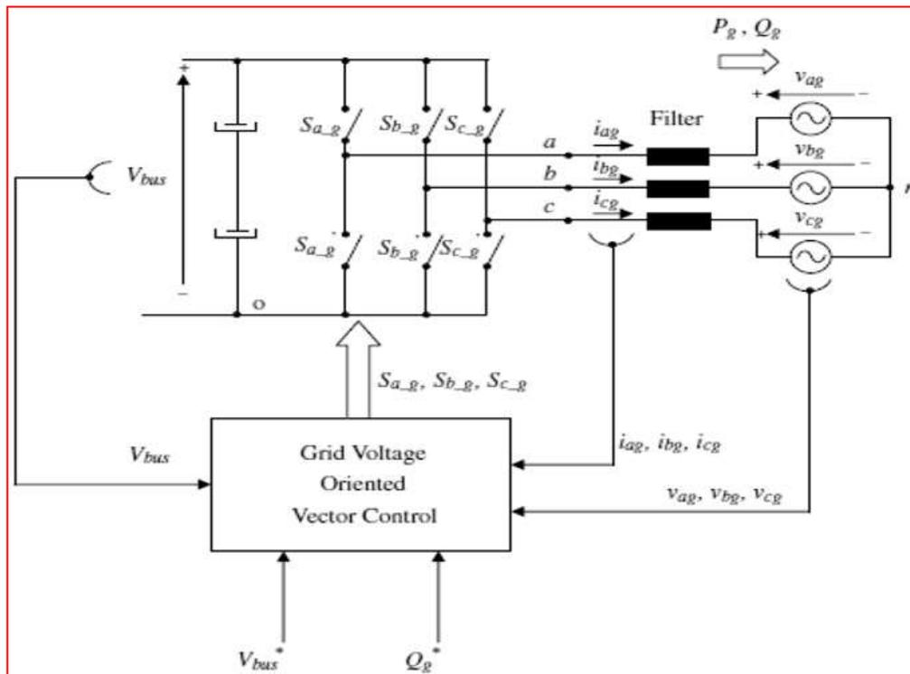
Figure 1.2 Grid side control scheme for the conventional back-to-back converter
