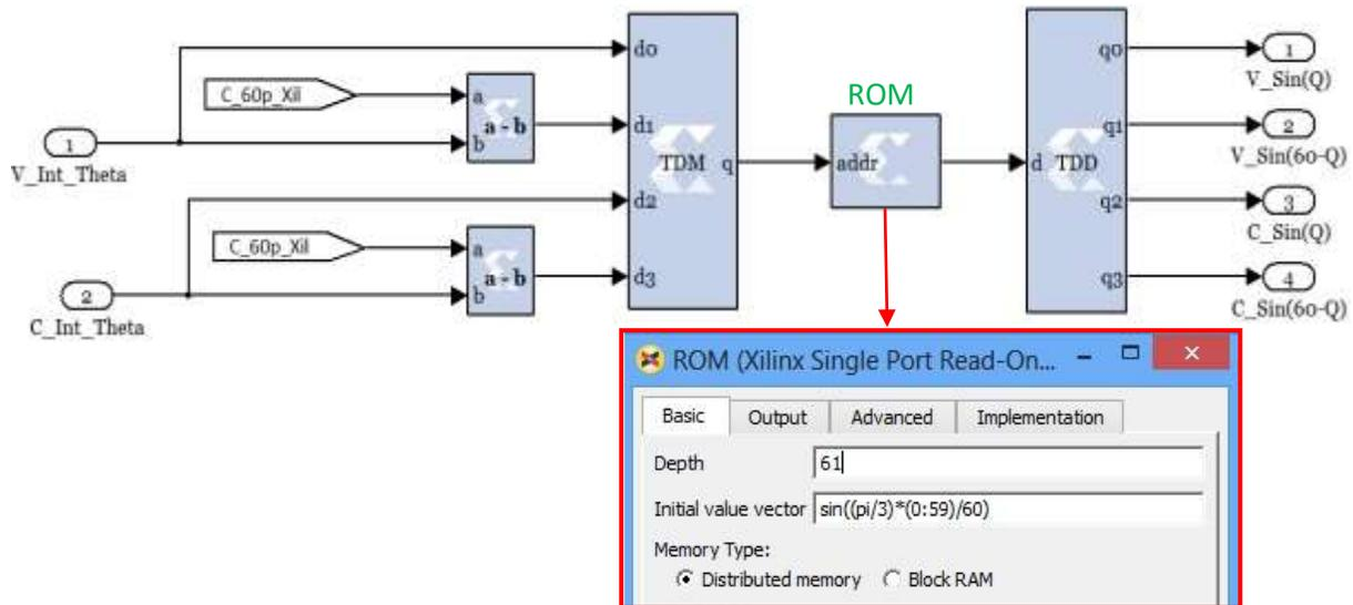
Figure 5.24 Calculation of duty cycles of the VSV and the CSV
