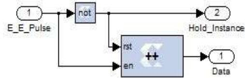
Figure 8.6 Matlab/Xilinx model to capture the Edge Pulse
