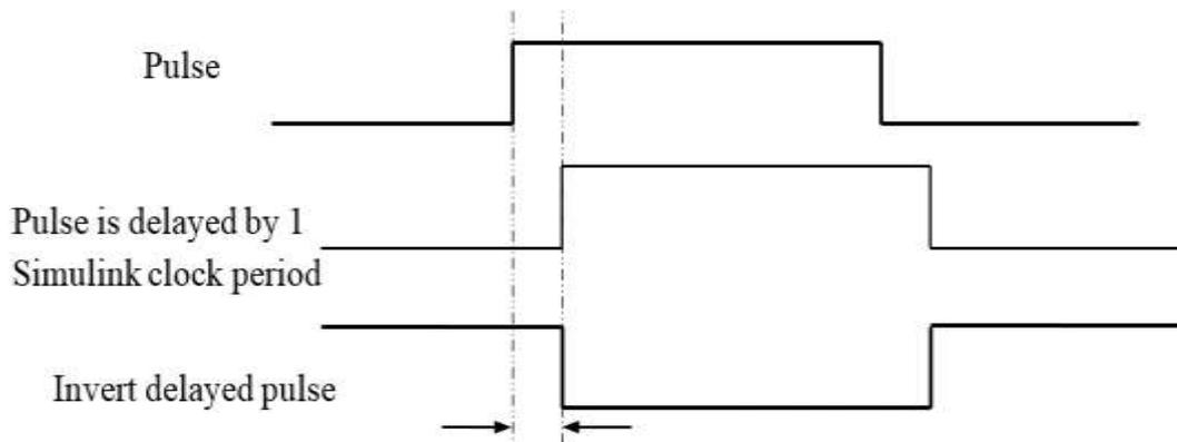
Figure 9.2 Raising edge detection logic
