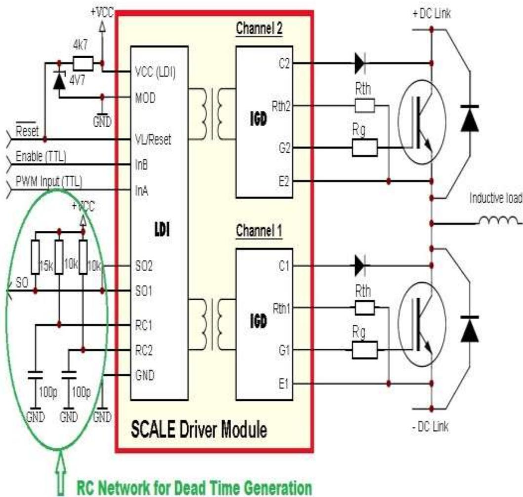
Figure 10.9 Pins RC1 and RC2 in the half bridge mode
