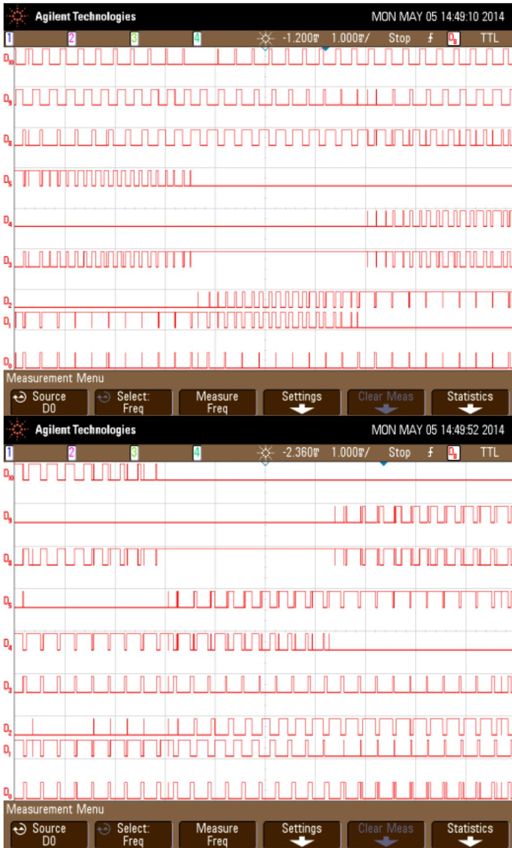
Figure 10.23 Eighteen switching pulses for the matrix converter generated from the FPGA
