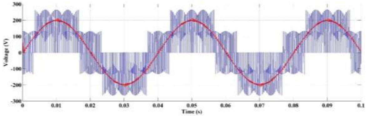
Figure 2.37 Instantaneous and Average Output phase voltage waveform
