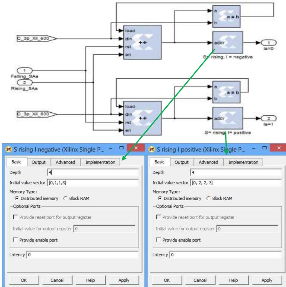
Figure 5.45 Commutation sequence generator when a rising edge is detected
