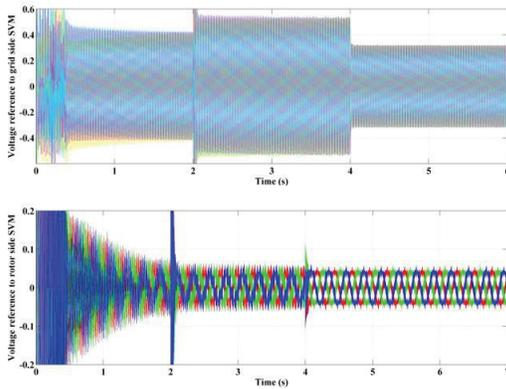
Fig. 11 Reference voltage to grid and rotor side Converters
