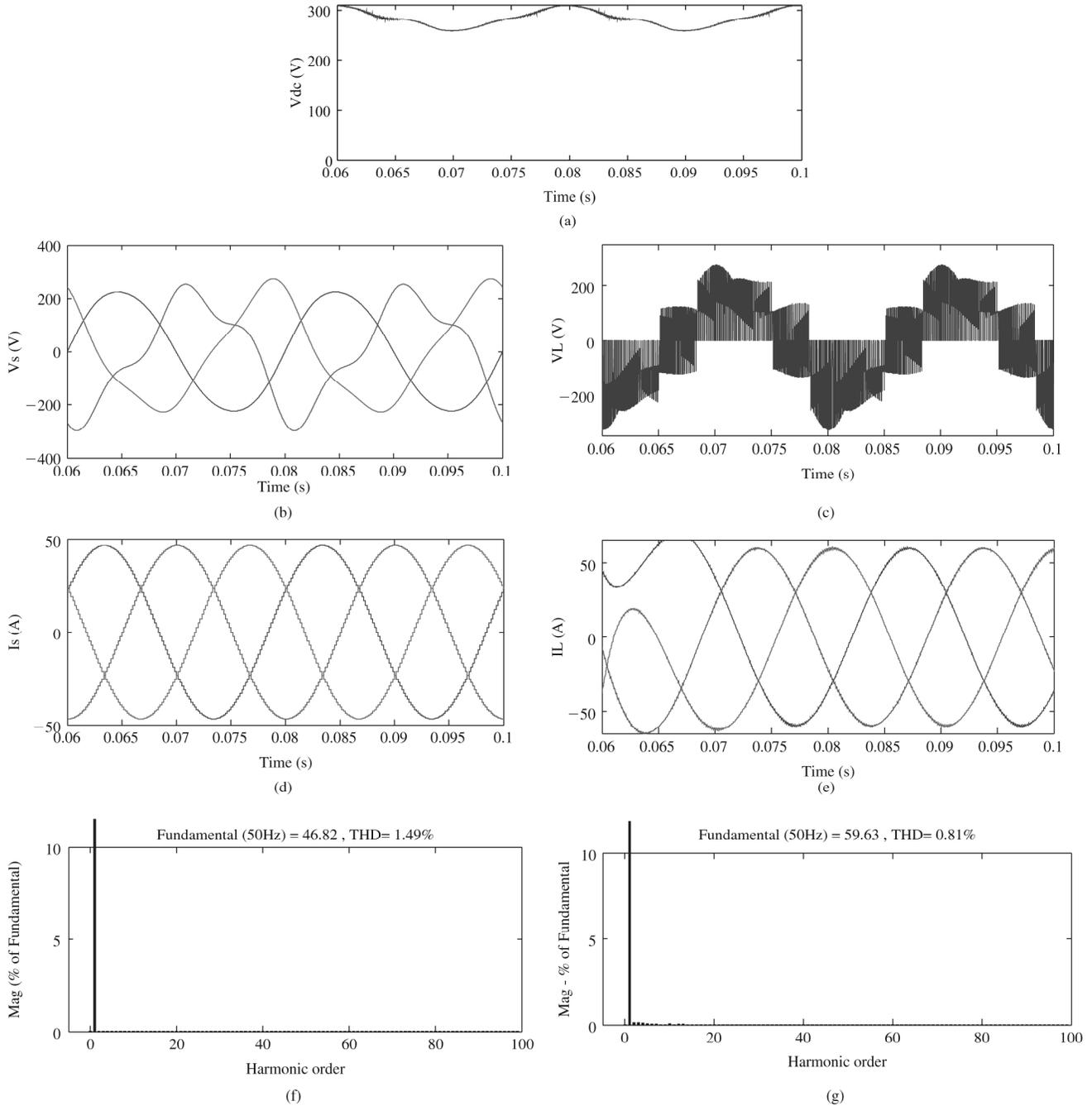
Figure 7. (a) FDC bus voltage, (b) input phase voltage, (c) output phase voltage, (e) input phase current, (e) output phase current, (f) harmonic characteristics of input current, and (g) harmonic characteristics of output current.
