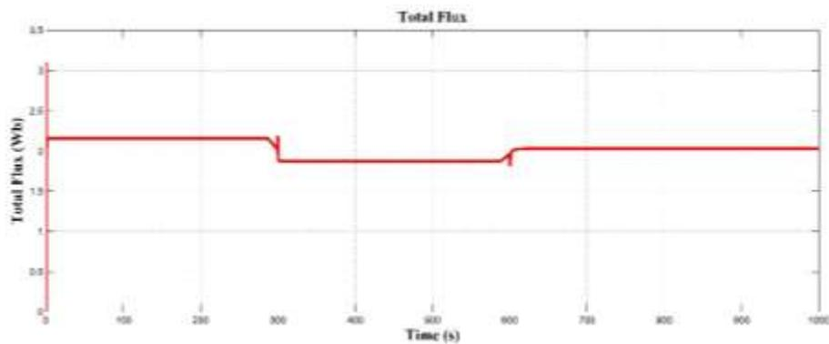
Figure 3.14 Total flux in d-q coordinates
