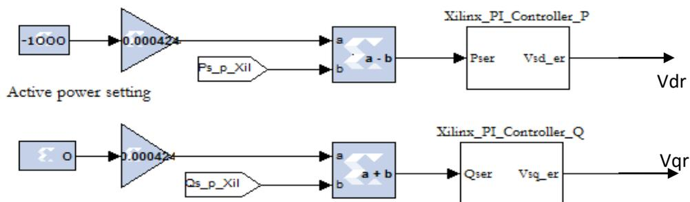
Figure 6.3 Matlab/Xilinx model of the active and reactive powers controller
