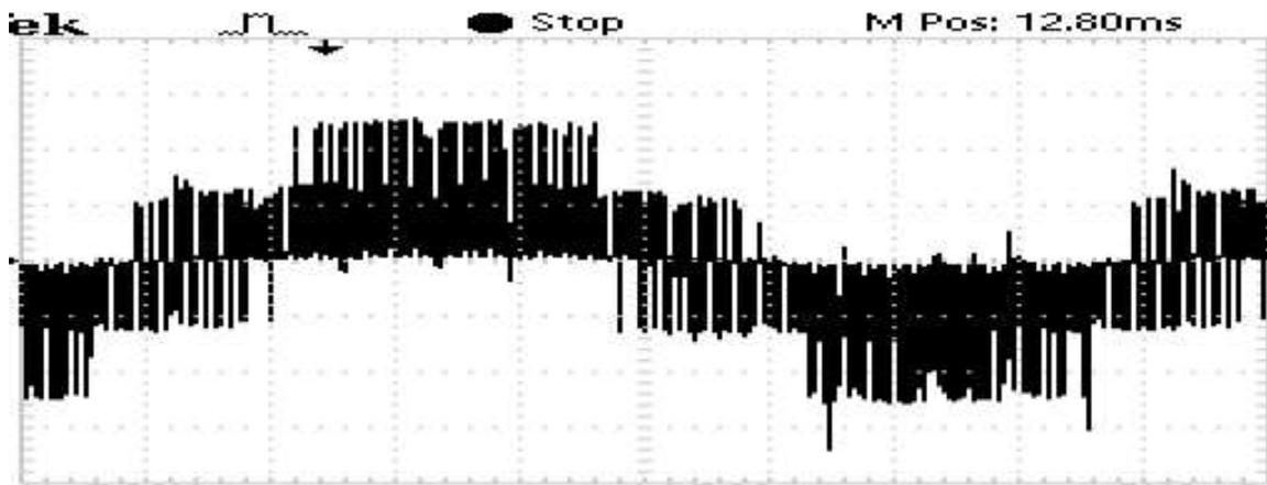
Figure 10.30 (b) Output phase voltage of matrix converter with RL load – Enlarged
