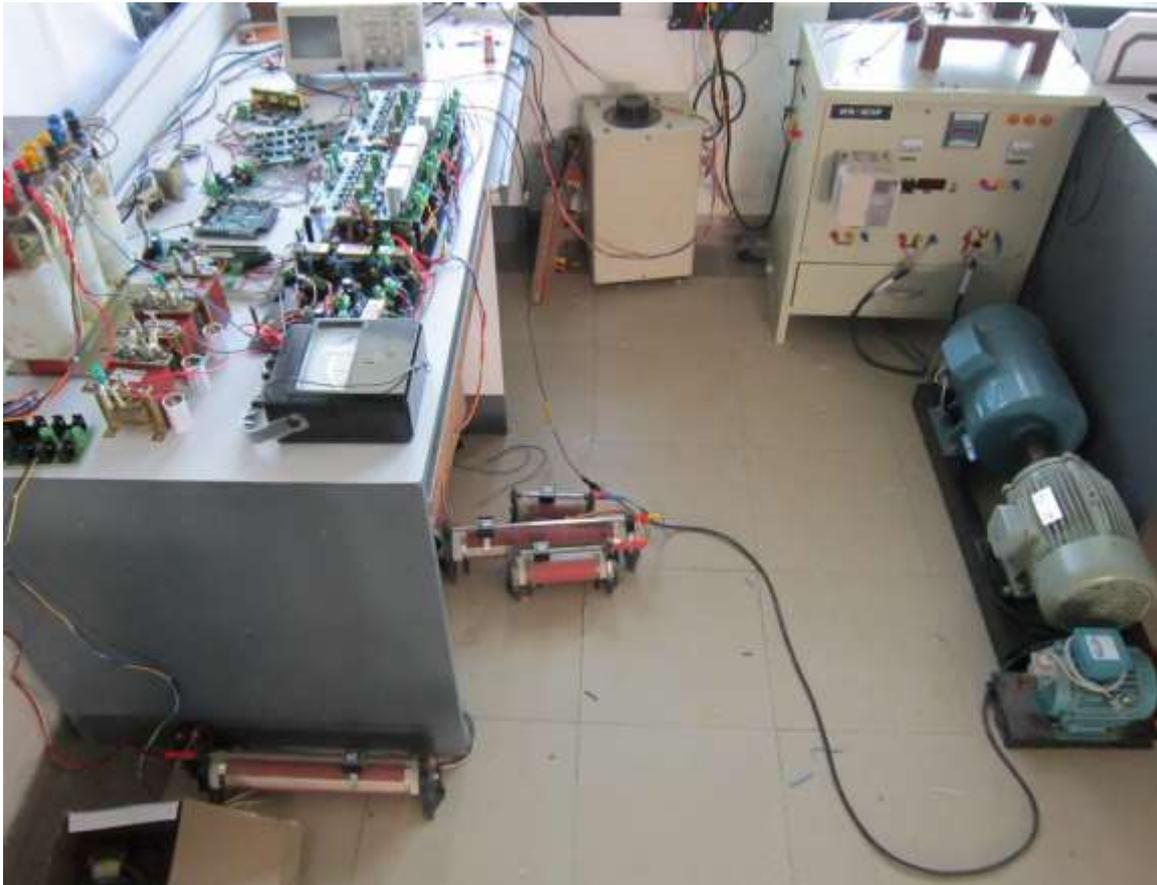
Figure 10.29 Complete prototype including Matrix converter and DFIG
