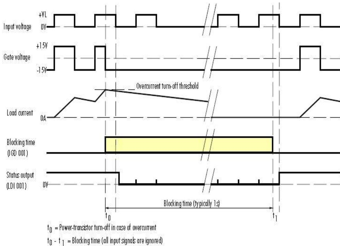
Figure 10.11 Short-circuit and over-current protection/ function of the blocking time
