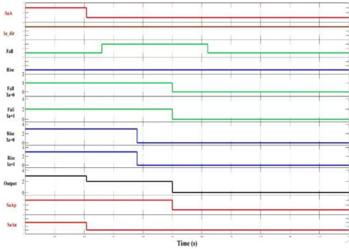
Figure 5.48 Pulses of switch SaA for a falling edge with positive current direction
