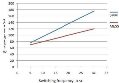
Fig. 9. Total losses in CMC with SVM and MESS techniques
