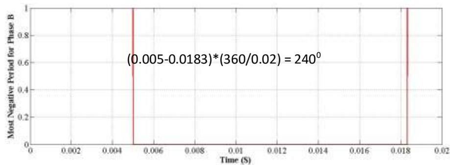
Figure 8.4 The most negative instant of the Y Phase
