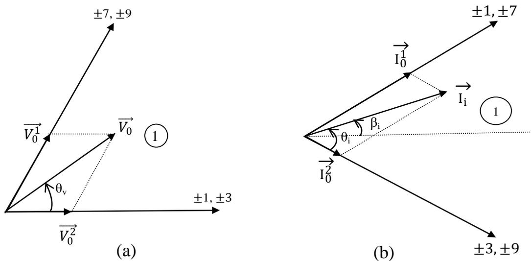
From two switching states with the same number, only one should be used since the corresponding voltage or current SSVs are in opposite directions. The sign of the switch state to be selected can be found using the formula of the duty cycle ratios. If the duty cycle is positive, the switching state with a positive sign is selected, otherwise, the one with the negative sign is selected.
