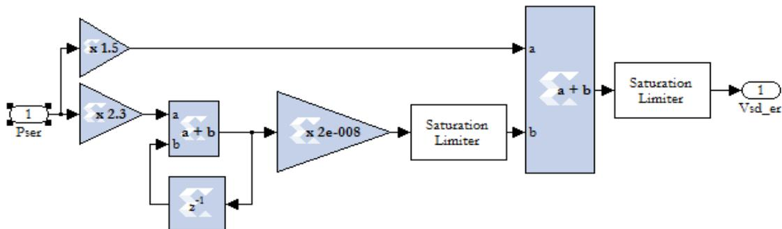
Figure 6.1 Matlab/Xilinx model for the PI controller implementation
