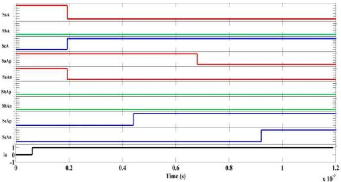
Figure 5.51 Final pulses to switches connected to load phase ‘A’ when current is positive
