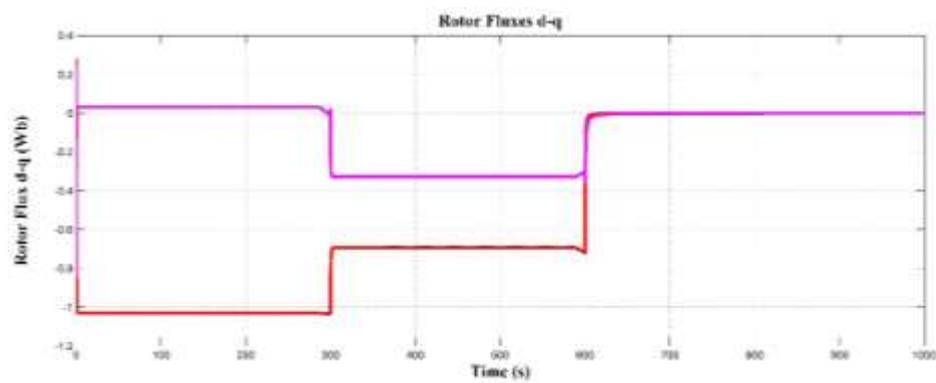
Figure 3.13 Rotor flux in d-q coordinates
