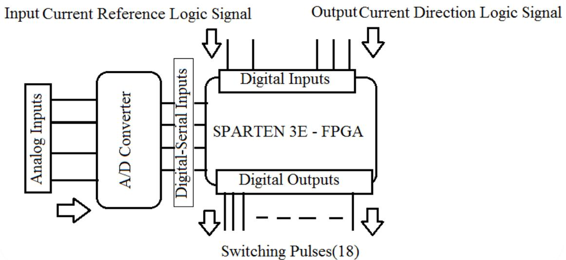
Figure 10.21 Block diagram of the input and output signals to FPGA
