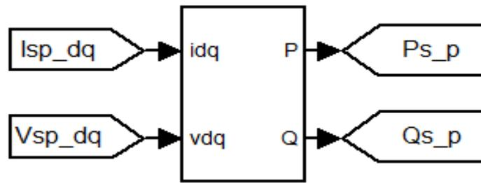
Figure 4.3 Calculation of actual real and reactive powers
