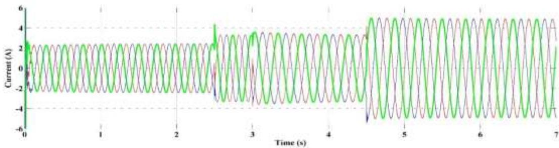
Figure 4.9 (a) Rotor currents  $I_{rabc}$  (matrix converter output currents) versus time
