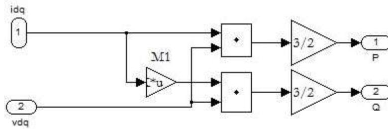
Figure 3.15 Matlab/Simulink model for calculating the stator power
