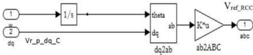
Figure 4.5 Matlab/Simulink model for converting dq to abc values
