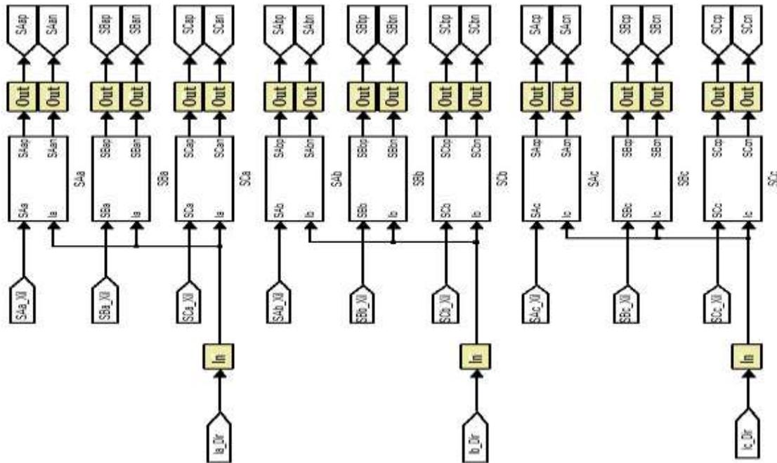
Figure 5.50 Four-step commutation for the nine bi-directional switches
