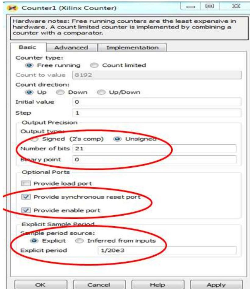
Figure 9.7 Counter settings to obtain the count between edges
