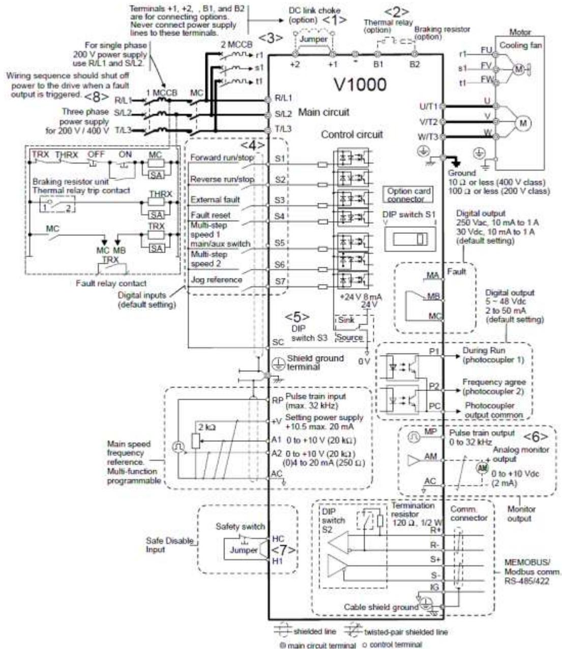
Figure 10.3(b) Connection diagram of the YASKAWA VFD drive
