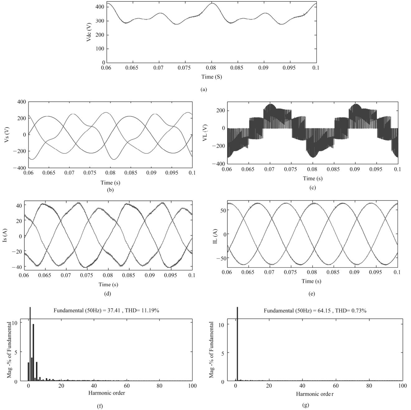
Figure 6. (a) FDC bus voltage, (b) input phase voltage, (c) output phase voltage, (d) input phase current, (e) output phase current, (f) harmonic characteristics of input current, and (g) harmonic characteristics of output current.
