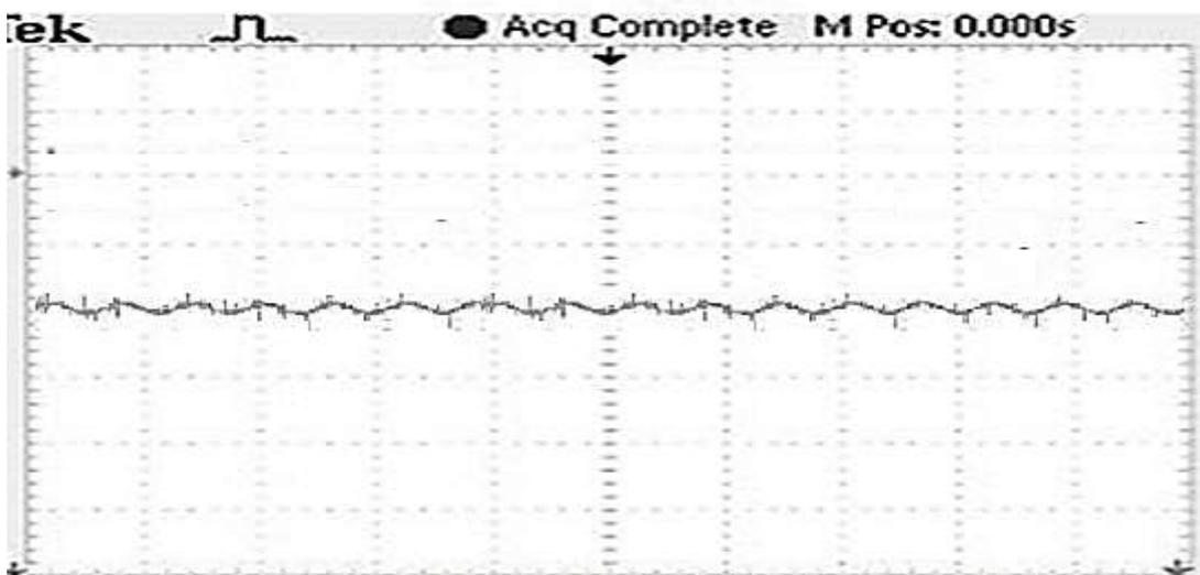
Figure 10.37 (b) Reactive power delivered in the Sub Synchronous mode of operation\
