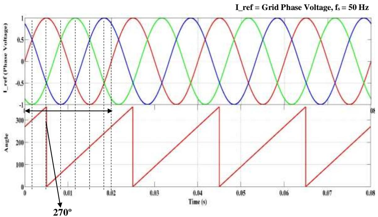
Figure 2.15 Angle of Current Reference with respect to “ $\alpha$ ” axis,  $\beta_i$
