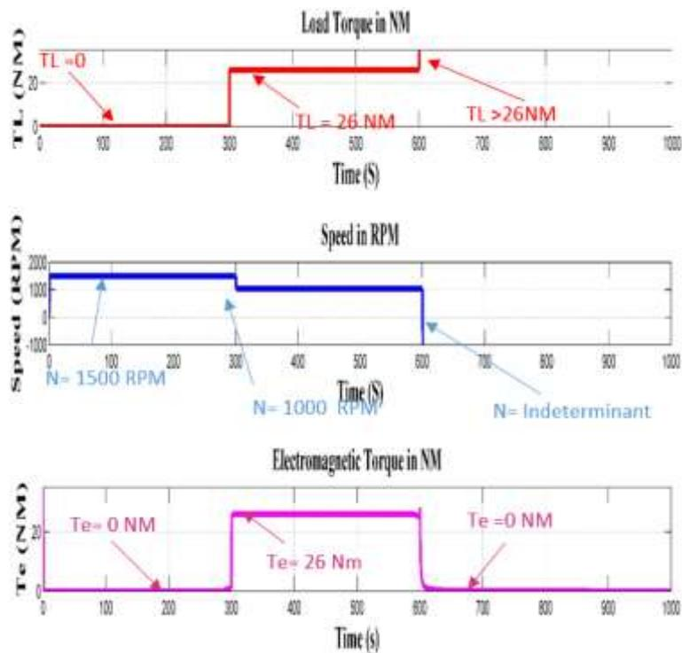
Figure 3.9 Results for load, torque, speed and electromagnetic torque obtained from the scope
