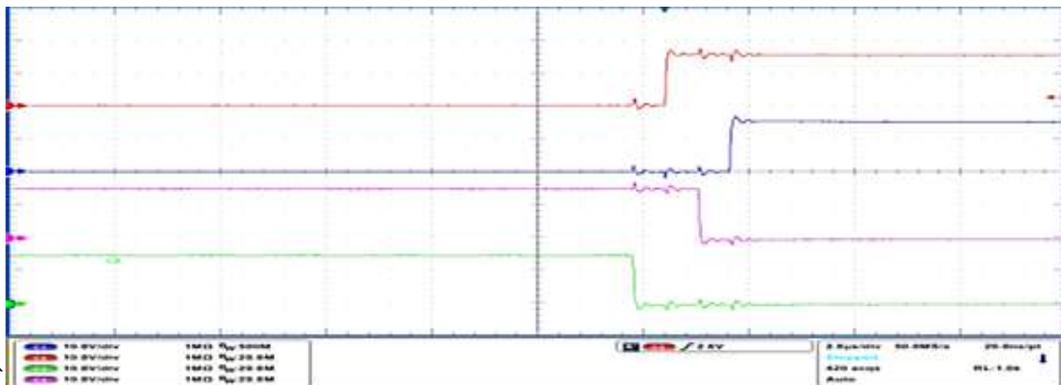
Figure 10.18 Commutation sequence when the current direction is positive
