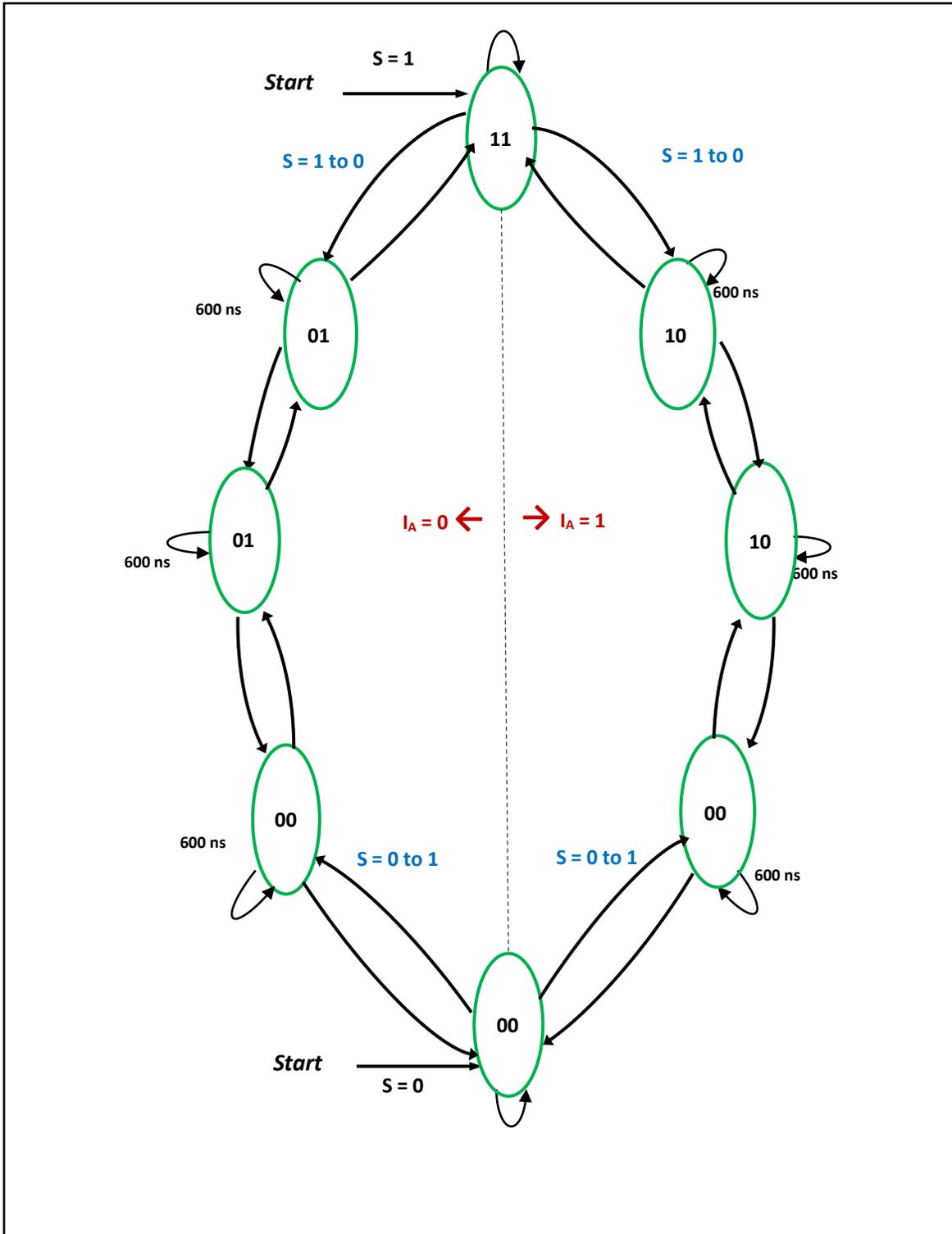
Figure 5.36 Four-step commutation state diagram
