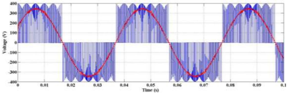
Figure 2.39 Instantaneous and average waveforms of the output line-to-line voltage
