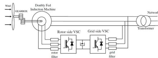
Fig. 1. DFIG-based variable wind-speed turbine
