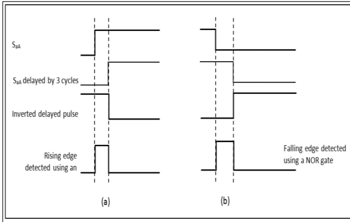
Figure 5.39 rising and falling edge detection
