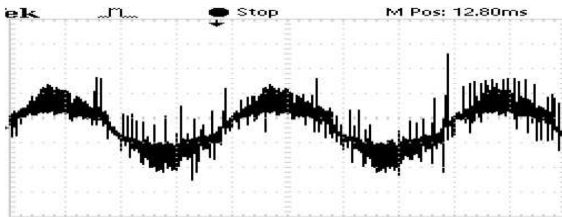
Figure 10.31 Input current of matrix converter with RL Load
