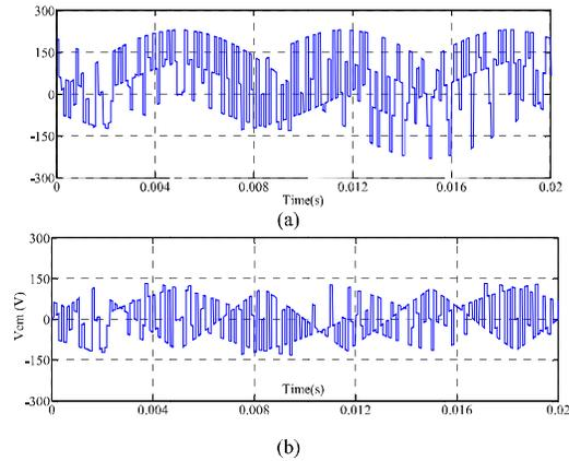
Figs. 7. Simulation Results (a) Without common mode voltage reduction and (b) With common mode voltage reduction
