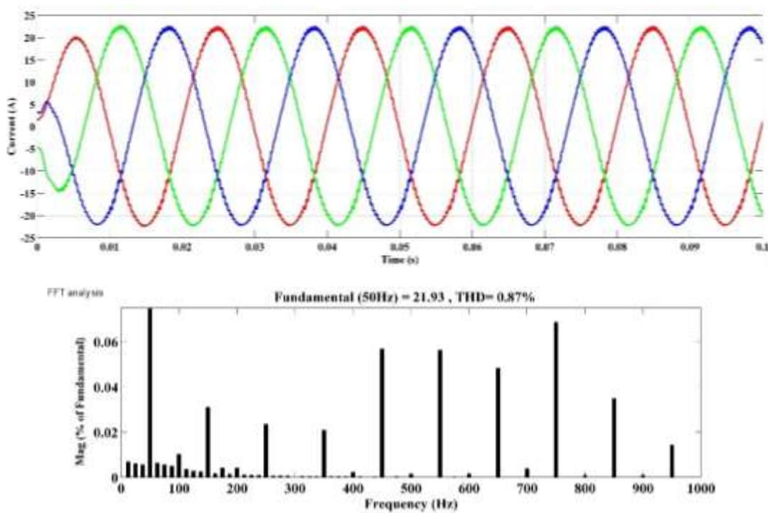
Figure 2.43 Input current when the filter is included, and its harmonic spectrum
