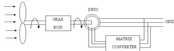
Fig. 2. Matrix converter based variable speed WECS
