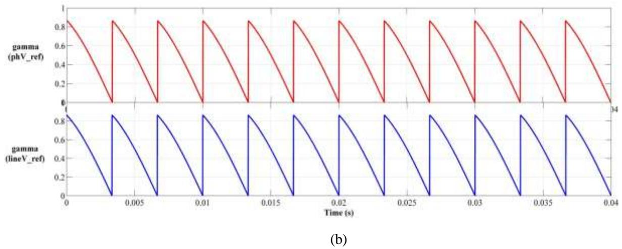
Figure 5.12 Computation of (a)  $d_s$  (b)  $d_\gamma$  using the conventional and proposed CSV methods
