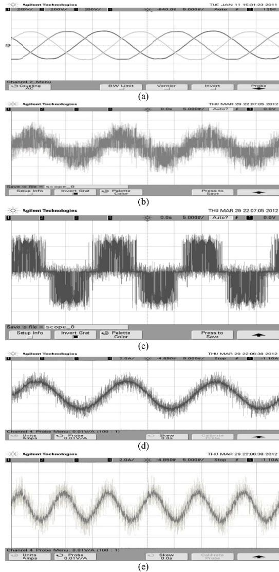
Figs. 12. Simulation Results (a) input phase voltage (b) output phase voltage, (c) output line voltage, (d) output current, (e) input current
