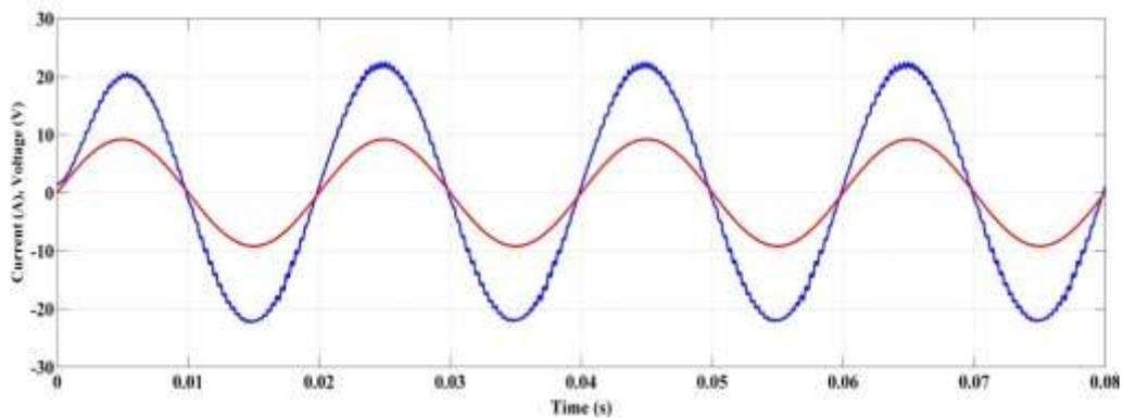
Figure 2.44 Phase relationship between the input current and phase voltage
