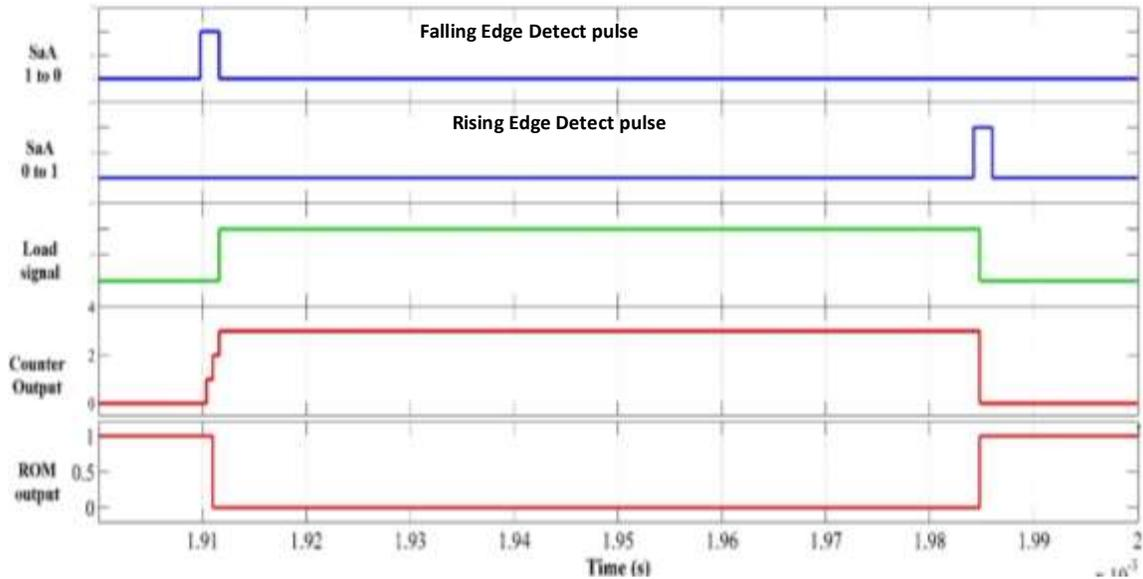
Figure 5.43 Counter output for the negative current when a falling edge is detected
