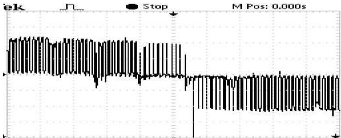
Figure 10.33 (b) Output Line Voltage of matrix converter applied to the rotor of the DFIG –
