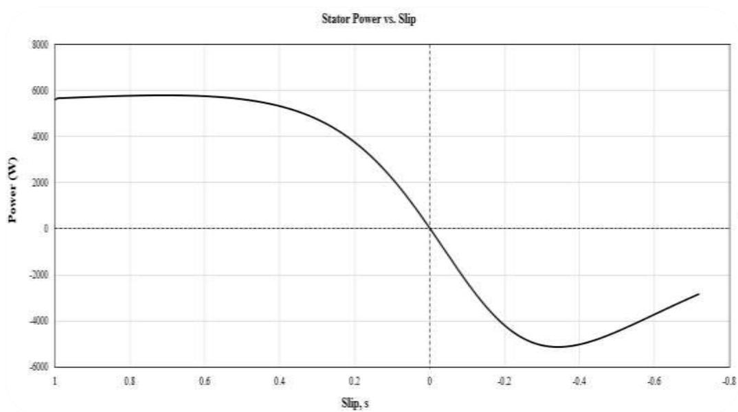
Figure 10.2(a) Power-slip characteristics of the induction generator used
