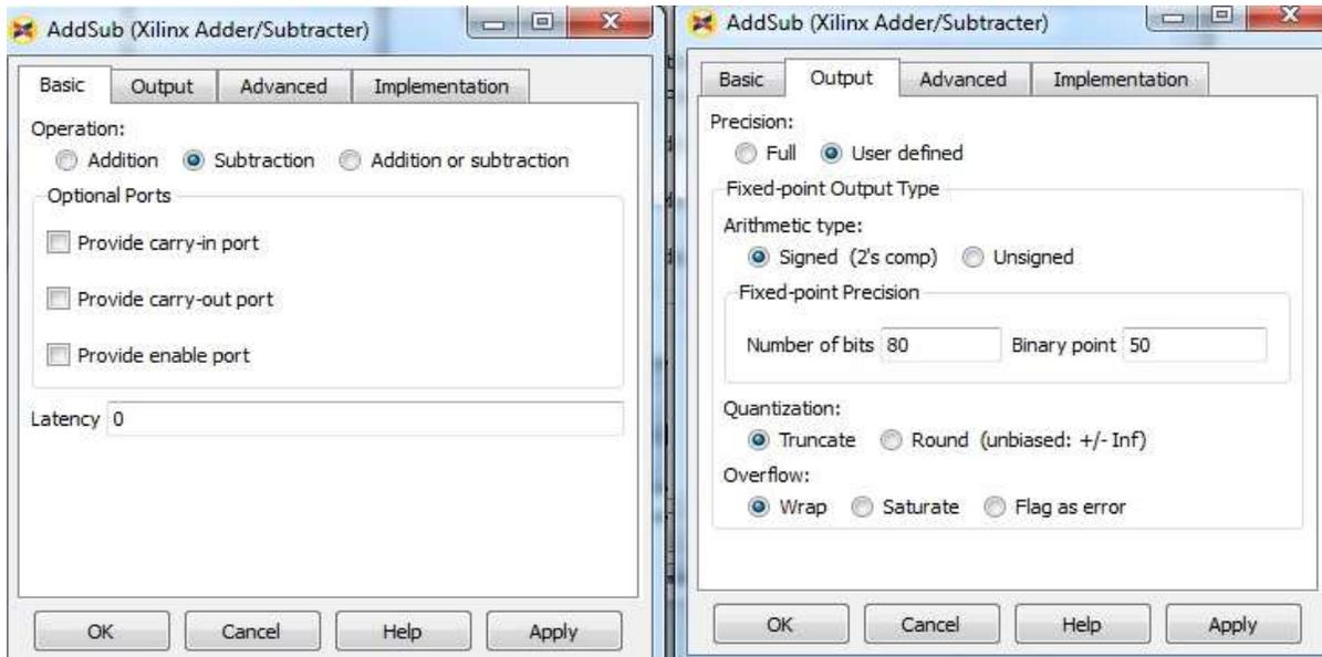
Figure 9.12 Setting for the Add-Sub block
