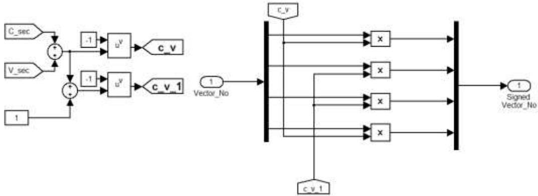
Figure 2.27 Sign Assignment for Vectors
