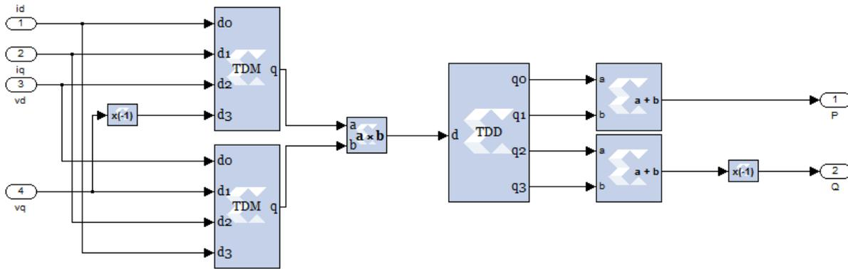
Figure 6.9 Use of TDM and TDD blocks to calculate the stator active and reactive powers
