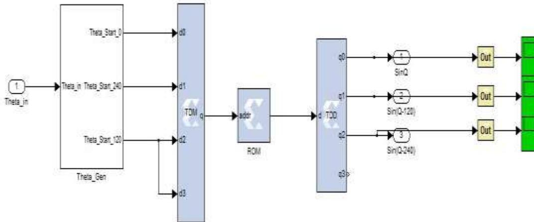
Figure 8.23 Matlab/Xilinx model for generating the sine wave using ROM, TDM and TDD blocks
