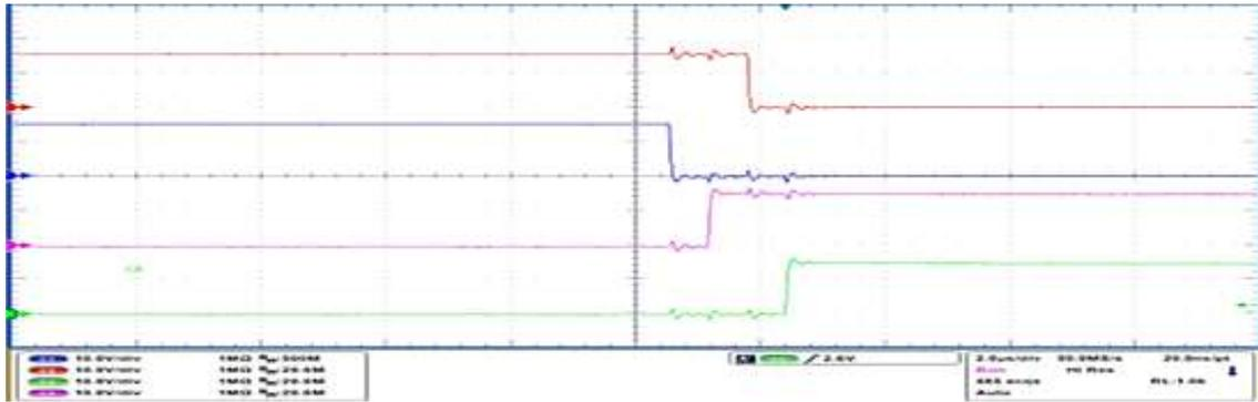
Figure 10.19 Commutation sequence when the current direction is negative
