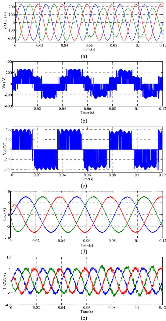
Figs. 10. Simulation Results (a) input phase voltage (b) output phase voltage, (c) output line voltage, (d) output current, (e) input current
