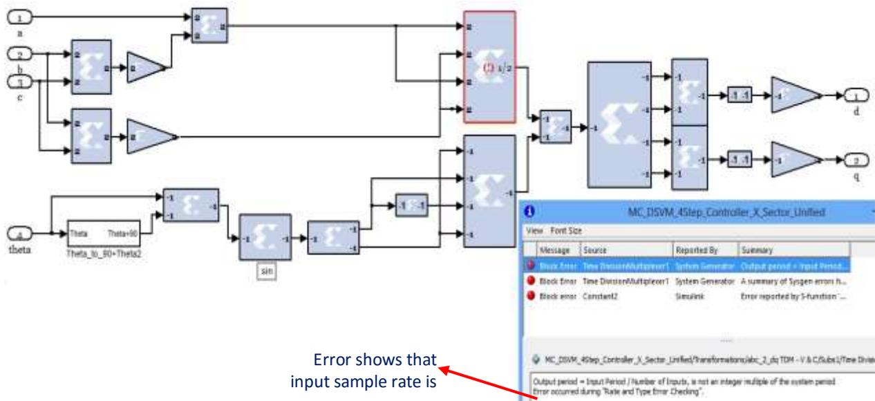
Figure 5.4 Sampling rate error
