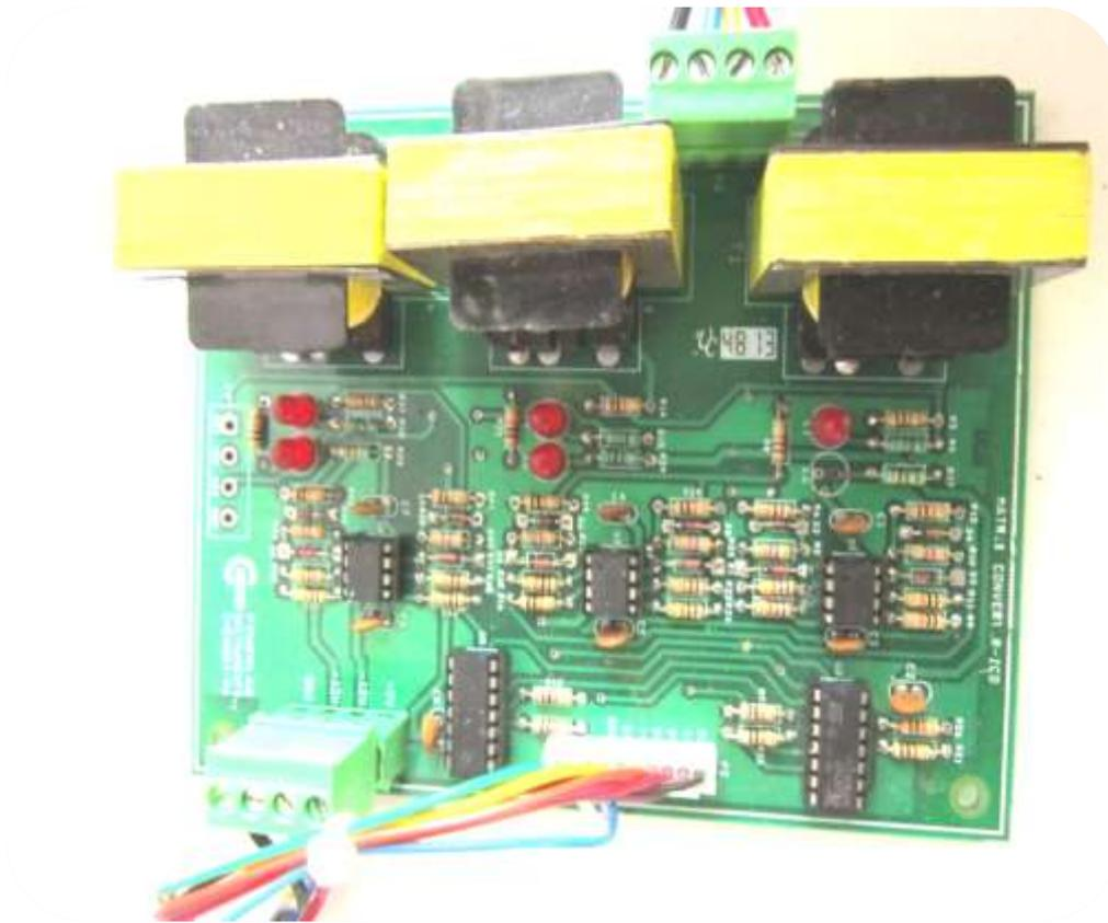
Figure 10.16 Comparator circuit for the generation of the current reference internally
