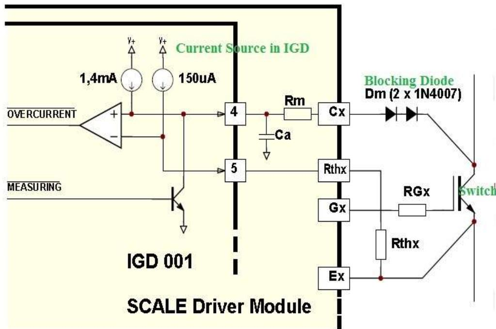
Figure 10.10 Collector sense circuit
