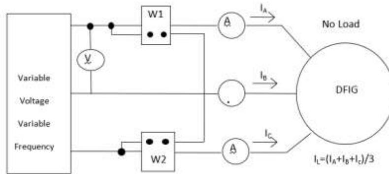
Figure 3.3 Circuit diagram for the no-load test
