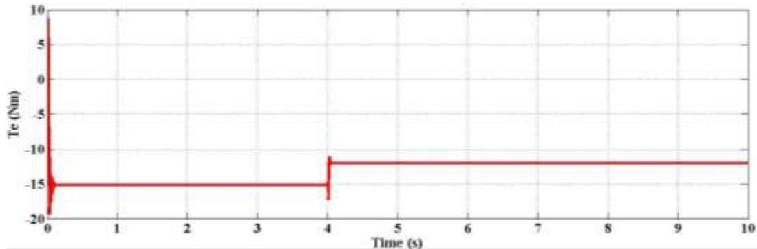
Figure 3.27 Electromagnetic torque for machine operation as Generator
