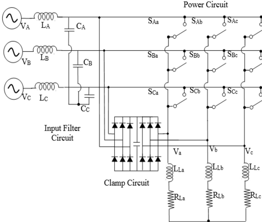
Figure 1.6 Structure of the conventional matrix converter
