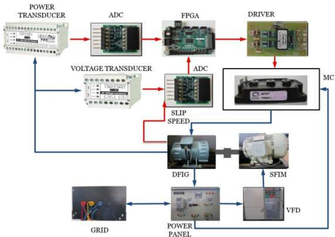
Figure 10.27 Block Diagram Representation of Interconnection of various units
