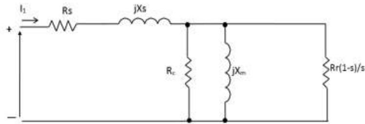
Figure 3.4 (b) Equivalent circuit after neglecting  $R_r$  and  $X_r$
