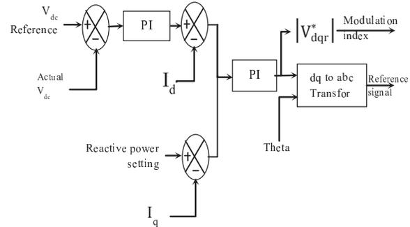
Fig. 4 Grid side converter control
