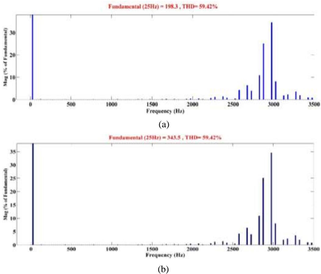
Figure 2.40 Harmonic Spectrum of (a) Output Phase voltage (b) Output line voltage
