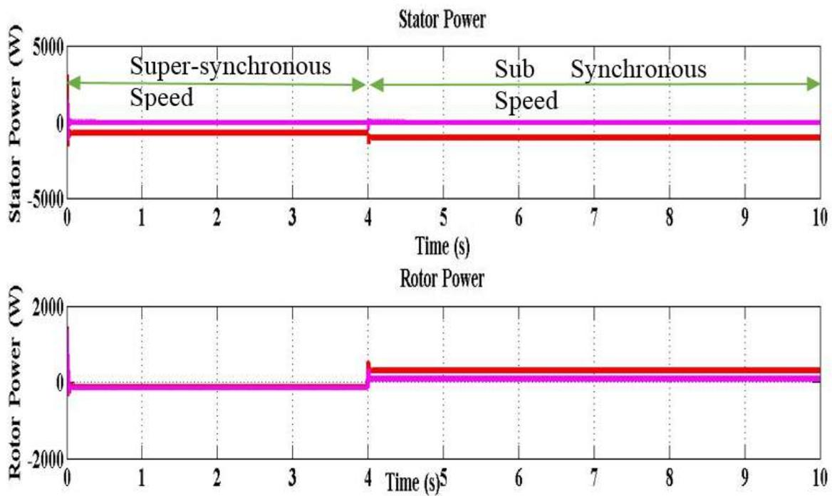
Figure 3.26 Active and reactive powers of the stator and rotor powers
