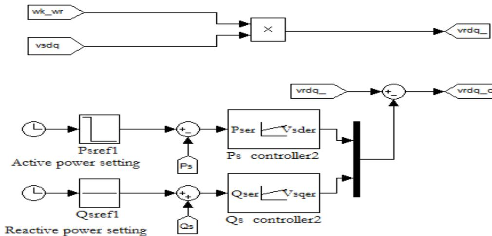
Figure 4.4 Active power and reactive power controllers for the RSC connected to the matrix converter fed DFIG based wind energy conversion system
