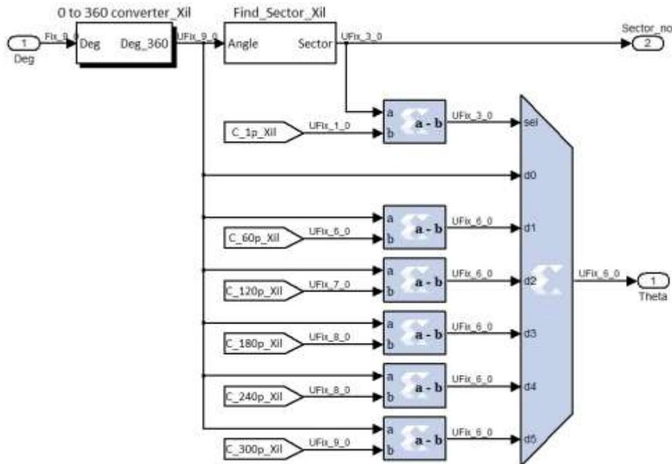
Figure 5.21 Internal angle computation
