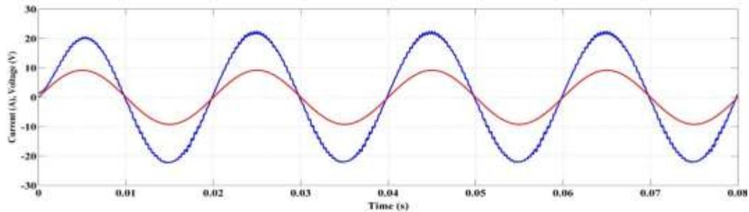
Figure 5.13 Phase relationship between input current and phase voltage
