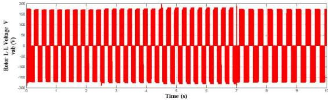
Figure 4.8 Rotor line-to-line voltage,  $V_{ab}$ , versus time
