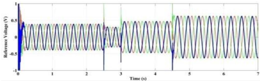
Figure 4.7 Three-phase reference voltages versus time
