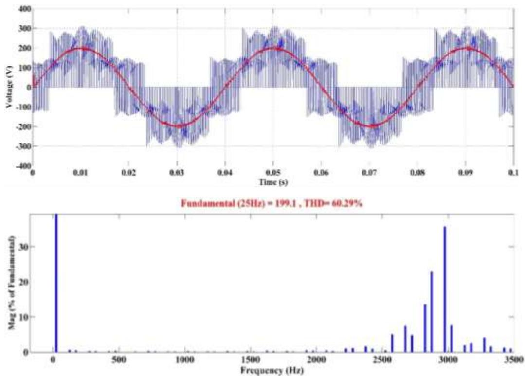
Figure 2.41 Output Phase Voltage and its Harmonic Spectrum with Input filter
