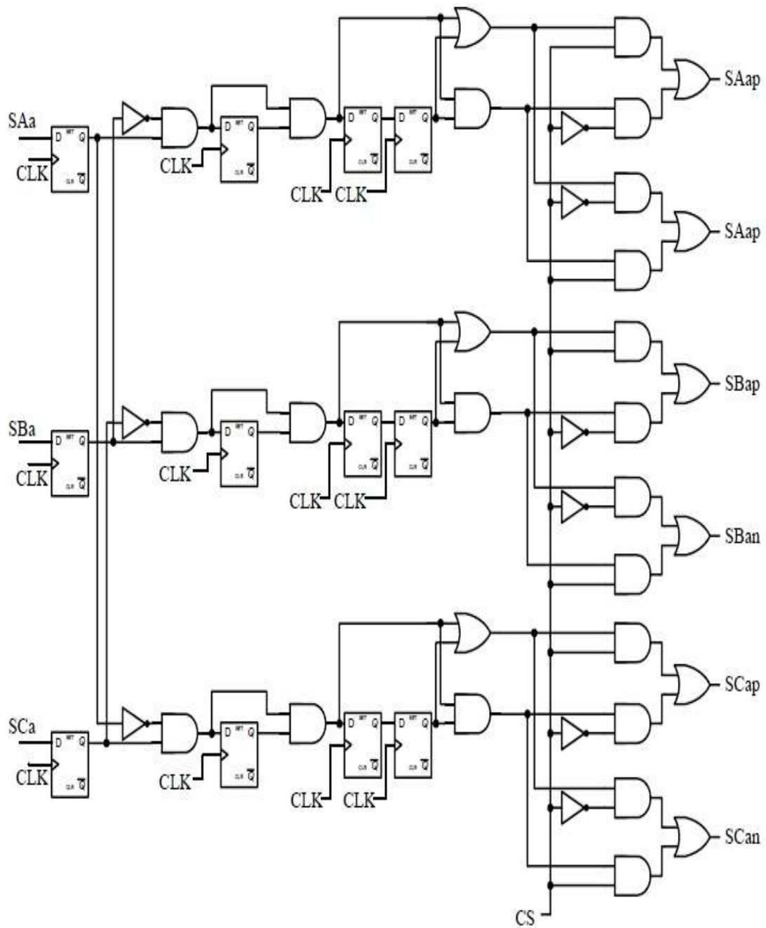
Figure 2.34 Sequential logic circuit that implements four-step commutation for one phase
