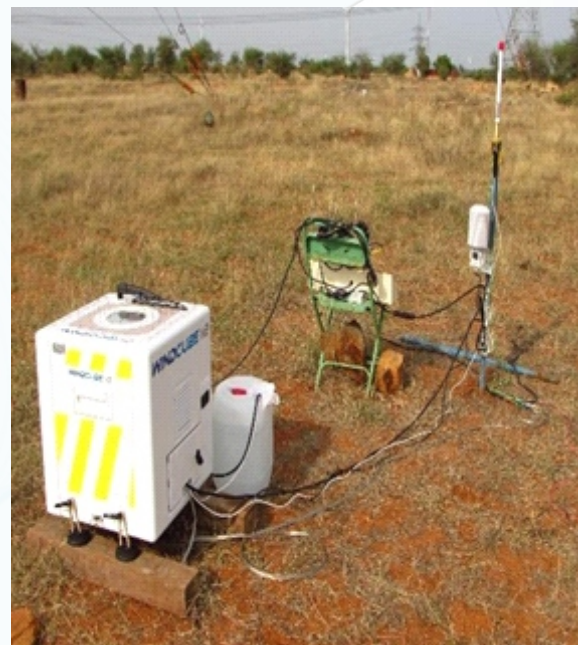
Fig 2. Installation of LIADR (Wind Cube)
